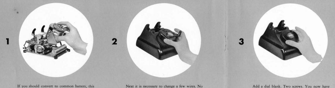
If you should convert to common battery, this Leich magneto telephone can be changed over to common battery operation in about five minutes. This can be done at the subscriber's premises. First—remove the generator as shown. Four screws, three spade connectors. Next it is necessary to change a few wires. No soldering. This changes the circuit to common battery operation. Then remove the generator face plate as shown. Two screws.
