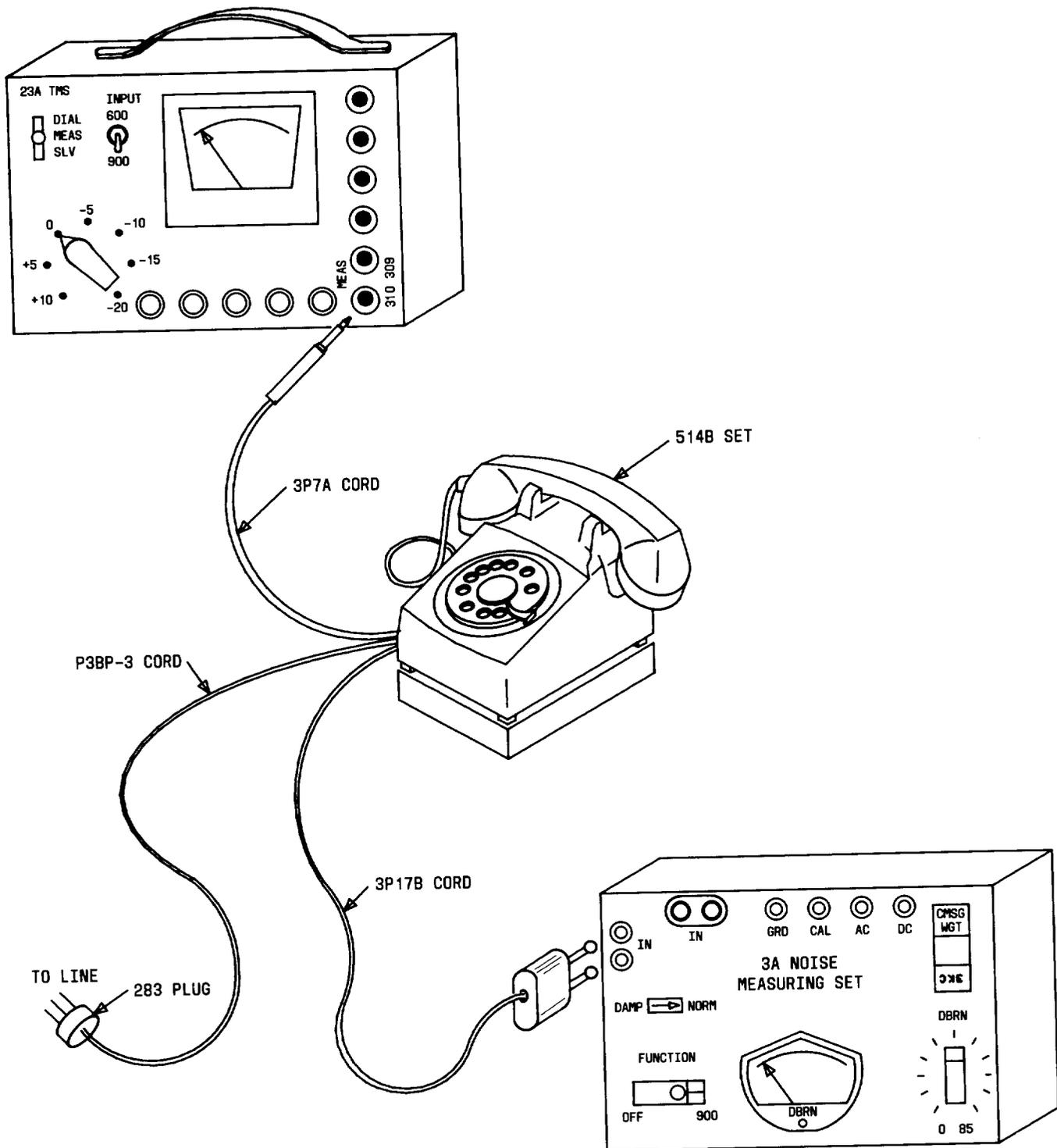
Fig. 8—514B Telephone Set Arrangement
