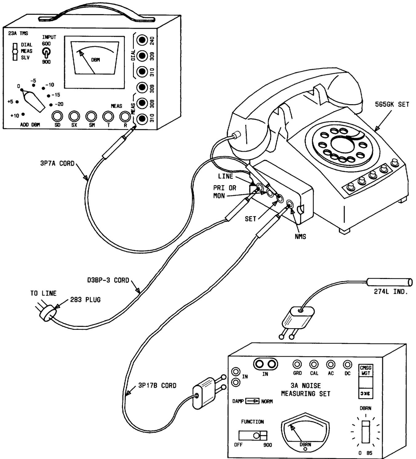
Fig. 9—565GK Telephone Set Arrangement
