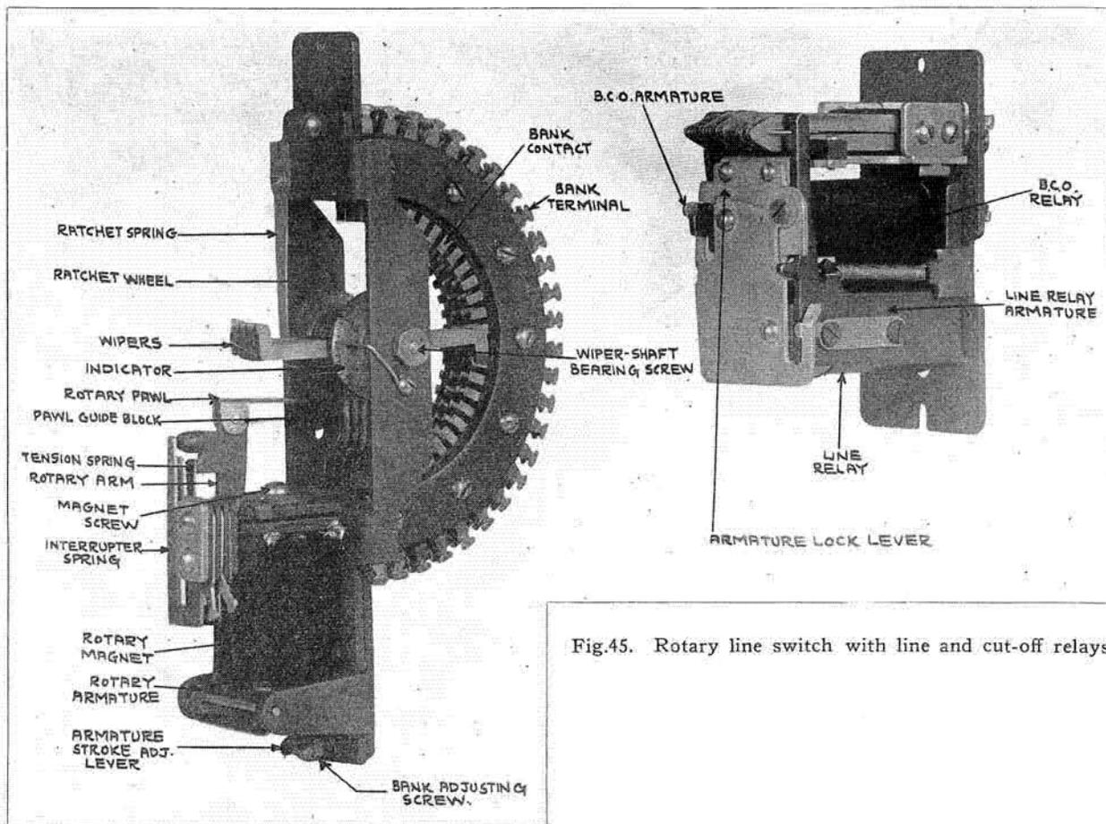
Fig.45. Rotary line switch with line and cut-off relays
