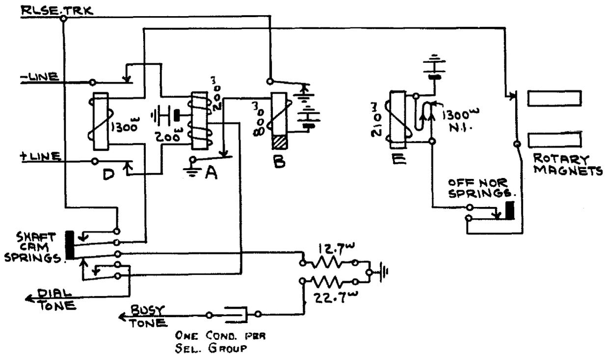
Fig. 32. Selector circuit, showing "all trunks busy" condition
