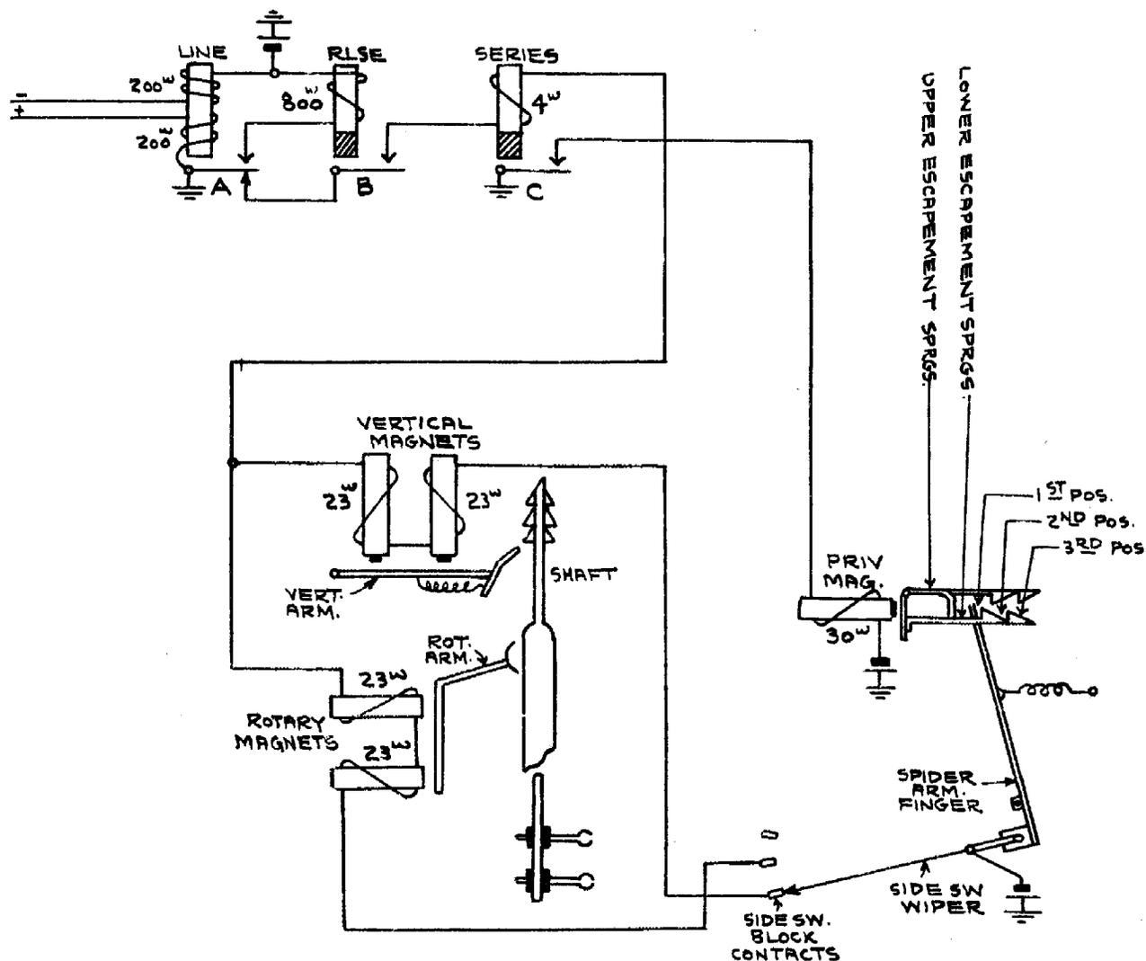
Fig. 95. Test distributor circuit, showing side switch operation
