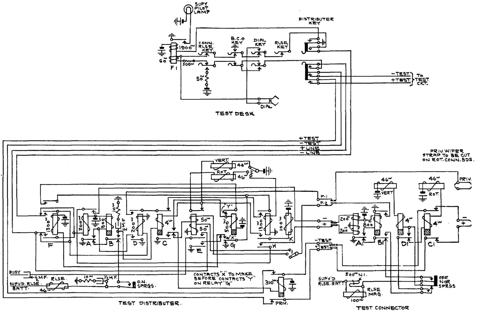
Fig. 97 Wire chief's testing equipment
