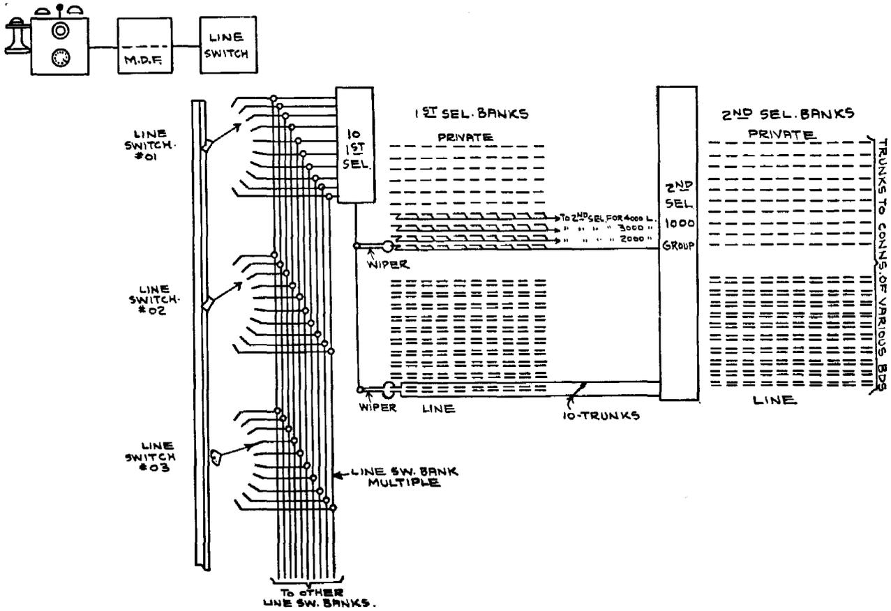
Fig. 40. 10,000 line system showing line switch multiple
