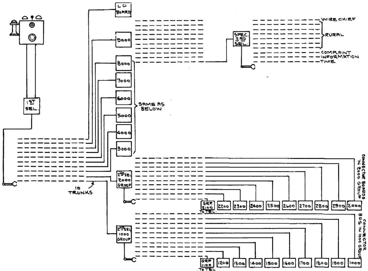
Fig. 25. Trunking scheme for 10,000 line system (4 digit)
