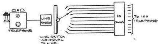
Fig. 36. 100 line system using line switches
