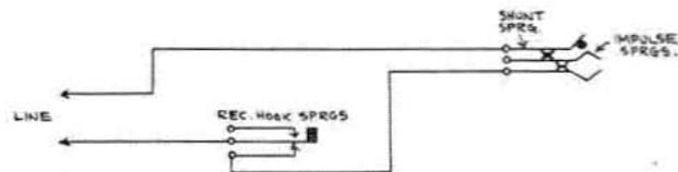
Fig. 5. Impulse circuit of telephone
