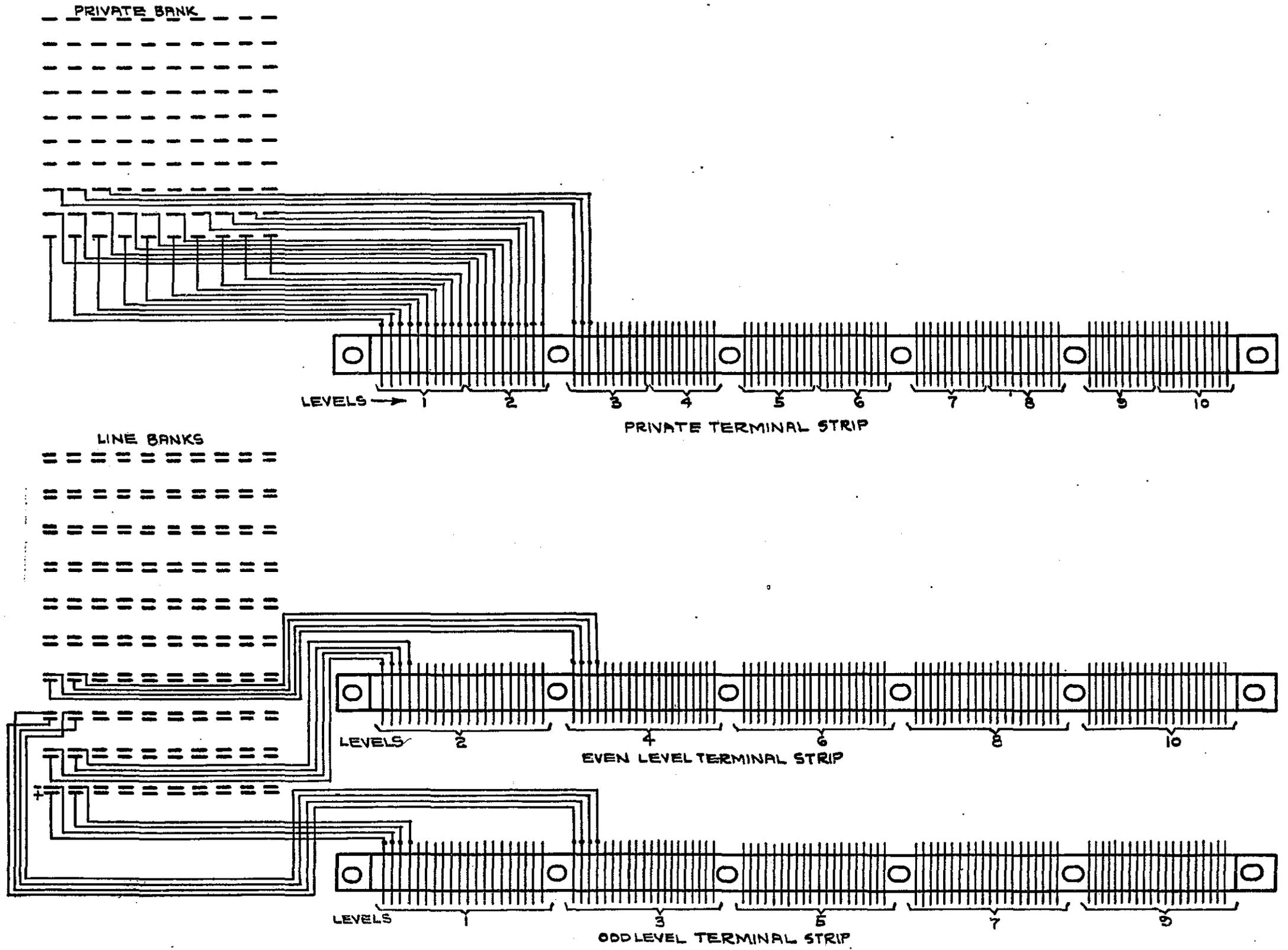
Fig. 69. Wiring of selector banks to terminal strips
