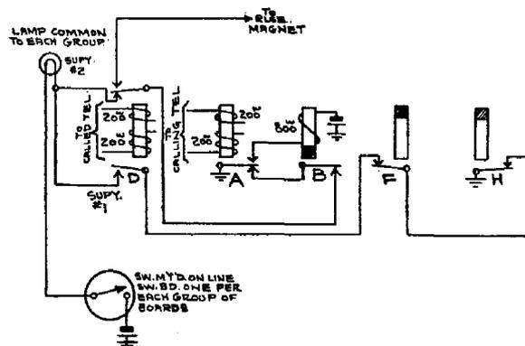
Fig. 18. Disconnect supervisory circuit
