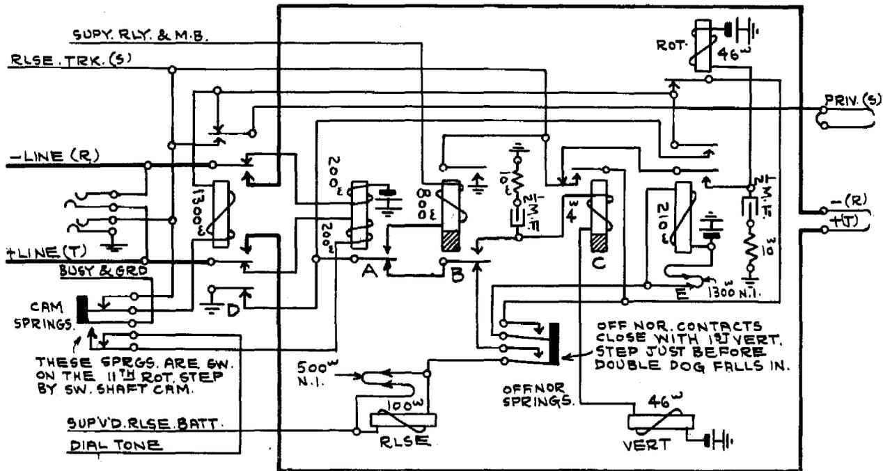
Fig. 33. Complete selector circuit
