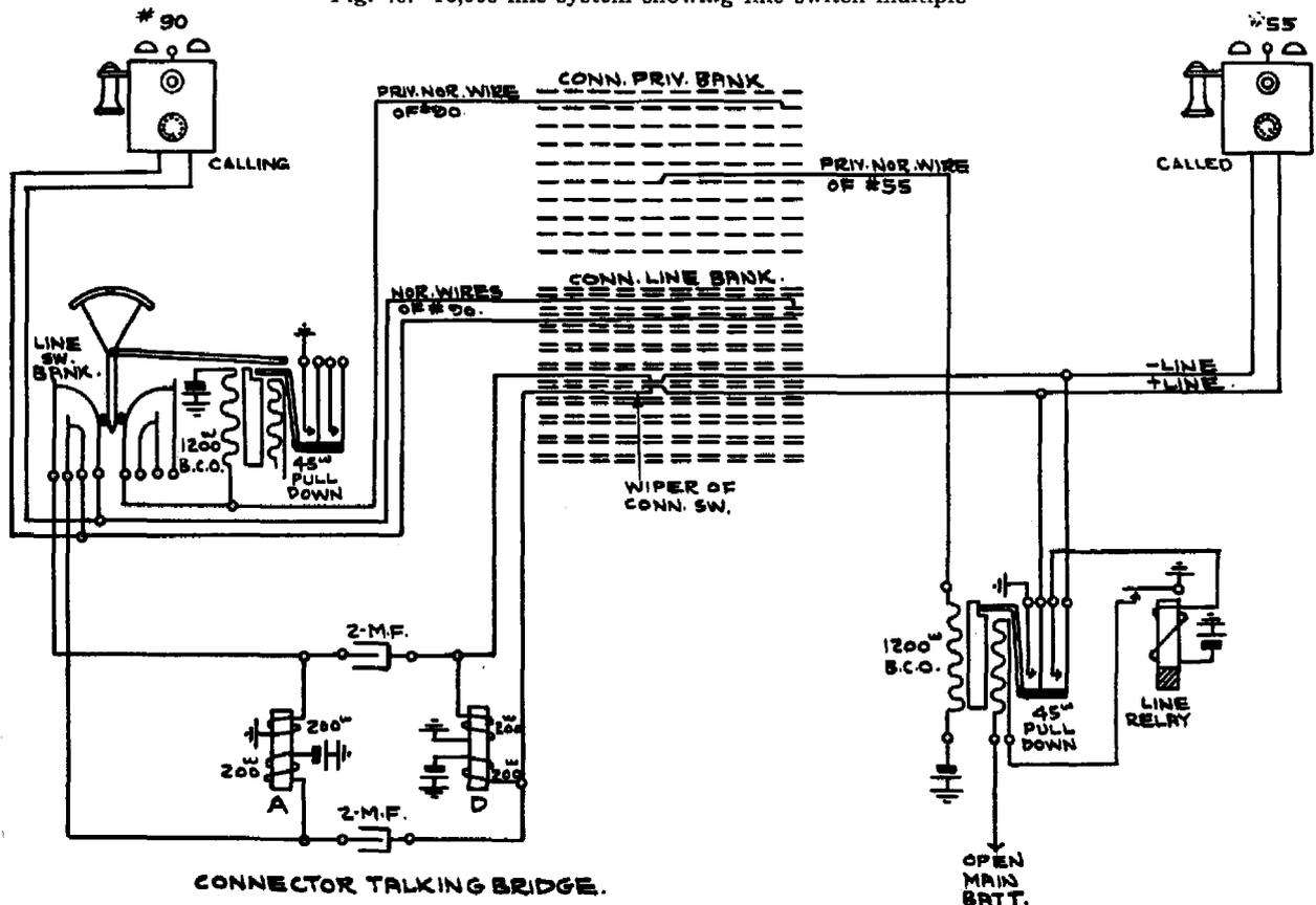
Fig. 41. Transmission circuit of 100 line system
