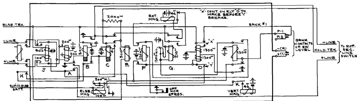
Fig. 88. Switching selector repeater, preparatory to switching
