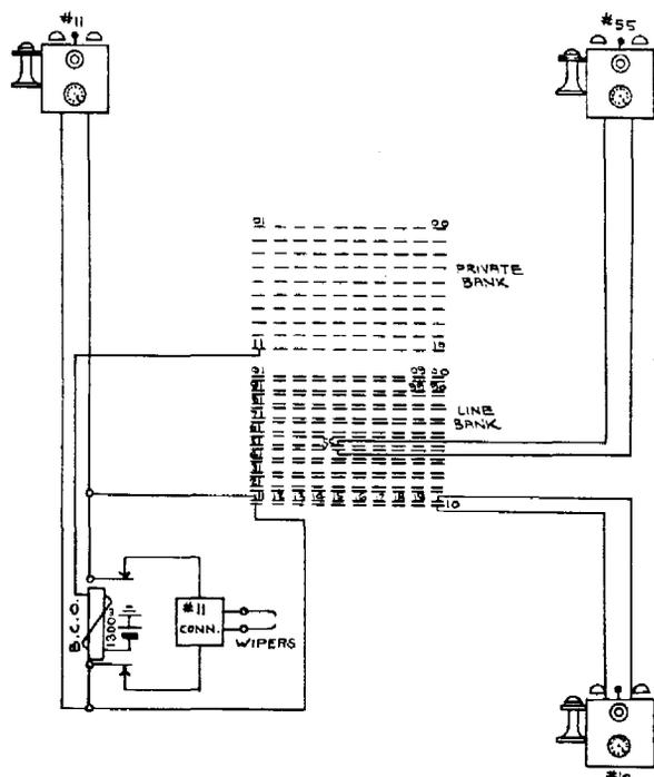
Fig. 9. Showing connections for a simple 100 line system
