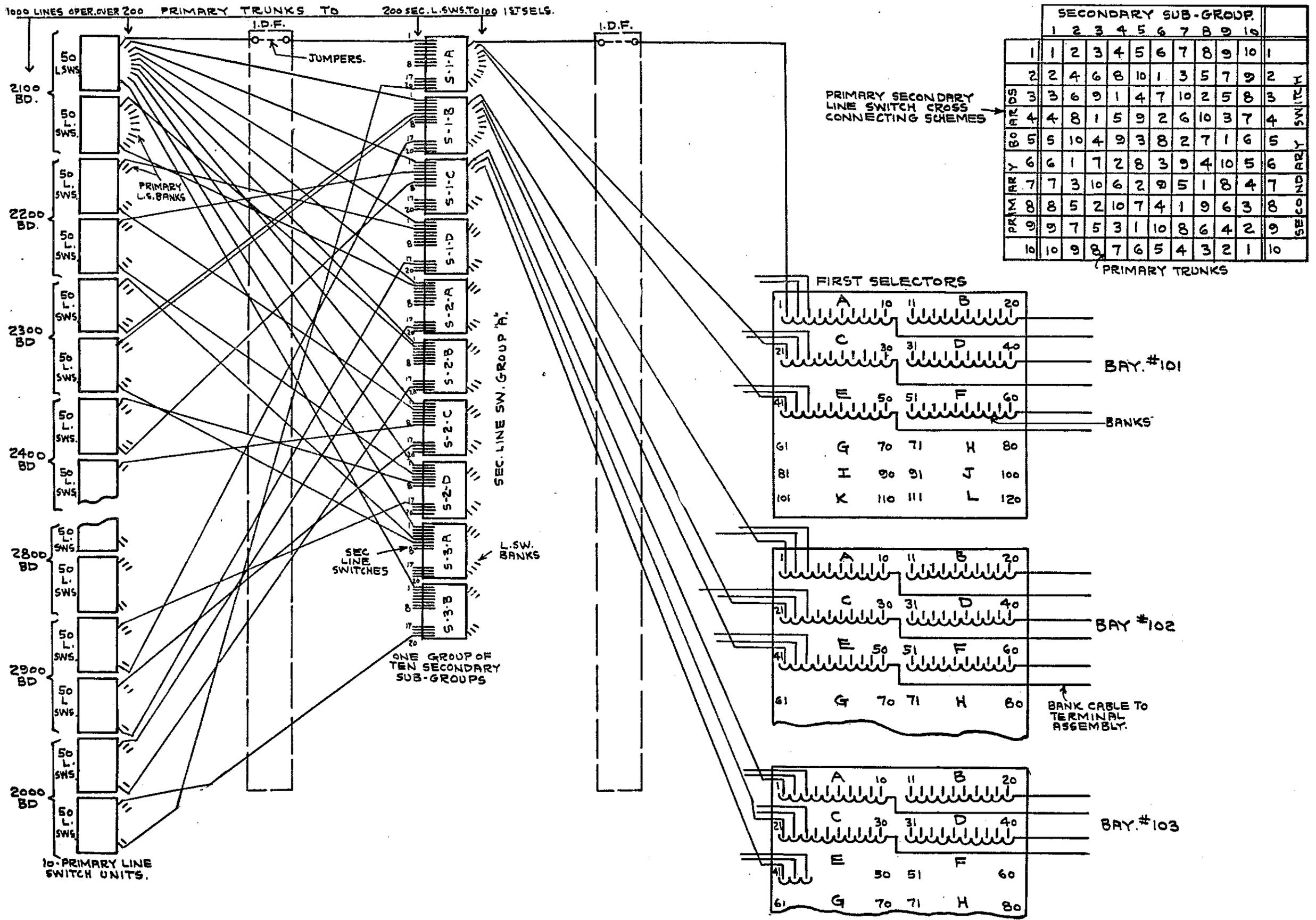
Fig. 65. Trunking plan, primary to secondary line switches
