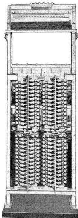
Fig. 35. Group of 100 plunger line switches
