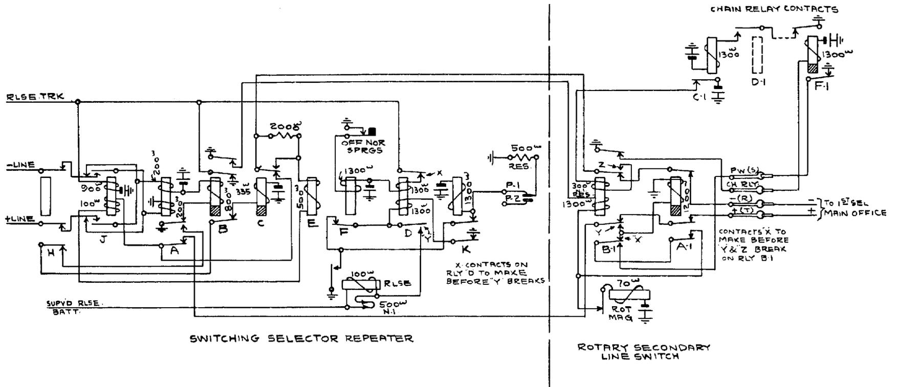
Fig. 86. Switching selector repeater, showing impulse repeating feature
