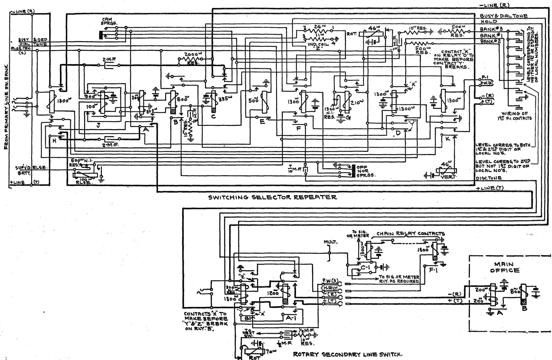
Fig. 90. Switching selector repeater, complete circuit
