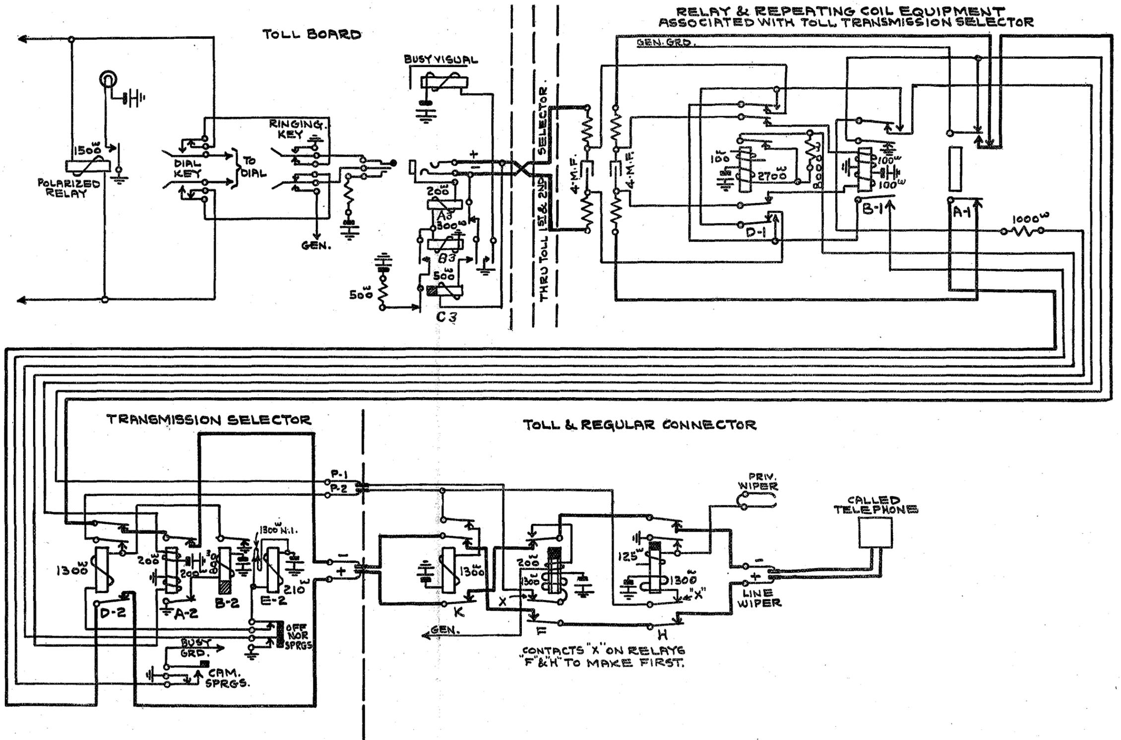
Fig. 83. Toll connection to subscriber's line, talking position, giving supervision to operator
