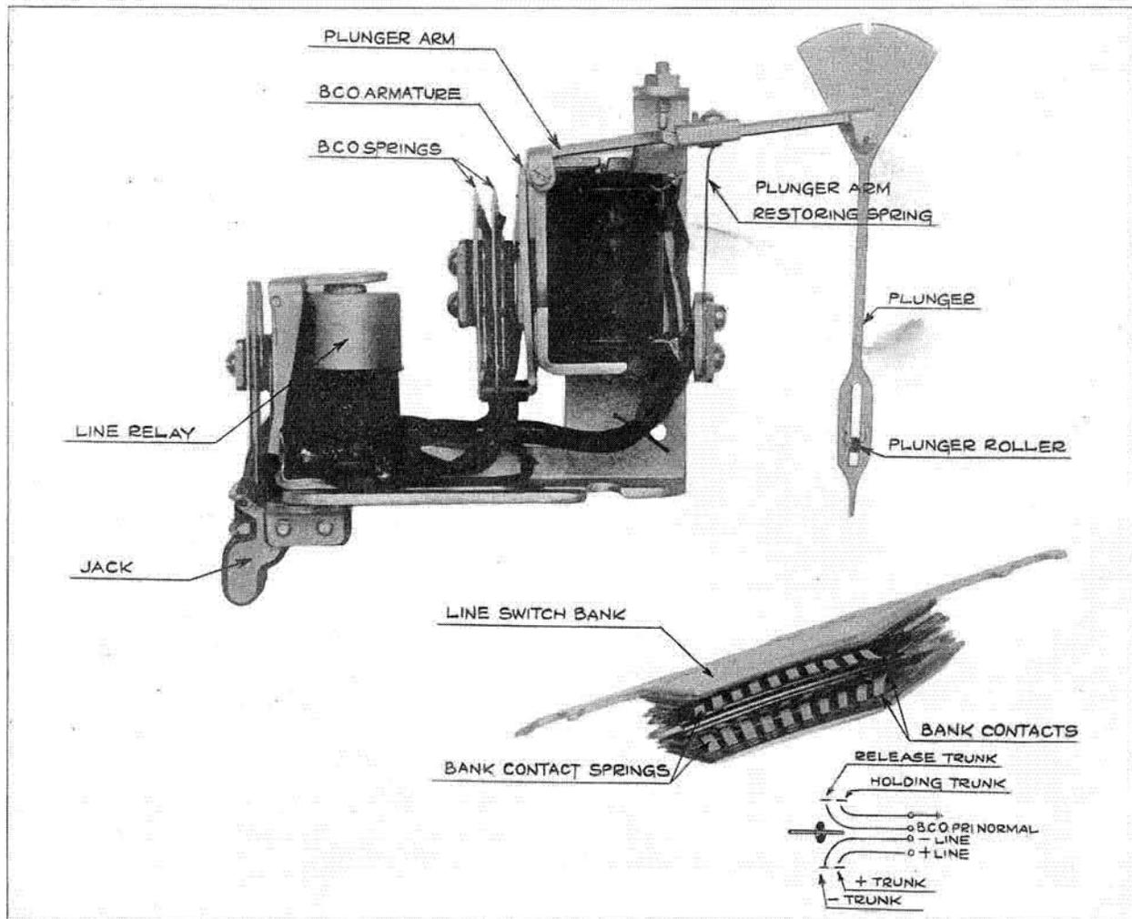
Fig. 34. Plunger type line switch and bank
