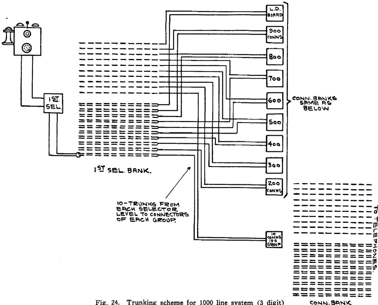
Fig. 24. Trunking scheme for 1000 line system (3 digit)
