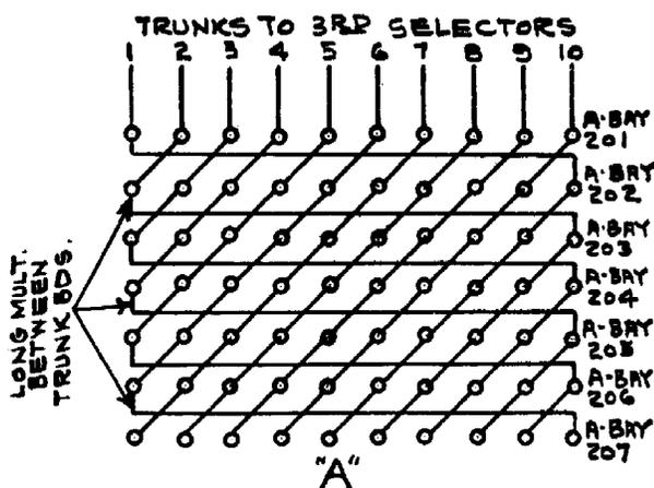
Fig. 72. Trunking scheme, second to third selectors
