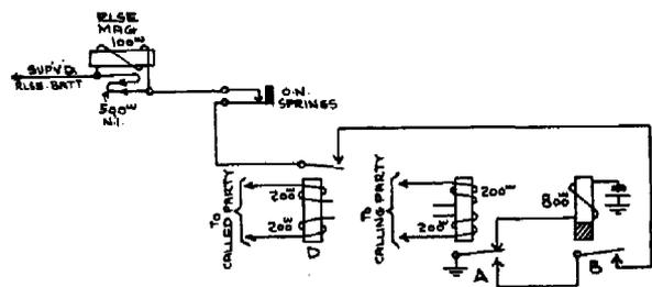
Fig. 19. Release circuit of connector
