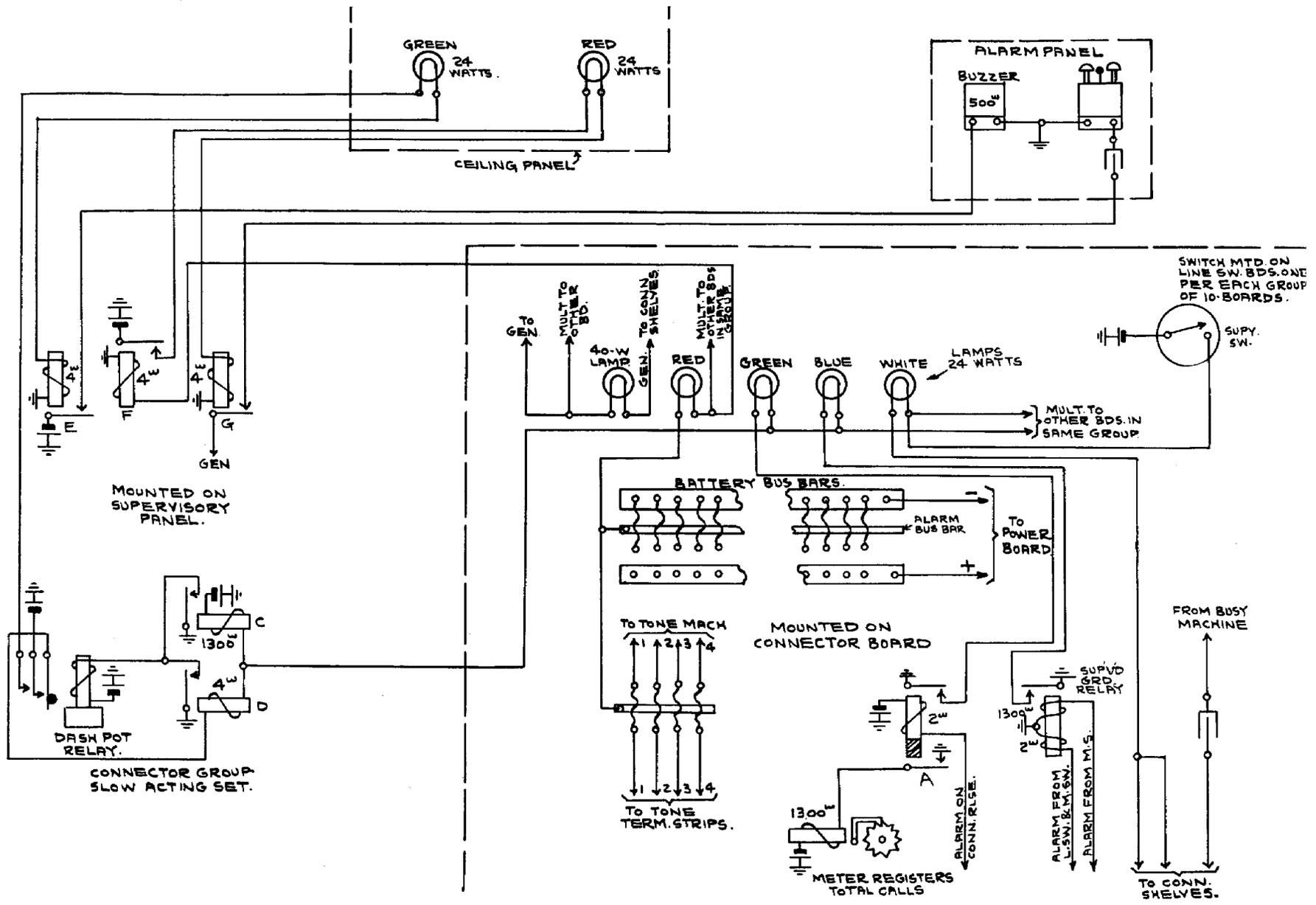
Fig. 59. Signal circuits for connector and line switch groups
