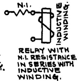
Fig. 1. Symbols used in telephone circuit drawings
