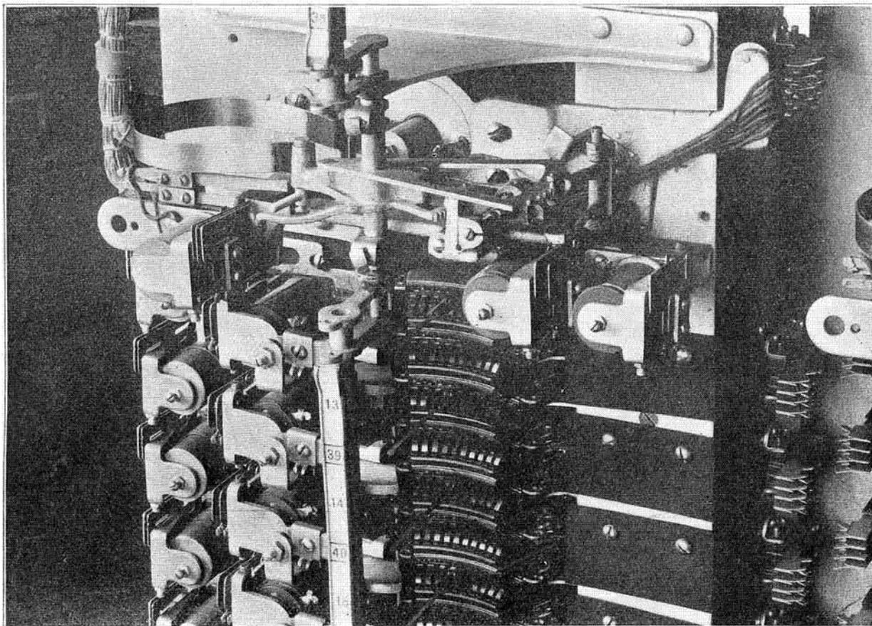
Fig. 42. Master switch and plunger guide shaft mechanism
