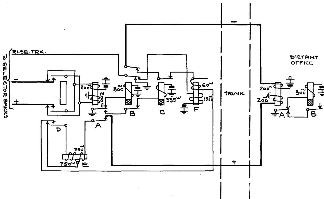
Fig. 52. Circuit of repeater ready for impulsing
