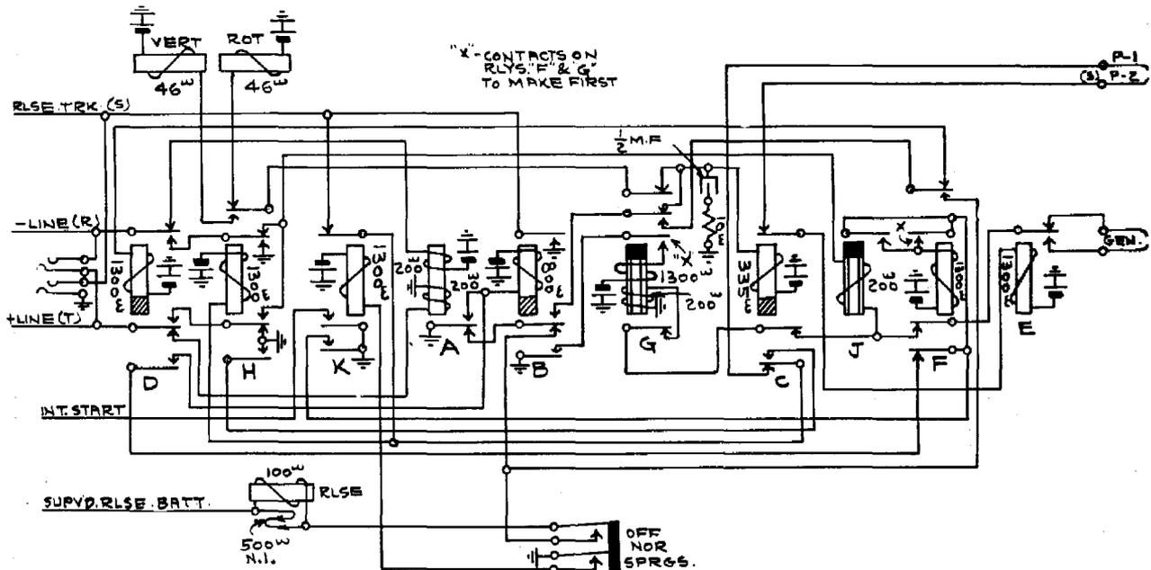
Fig. 94. Reverting call switch, complete circuit
