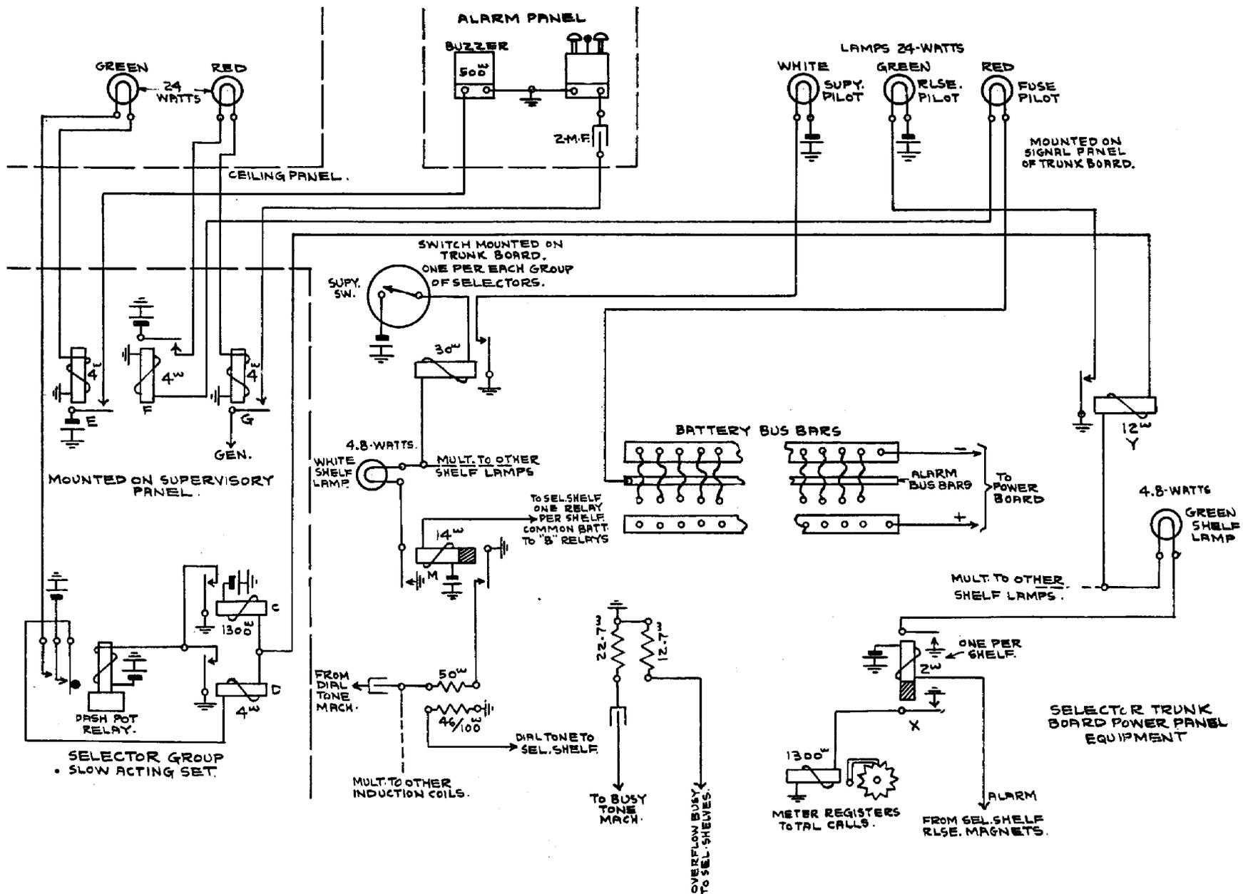
Fig. 60. Signal circuit for selector group
