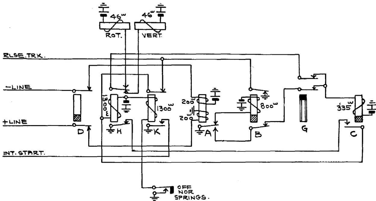
Fig. 92. Reverting call switch, impulse circuit
