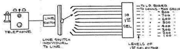
Fig. 37. 1,000 line system using line switches
