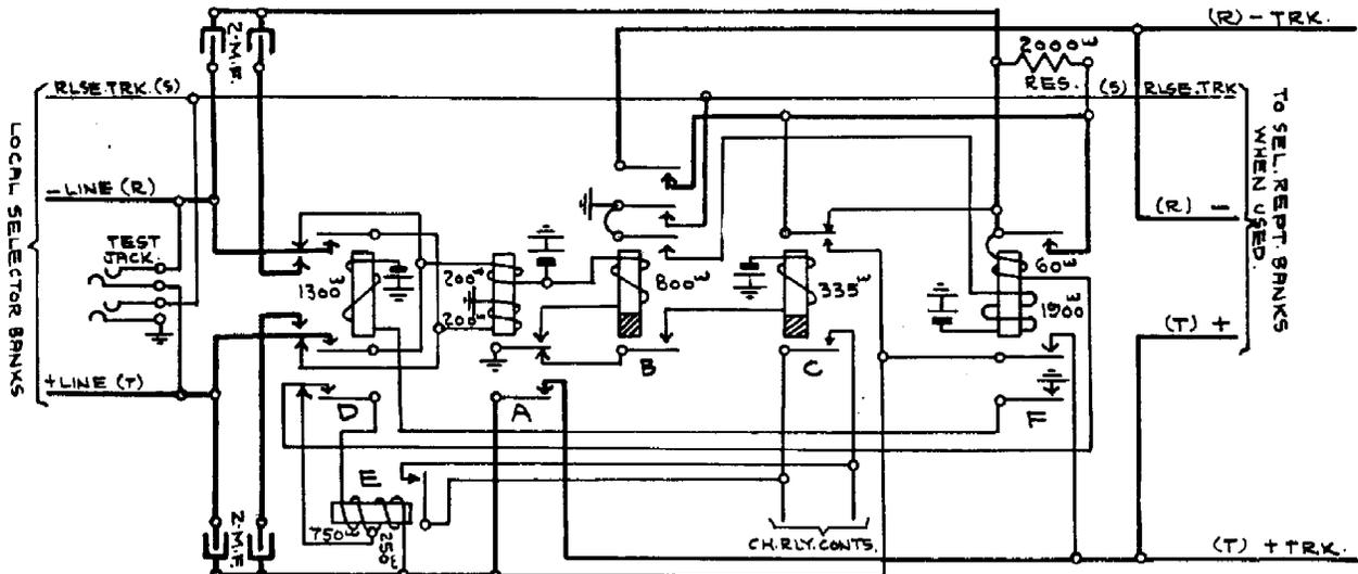
Fig. 55. Complete repeater circuit
