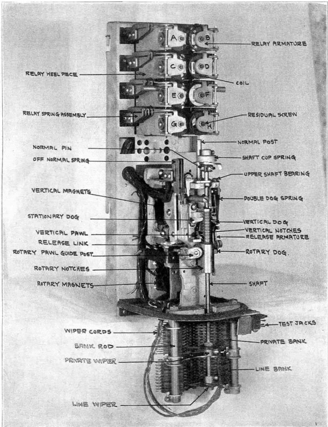
Fig. 10. Connector switch
