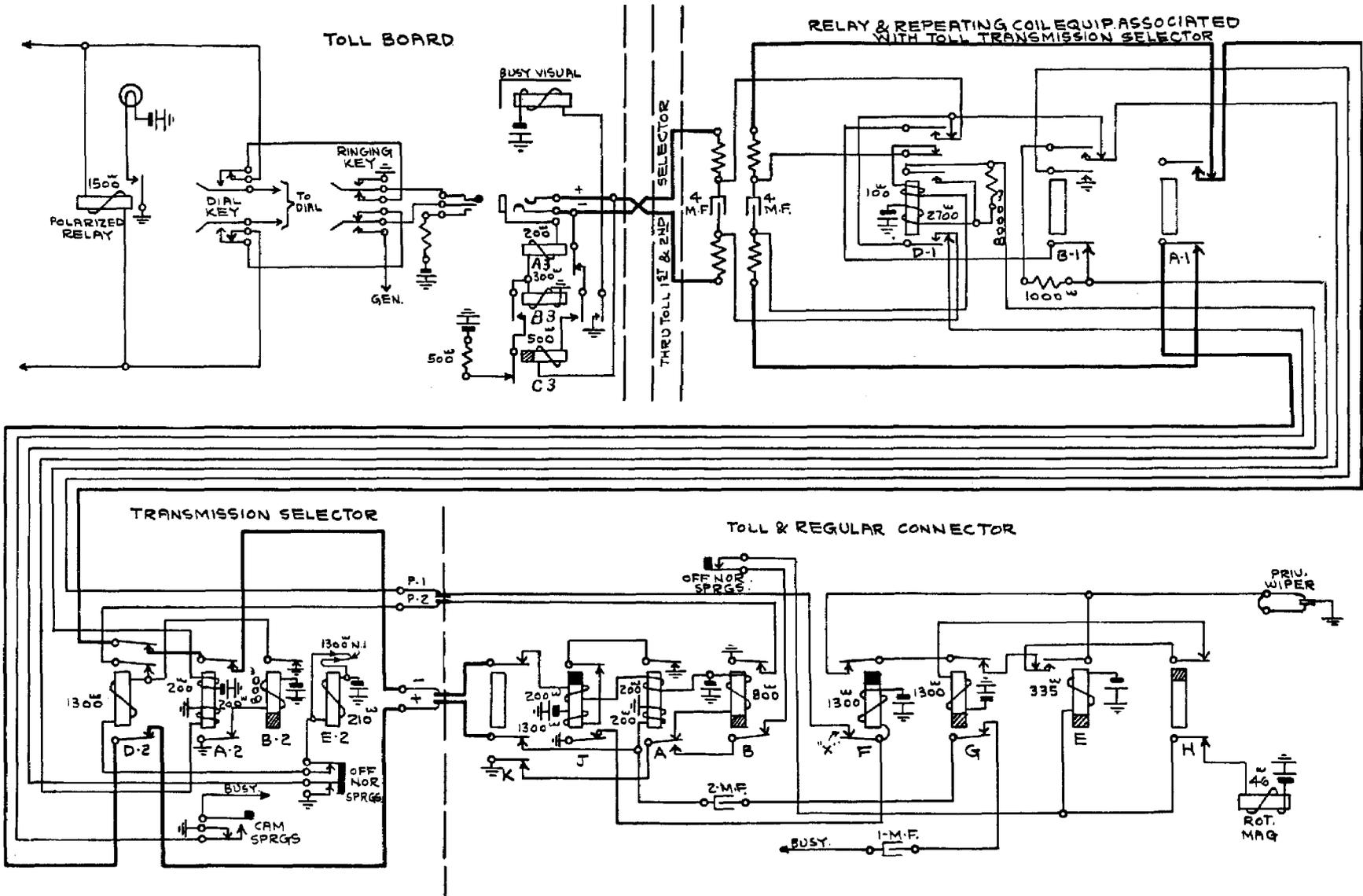
Fig. 81. Toll connection to subscriber's line, giving busy supervision to operator
