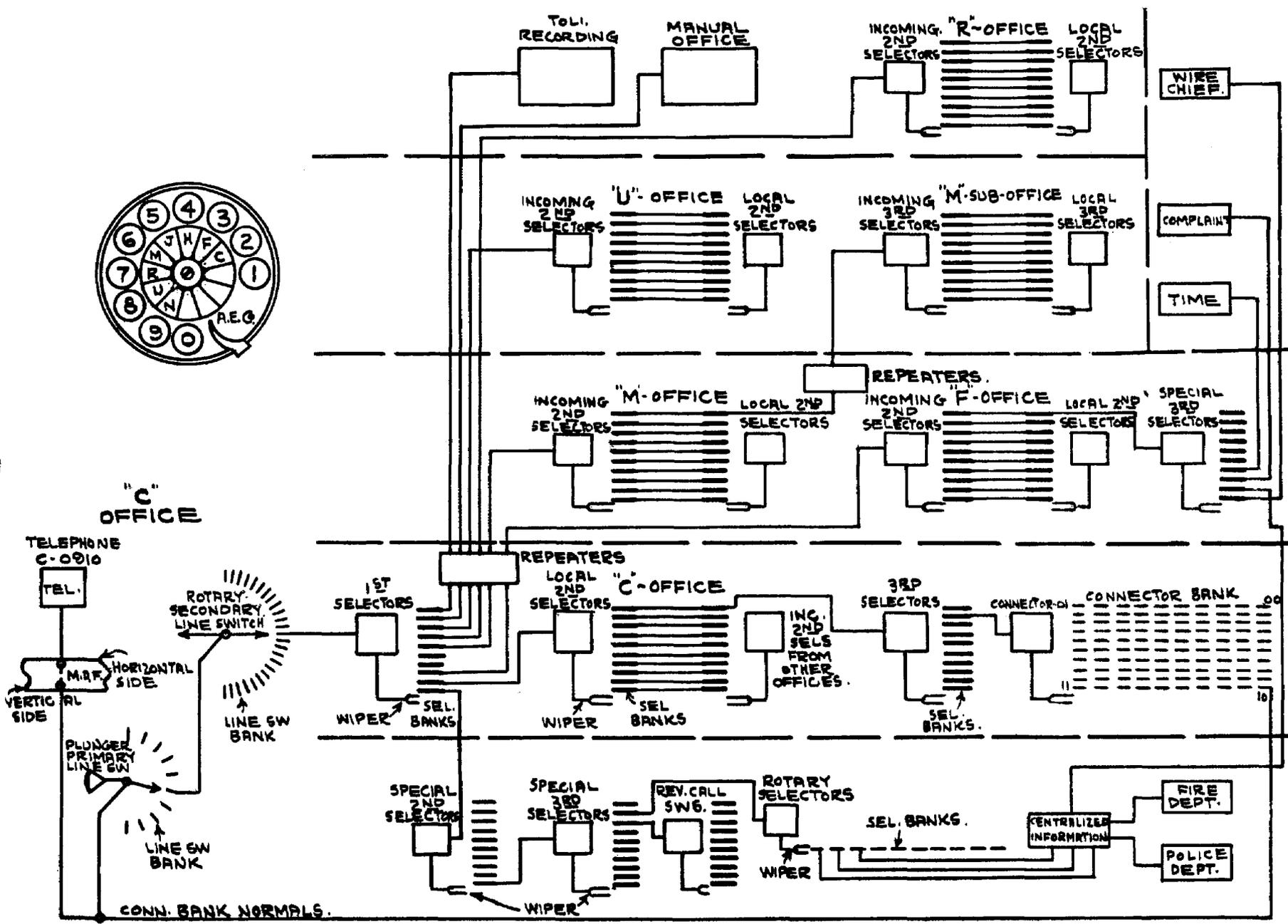
Fig. 61. Trunk layout for 100,000 line system
