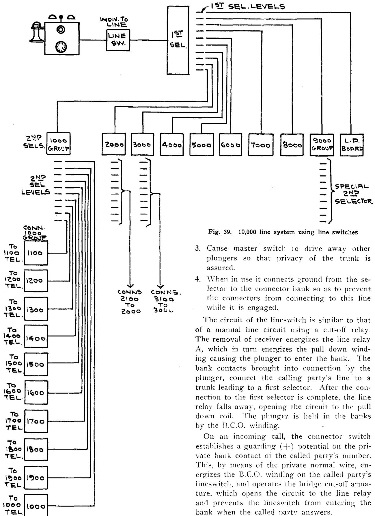
Fig. 39. 10,000 line system using line switches
