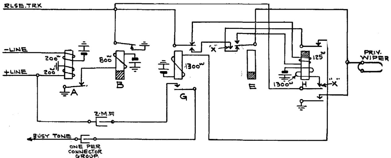
Fig. 14. Circuit showing busy test of called line
