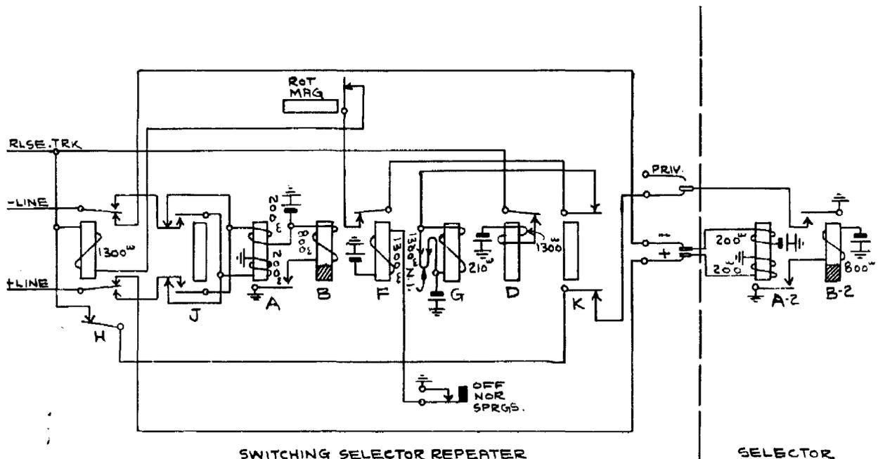
Fig. 89. Switching selector repeater after being switched through to succeeding selector in same office
