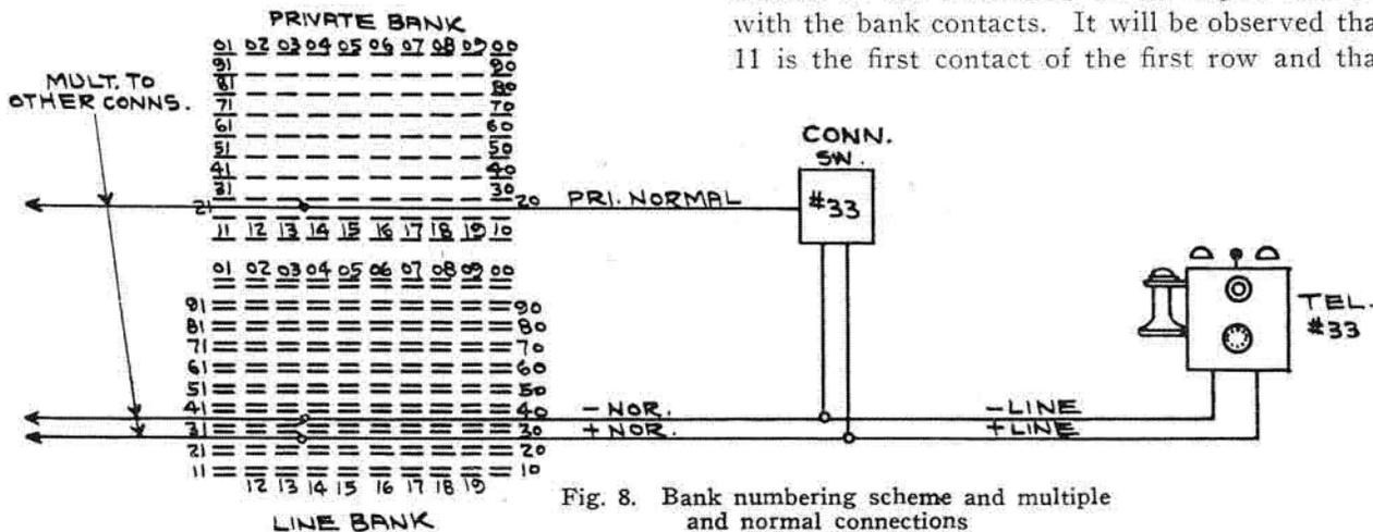
Fig. 8. Bank numbering scheme and multiple and normal connections
