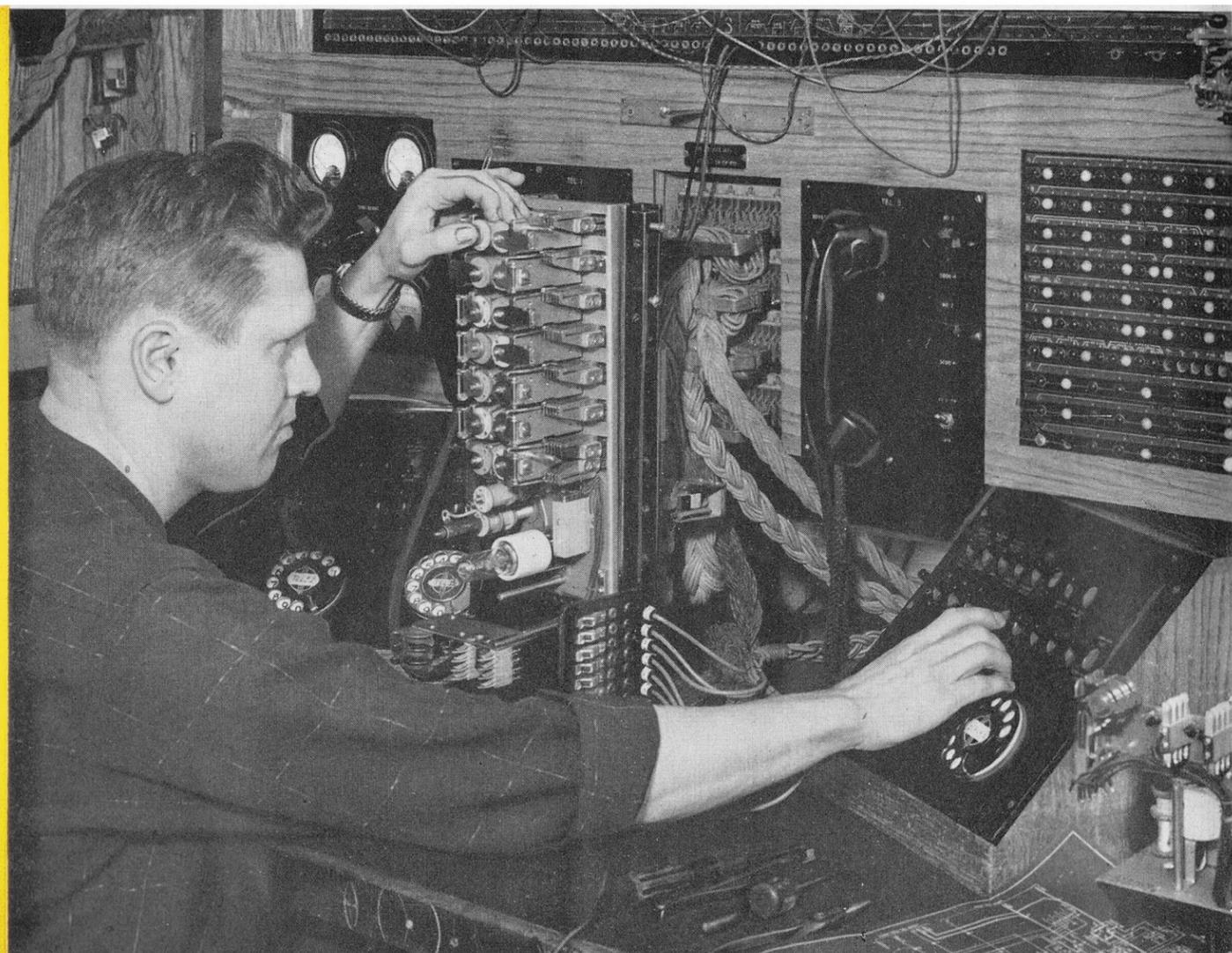
**J**ust before it is shipped, your Strowger Automatic telephone equipment proves its fitness for your specific service. Each unit is put through its paces under conditions as close as possible to those in your exchange. Strowger *must* pass these tests with flying colors before it is tagged "OK to ship."
