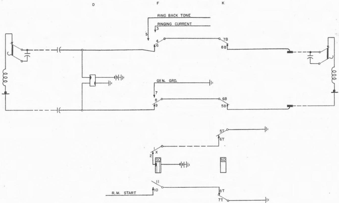
Figure 14. Relay F has operated fully. Ringing cut off.
