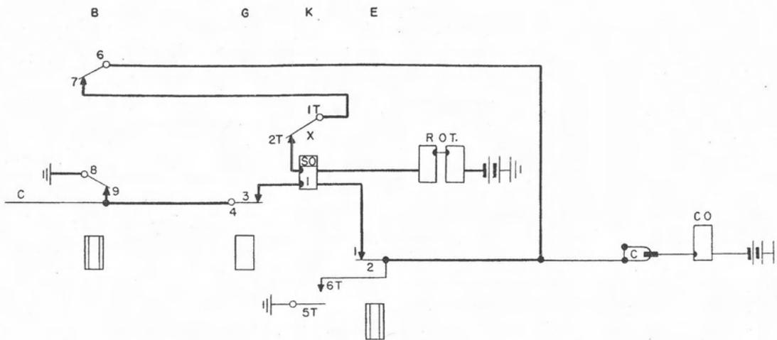
Figure 10. Seizure of the called line. Relay K winding #1 has just closed contacts "X".
