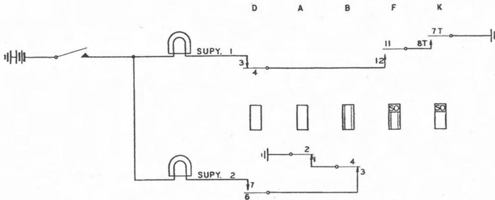
Figure 23. Supervisory circuits of an idle connector.
