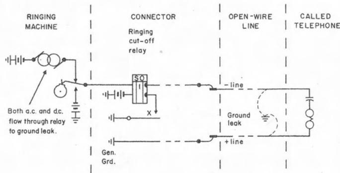
Figure 21. Battery-connected generator, showing a fault drawing a.c. AND d.c. thru ringing cut-off relay.
