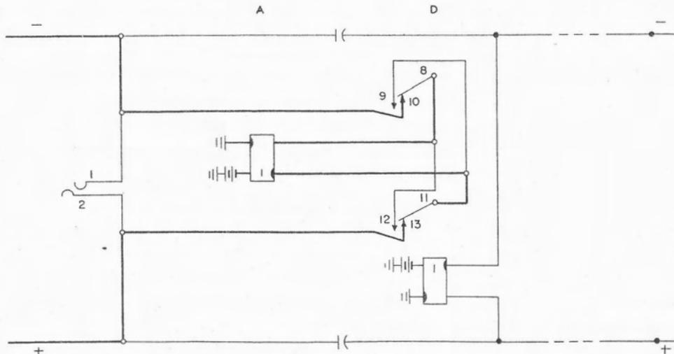
Figure 15. Caller's transmitter-current polarity reversed.
