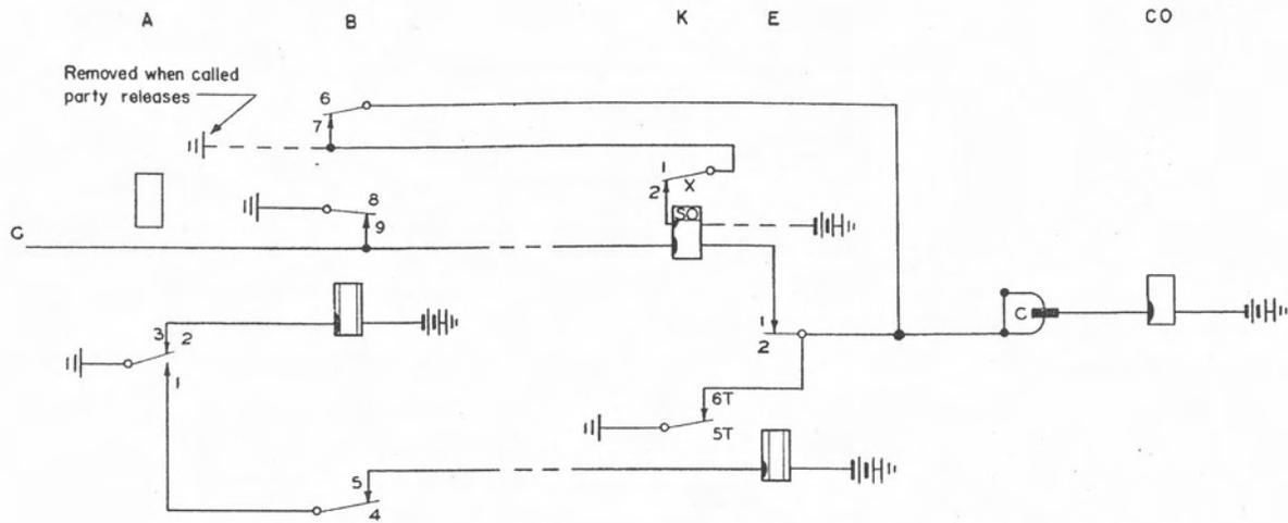
Figure 18. Connector circuits for dropping preceding switches.
