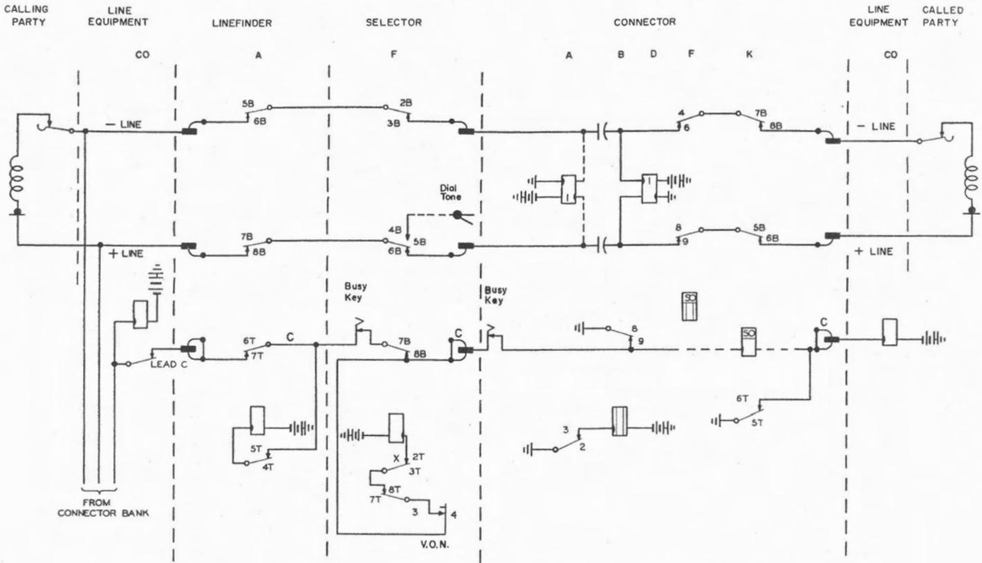
Figure 16. Conversation thru local switch train in a 1000-line central office.
