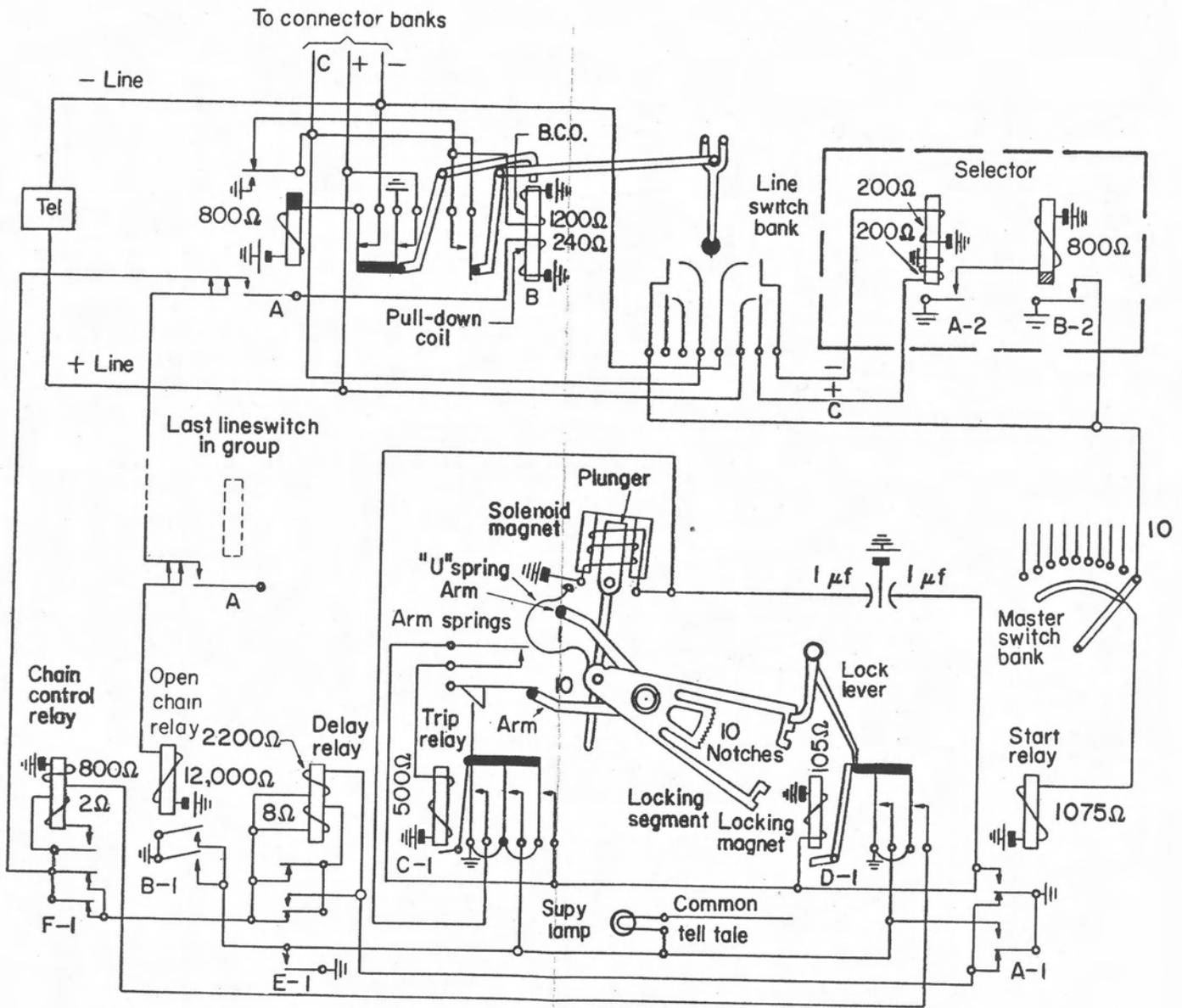
Figure 4. Circuit of self-aligning plunger lineswitch, master-switch, and parts of a selector.
