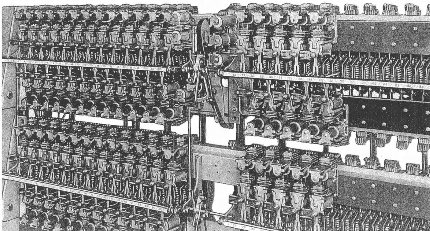
Figure 2. Master-switch and self-aligning plunger lineswitches.
