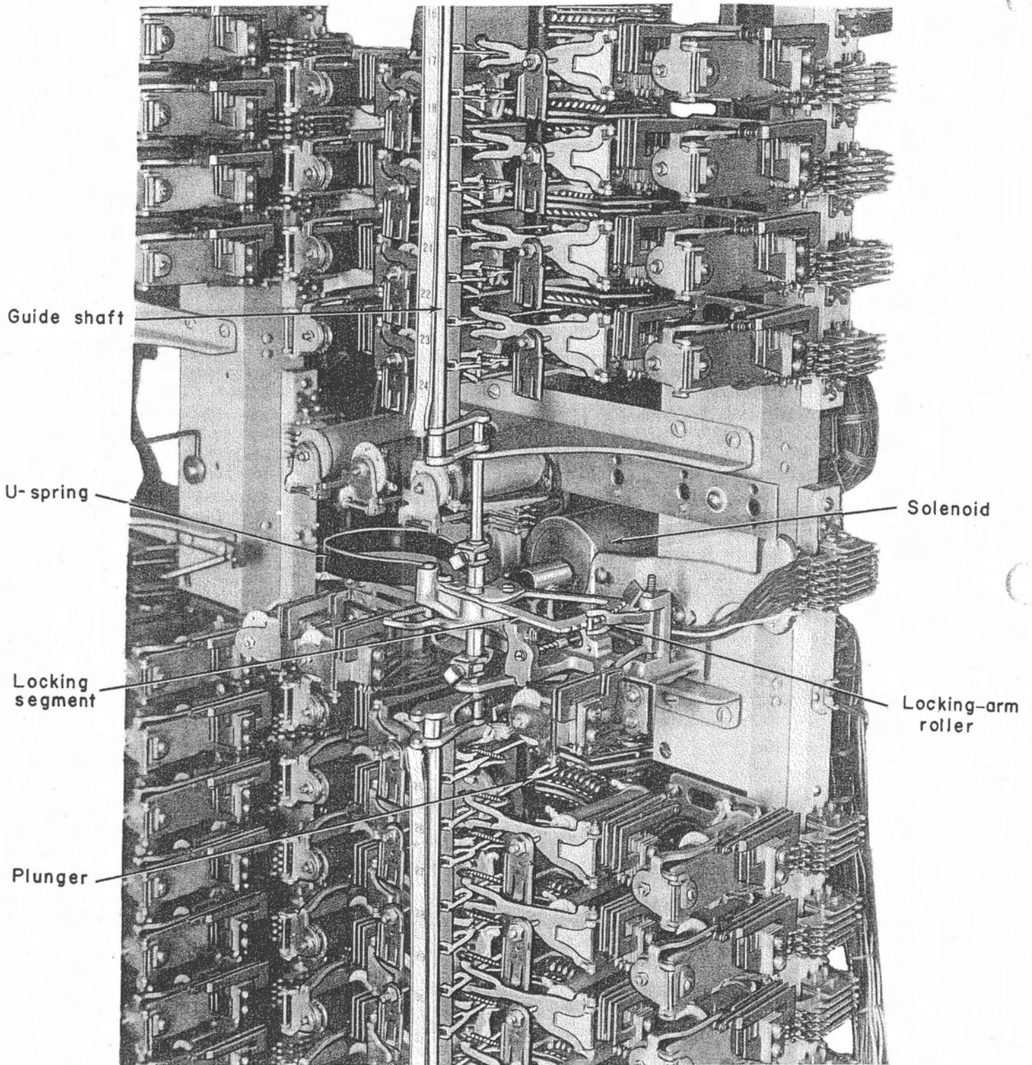
Figure 1. Master-switch and self-aligning plunger lineswitches.
