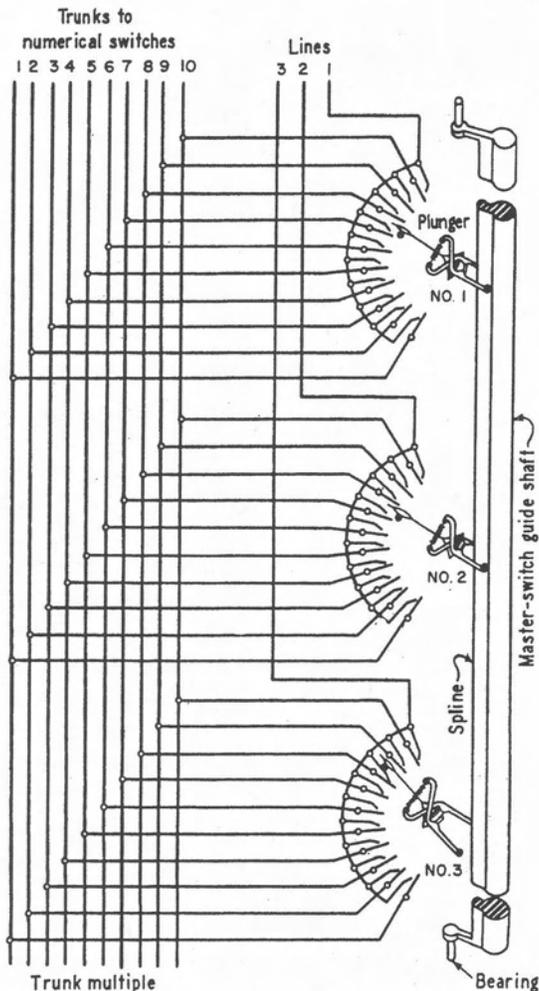
Figure 3. Relation of plunger lineswitches and trunks.
