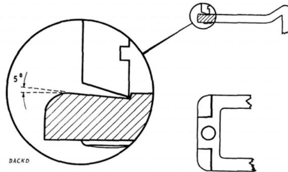
★FIG. 3. ARMATURE WITH 5° TILT
