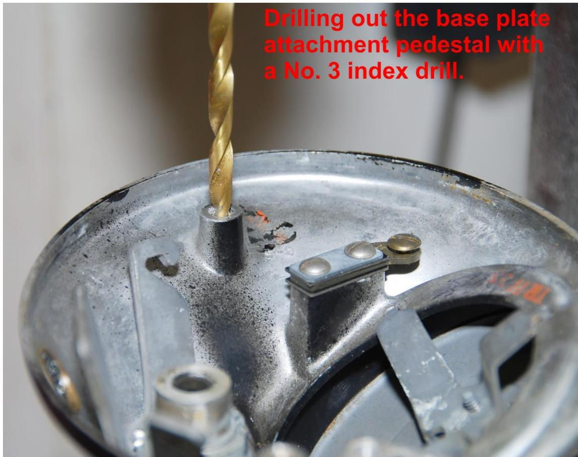
Once the pedestal hole is enlarged by drilling it out, set the housing aside for a minute, and install a  $\frac{1}{4}$  - 28 regular tap in the chuck of the drill press.
