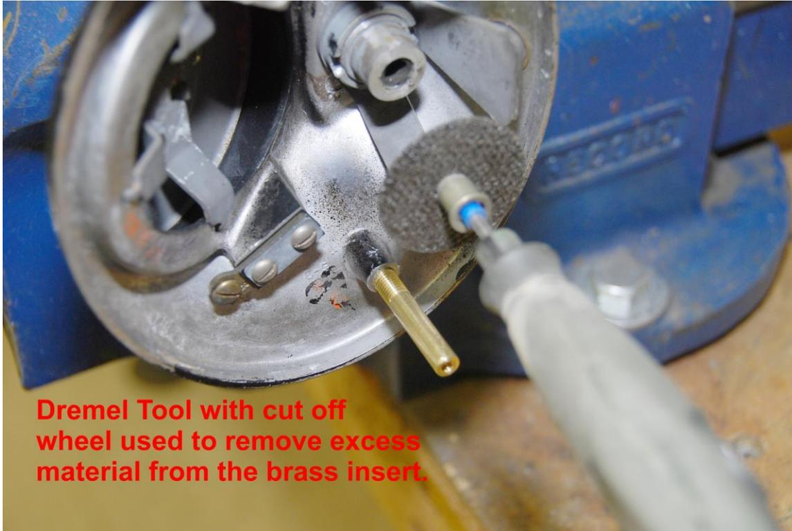
**Dremel Tool with cut off wheel used to remove excess material from the brass insert.**
