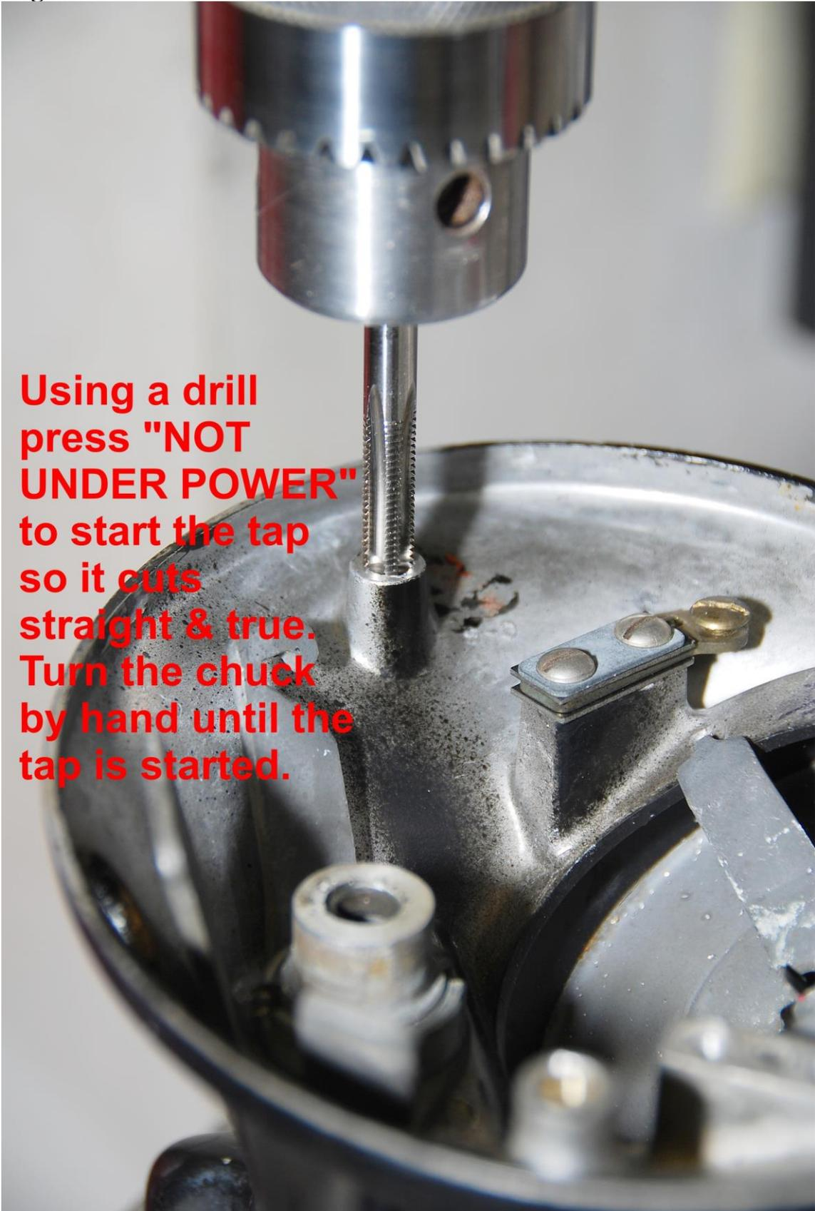
Using one hand to hold the telephone case firmly on the drill press table, turn the chuck with the tap installed, clockwise (that's clockwise when looking down at the pedestal, or, the normal direction in which a drill press would turn if under power). Just turn the chuck  $\frac{3}{4}$  of a turn and crank the drill press table up slightly, to compensate for the tap cutting into the telephone case pedestal.
