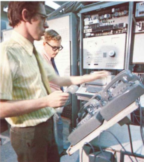
Bell-Northern Research has designed communications switching machines for a wide range of sizes, passbands and features. Control techniques range from electromechanical to wired logic electronic to fully stored program control. Similarly, switching matrices have run the gamut from electromechanical to space division electronic to time division pulse amplitude modulation (PAM).
