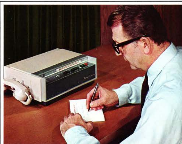
INCOMING MESSAGE VOLUME STAYS AT AUDIBLE LEVEL whether loop resistance is normal, high or low. Automatic Volume Control feature smooths out recording level—helps make sure that all messages will be clearly understood by the subscriber.
