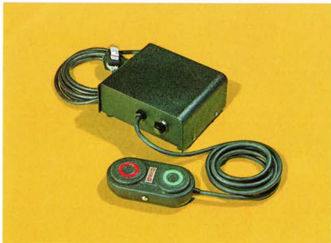
FOOT CONTROL enables the attendant to start, stop, rewind and backspace the play-back mechanism while keeping both hands free for typing. Foot control is also available without backspace feature.
