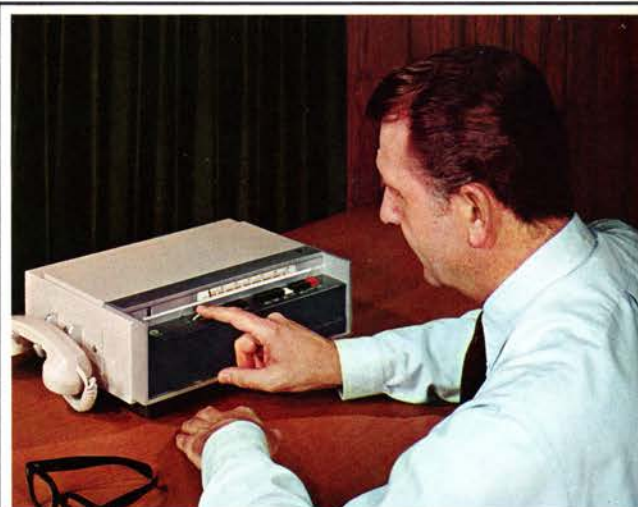
SUBSCRIBER CAN LISTEN TO MESSAGES AS THEY COME IN, using the "Message Monitor" feature on the LP-3. He can adjust the volume control for any desired speaker volume, as shown. Should he wish complete privacy, he can turn the volume down and listen with the handset.
