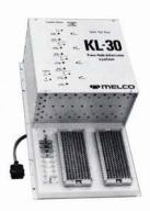
KL-30 Two-Link Intercom System: Provides up to 40 stations with two private talking paths, call progress tones, flashing lamps, interrupted ringing and lockout. Only one telephone pickup key is required to access all stations and both links. Switch-selectable PABX features include specific call pickup, call forwarding, conferencing, message waiting and do-not-disturb. Paging, outside line access and call announcing capabilities are circuit pack options.
