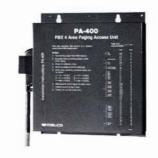
PA-400 Four-Area PABX Paging Access Unit: Provides paging access through a PABX station to up to four paging areas which may be accessed separately or simultaneously. Any station user can access the paging amplifiers by dialing the assigned access code. Call attention tone and background music are optional. The PA-400 provides 600 ohm impedance and is compatible with Melco's MAX Communication Systems.
