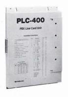
PLC-400 PBX Line Card: A 1A2 type key system line card which allows up to 4 C.O. lines to be added to a MAX Communication System or similar PABX system. Designed to enable key telephones to be used with the PABX installation, the PLC-400 provides lamp control, bell or buzzer ringing and line hold. Input ports are available to allow the PABX stations controlled access to the same C.O. lines as the key telephone stations.
