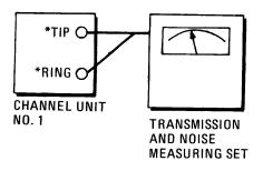
\*Make connections to TIP 1 and RING 1 on 4-wire channel units.
