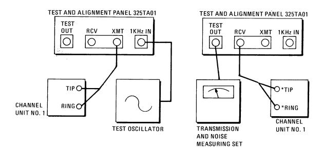
\*TIP 1 and RING 1 on 4-wire channel units.
