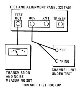
\*Make connections to TIP-1 and RING-1 jacks on 4-wire channel units.
