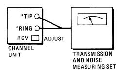
\*Make connection to TIP 1 and RING 1 on 4-wire channel units.
