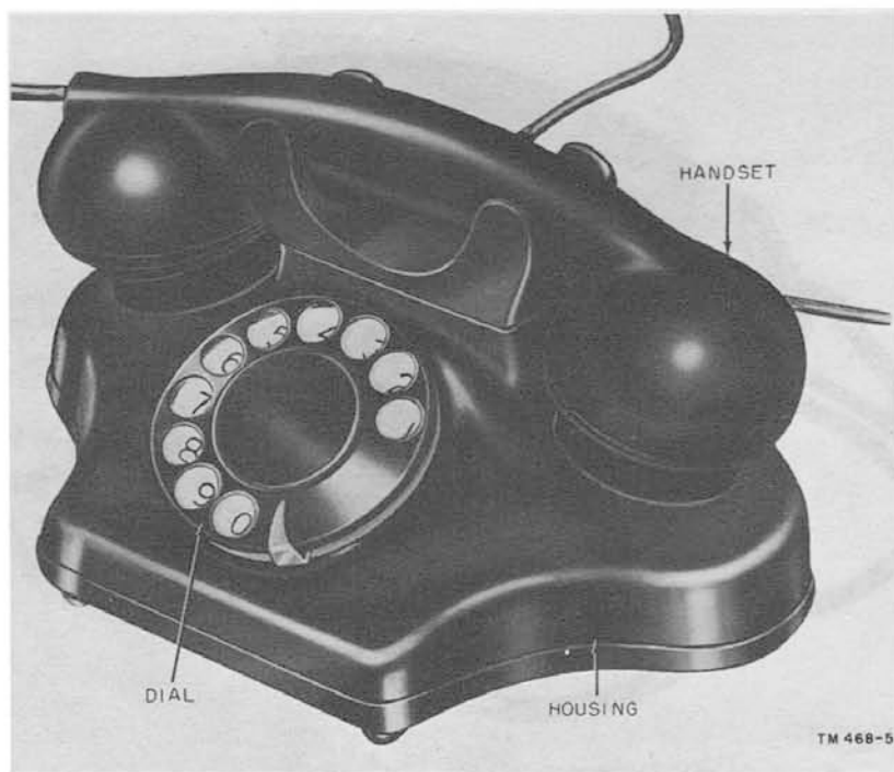
Figure 6. Telephone TA-102/FTC (Kellogg No. 925BAX), arranged for dial operation.
