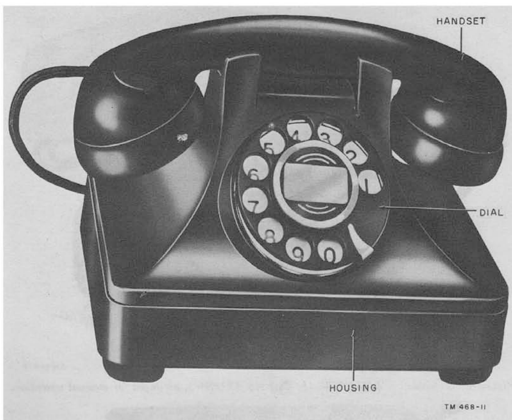
Figure 10. Telephone TP-6 (North Elec Mfg No. H-600SL and No. 3H6SL), arranged for dial operation.
