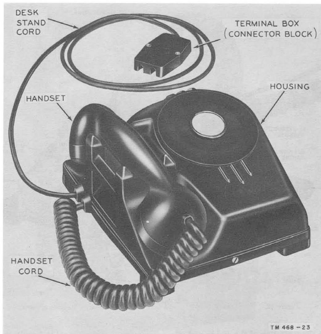
Figure 22. Telephone TA-166/U, arranged for manual operation.
