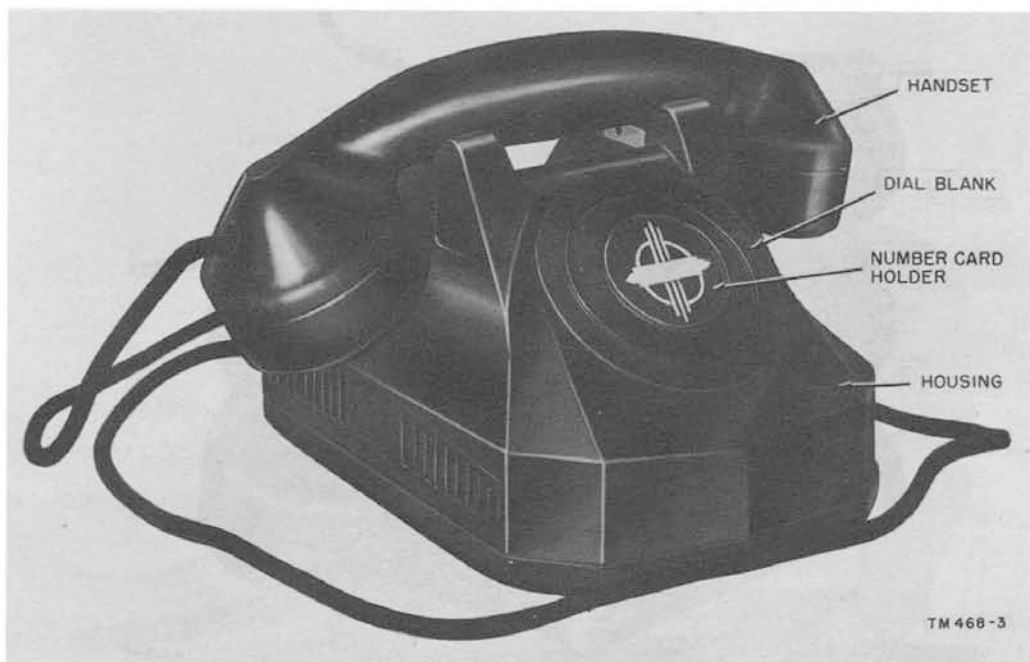
Figure 4. Telephone TA-101/FTC (Auto Elec No. 40), arranged for manual operation.
