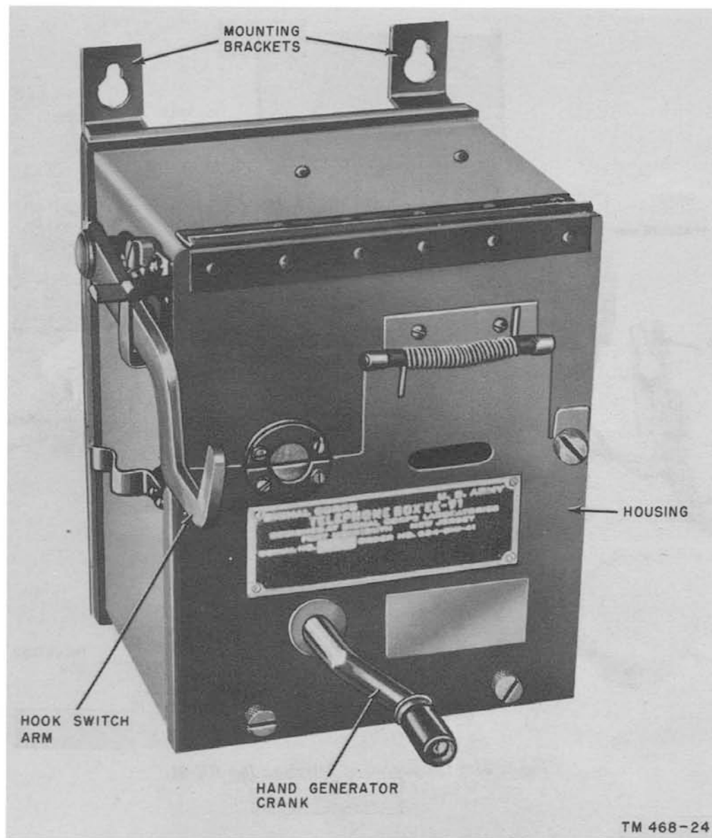
Figure 24. Telephone Box EE-91, common-battery telephone.
