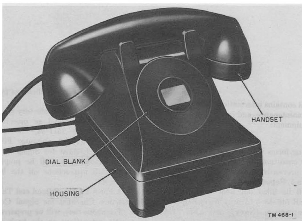
Figure 2. Telephone TP-6, arranged for manual operation.
