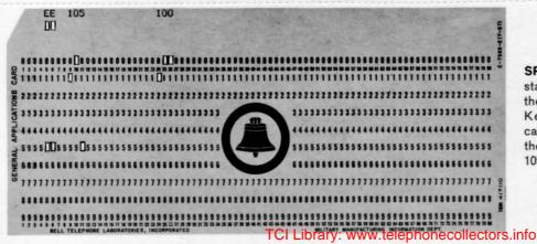
**SPEECH SOUNDS** are specified on standard punched cards in the new synthesized speech program devised by Kelly and Gerstman. This particular card instructs the computer to produce the sound EE (as in beat) at a pitch of 105 cps for 100 milliseconds.
