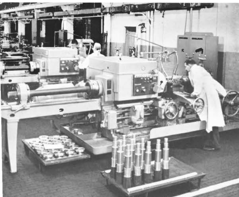
Turret lathe, redesigned on basis of human capabilities and limitations, reduces operator effort.
