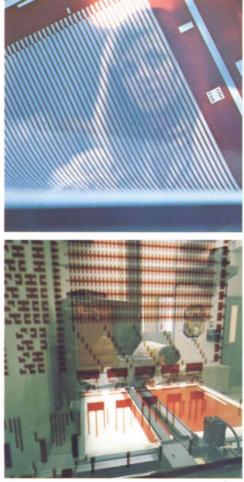
• permits standard metal oxide silicon (MOS) logic on the same chip for refresh and other control circuitry
