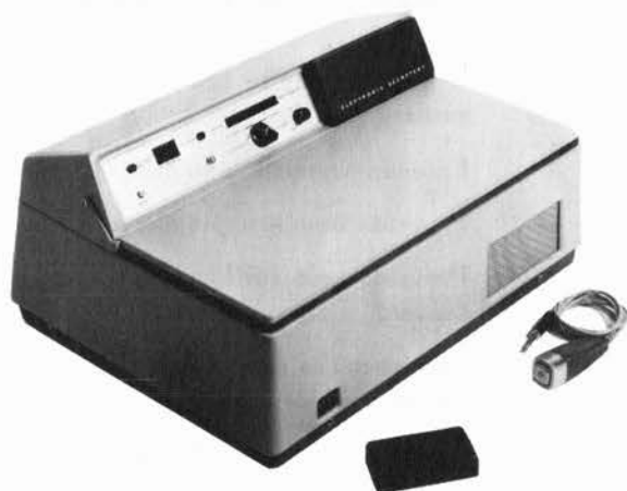
Model RFP Electronic Secretary Telephone answering set with microphone and personal call-back signaler for remote control.
