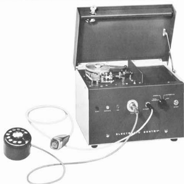
Electronic Sentry with microphone and dial used to record the report message.
