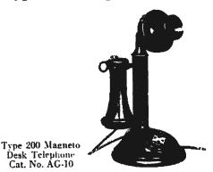
This telephone is identical in appearance with the Type 21 Manual Convertible Central-Battery Desk Telephone (see page 18), but has a local-battery transmitter, and is wired for use in the local-battery booster circuit. A 6-foot, 3-conductor Monotype cord is provided for connection to the ringer box and battery.
