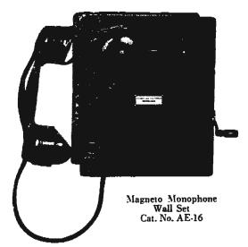
Cat. No. AE-16 contains a specially-designed generator providing a higher voltage of ringing current, and a special 2500-ohm ringer with exposed gongs. This instrument is designed for use on long and heavily loaded lines where a very loud ringing signal is desired.
