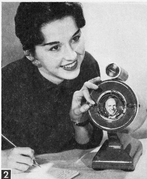
2 Bell Laboratories engineers envision one use for this television-telephone, the Picture Phone , in an executive's office. Here a secretary uses one of the knobs to decrease volume. Lens at the top of the set transmits her picture.
