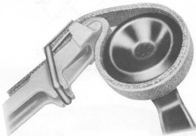
Fig. 2—Correct Positioning of the 514B Tool
