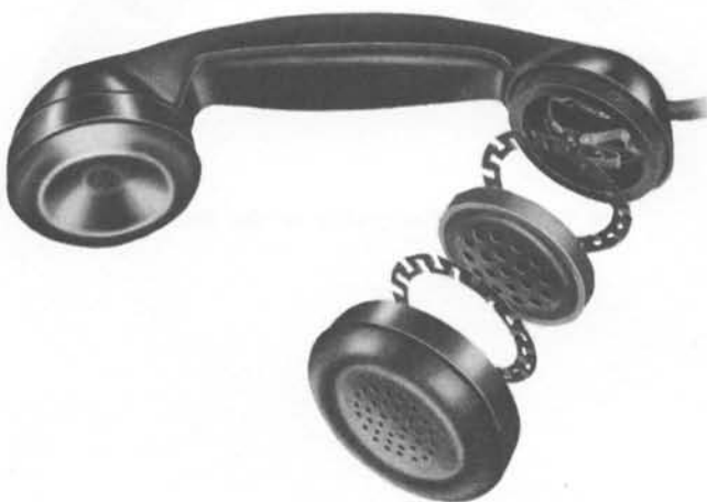
Fig. 5—Lock KS-14200, Order of Assembly of Lock Transmitter Unit and Cap
