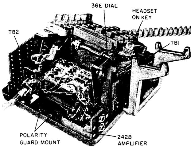
Fig. 4—2664A1 Telephone Set, Housing Removed
