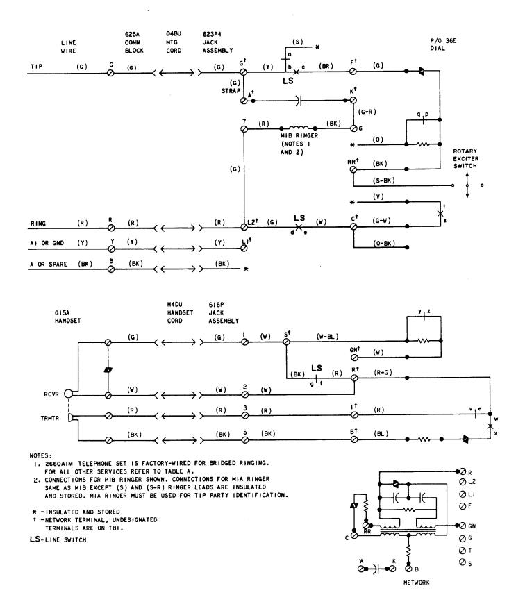
Fig. 1—\$2660A1M Telephone Set, Connections\$
