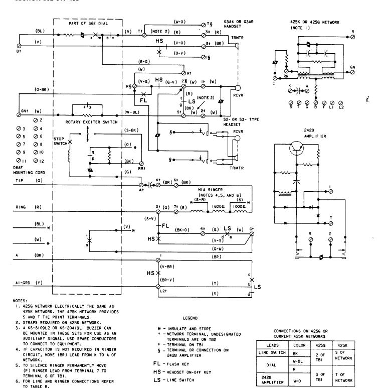
Fig. 1—2663A1 Telephone Set Connections
