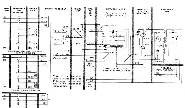
When telephone set is used with 1A1 key telephone system, switch contact ed must break last when handset is
