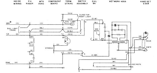
Note: For manual service, remove lead from Terminal F and connect to RR and remove white dial lead from Terminal GN and connect to R1.
