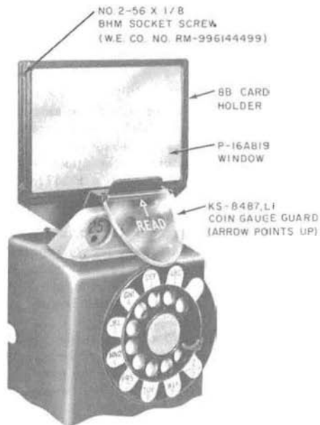
Fig. 9—Dial Type Coin Collector Equipped with Coin Gauge Guard
