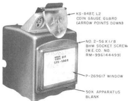
Fig. 8—Manual Type Coin Collector Equipped With Coin Gauge Guard
