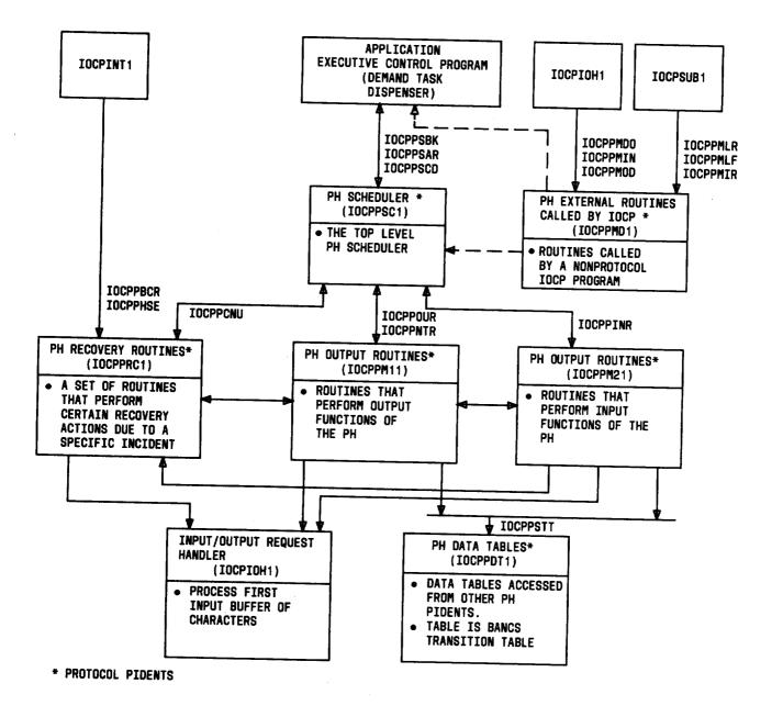
Fig. 5—IOCP High Speed I/O Protocol Pident Interfaces
