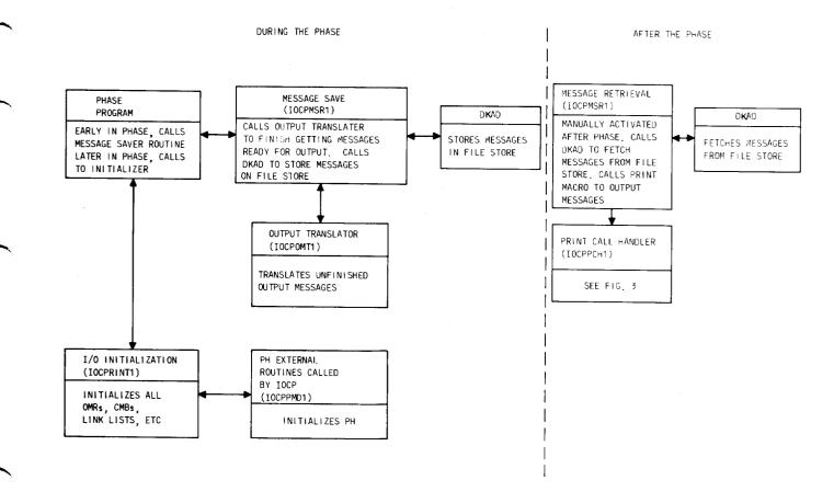
Fig. 4—IOCP Actions During Phase of Software Initialization
