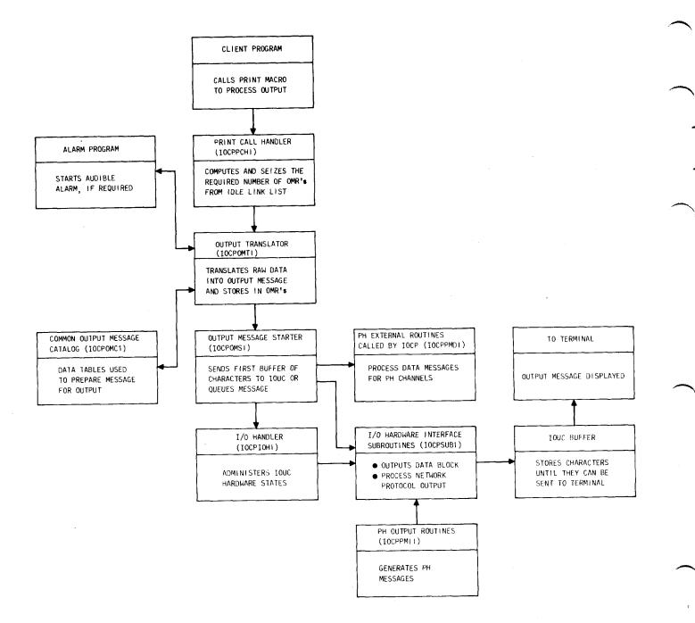
Fig. 3—Output Message Processing
