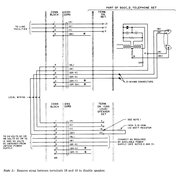
Note 2: Connect negative (-) side of battery to terminal 10 to disable ON-OFF switch.
