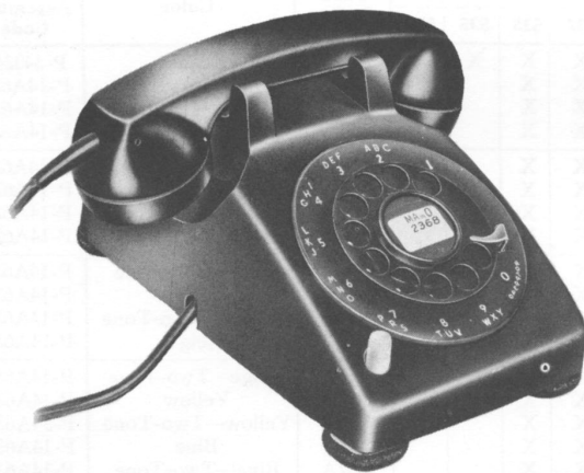
Fig. 1—Telephone Sets Equipped with Transistorized Amplifiers—External
