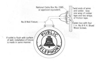
Fig. 13 - No. 8 Sign - Wall Installation
