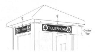
Fig. 9 — Installation of No. 26 Sign on Booth
