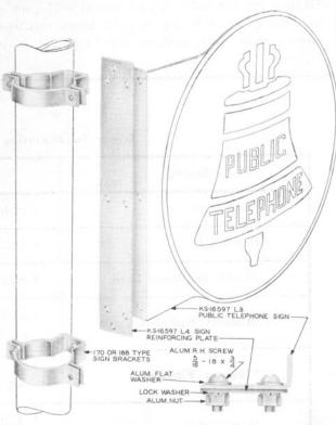
Fig. 3 — KS-16597, List 4 Sign Reinforcing Plate with 170- or 188-type Sign Brackets
