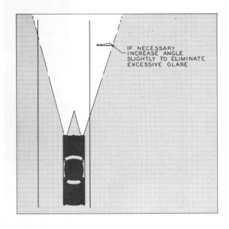
Fig. 20 — KS-16540 Sign — Angle Increased to Eliminate Excessive Glare
