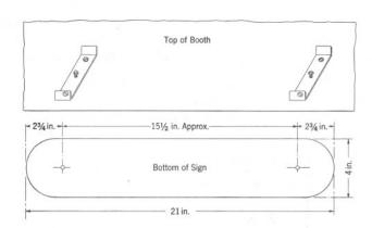
Fig. 5 — Installing KS-14154, List 4
