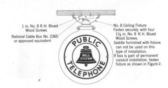
Fig. 12 - No. 8 Sign - Ceiling Installation
