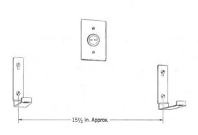
Fig. 4—Installing KS-14154, List 3 Brackets to Vertical Surface
