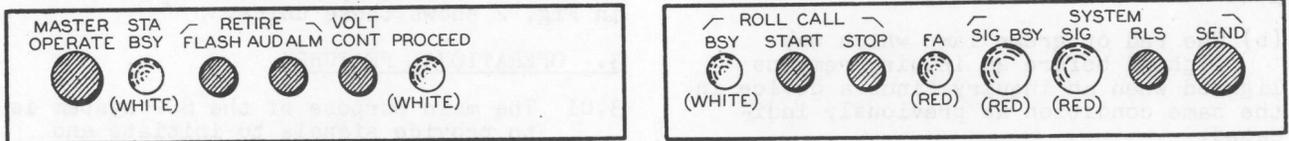
Fig. 4 - Common Control Keys and Lamps on Main Station Console
