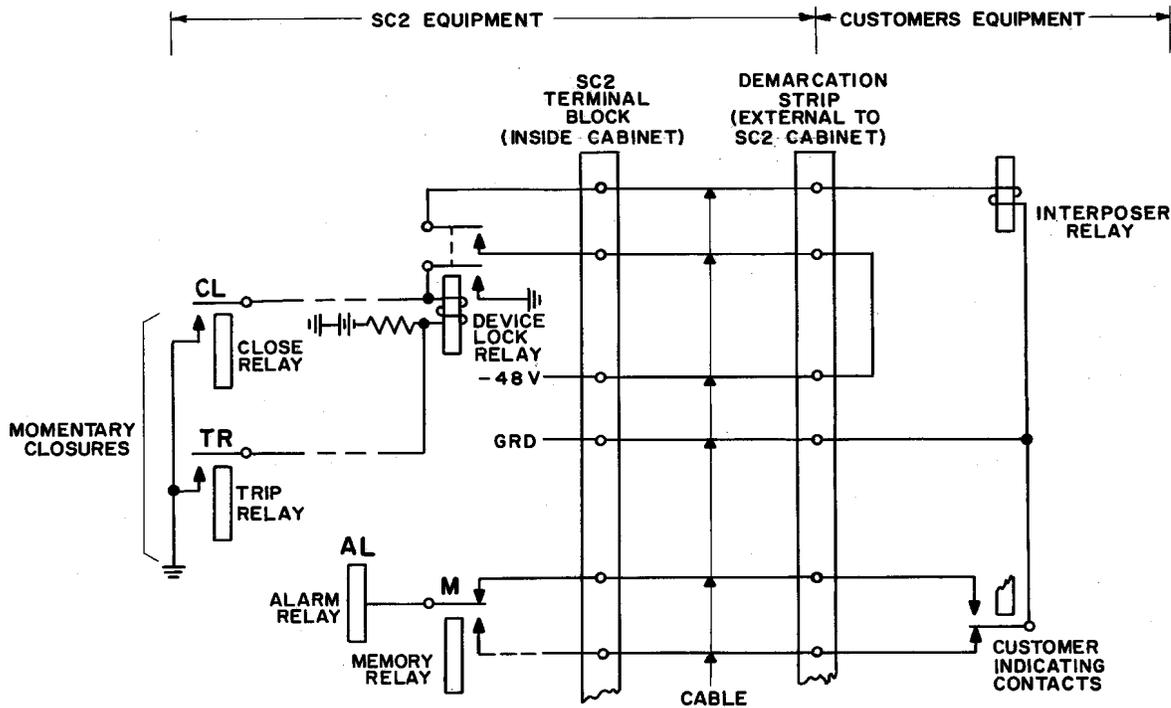
Fig. 9 - Typical Connection to Customer's Equipment
