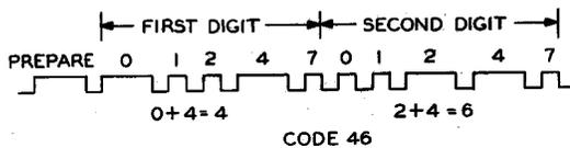
Fig. 7 - Typical 2-digit Pulse Length Code
