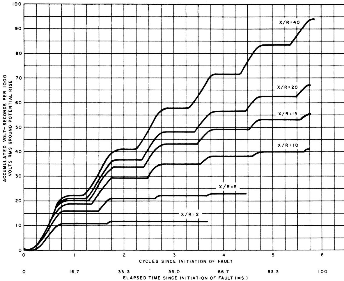
Figure 6 – Required Transformer Capability in Volt-Seconds Per 1000 Volts RMS Ground Potential Rise
