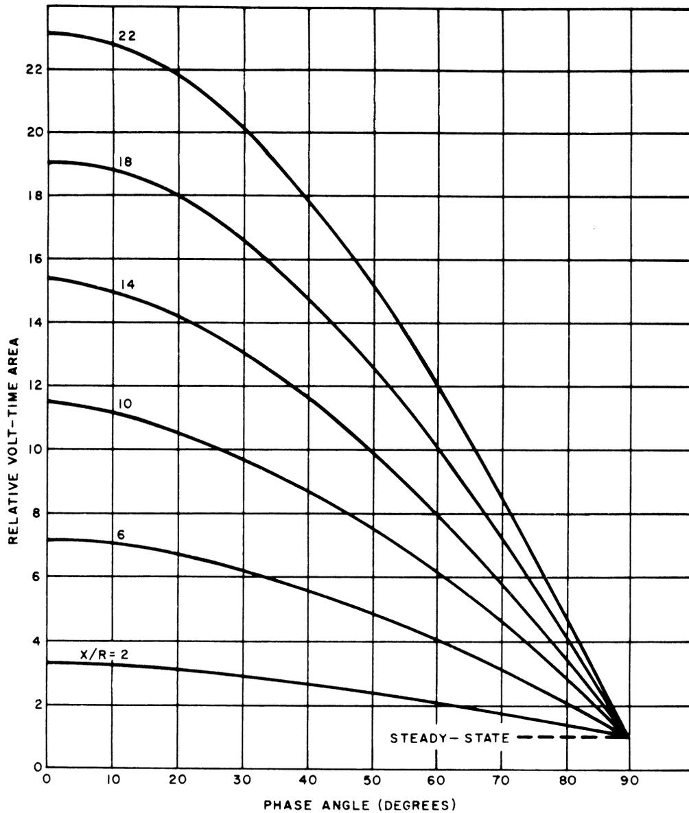
**Figure 3** – Relative Volt-Time Area (Asymptotic Value) For Various X/R Ratios As a Function of Power Line Voltage Phase Angle at Initiation of Fault
