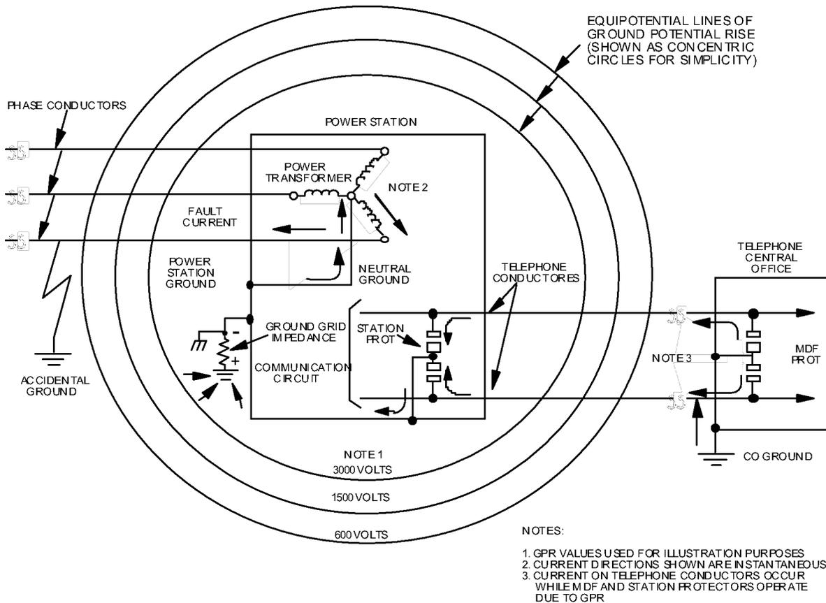
Figure 2 - Rise Potential of Power Station Ground Resulting from a Fault on the Power Line
