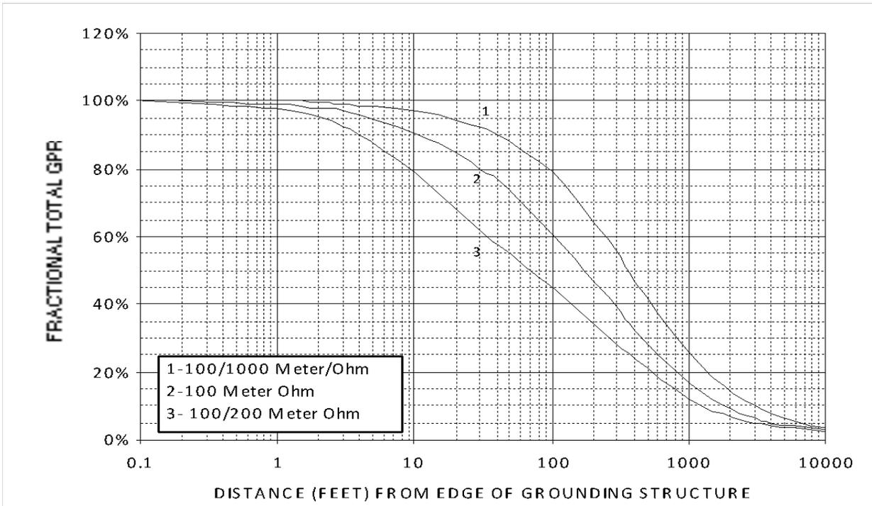
**Figure 5c** – 290,000 Square Feet: Ground Potential Distribution From Edge of Power Station Ground Grid With Respect to Remote Earth
