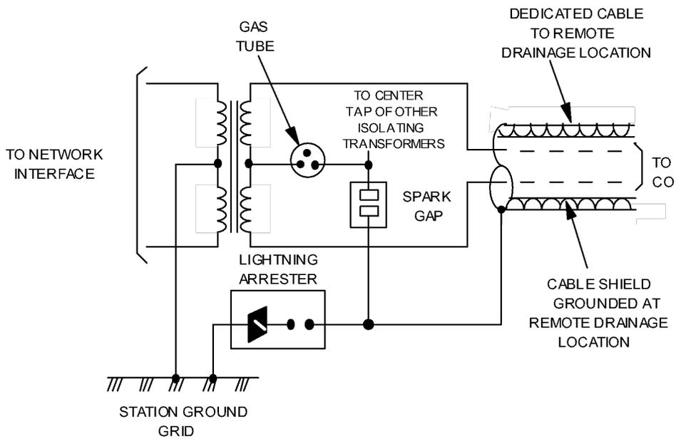
Figure 6 – Isolation Transformer – Typical Application
