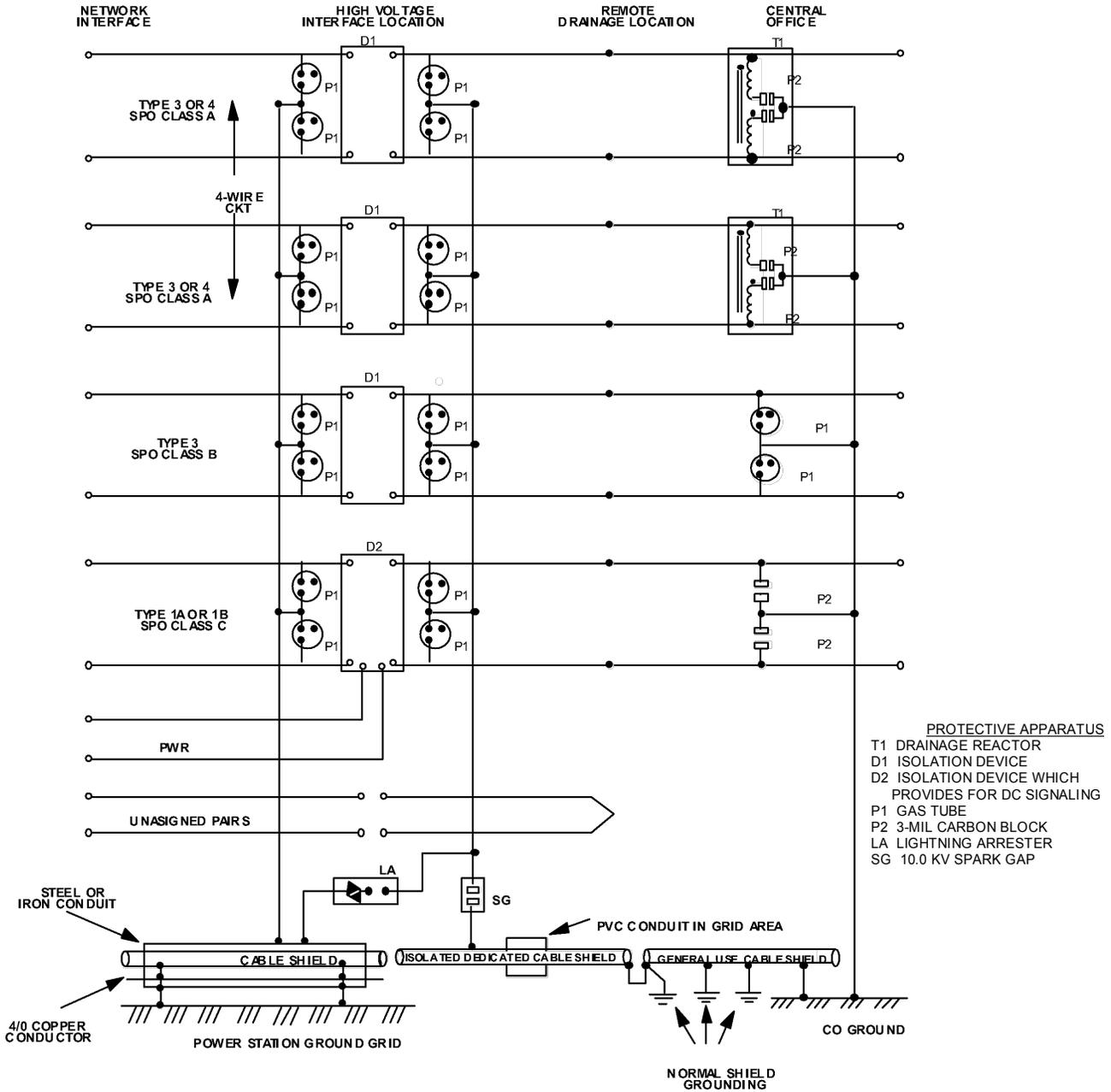
Figure 11 – Isolation System of Protection Using Modular Components
