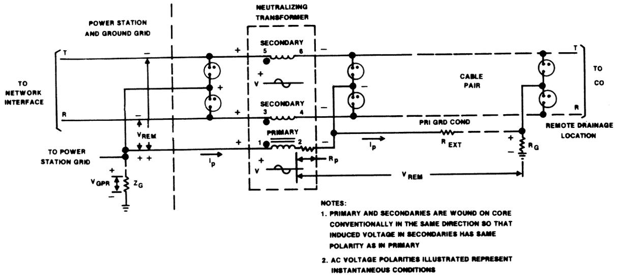
Figure 1 – 3-Winding Neutralizing Transformer – Neutralizing Ground Potential Rise at Power Station
