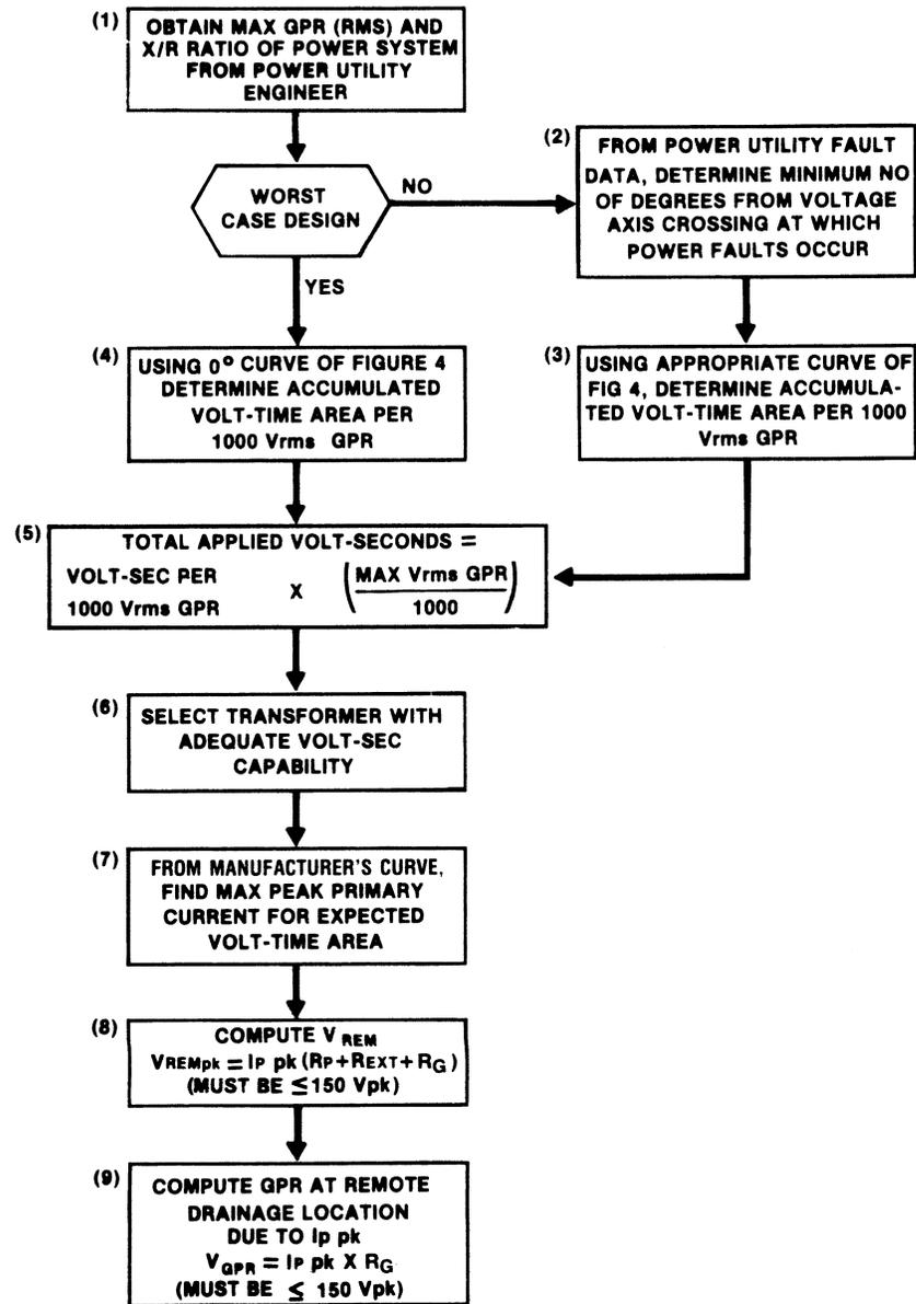
Figure 10 - Recommended Design Procedure For Neutralizing Transformer Installations
