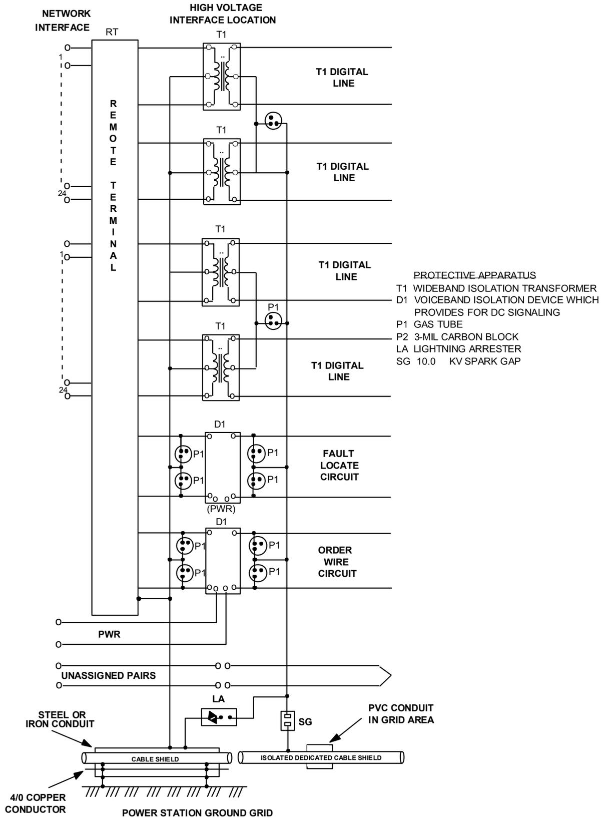
**Figure 13** – Isolation System of Protection for Carrier Systems – Connections at HVI for Multiple Digital Lines
