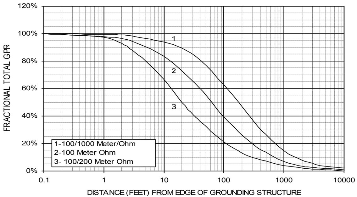
**Figure 5b** – 35,000 Square Feet: Ground Potential Distribution From Edge of Power Station Ground Grid With Respect to Remote Earth
