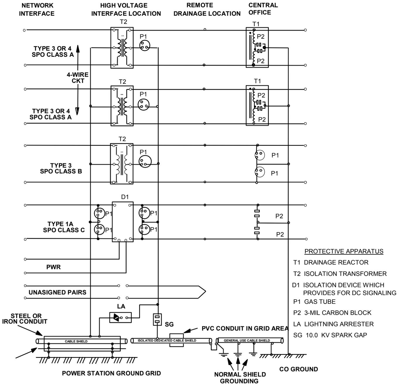
Figure 10 - Isolation System of Protection Using Discrete Components
