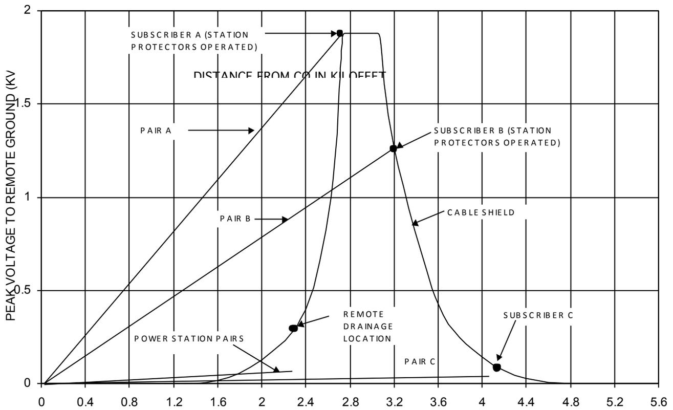
Figure 15 – Voltage Gradient Along General Use Cable
