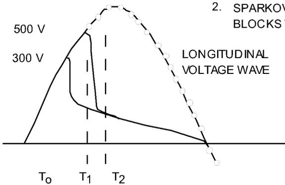
Figure 9 - Unsymmetrical Operation of Protectors
