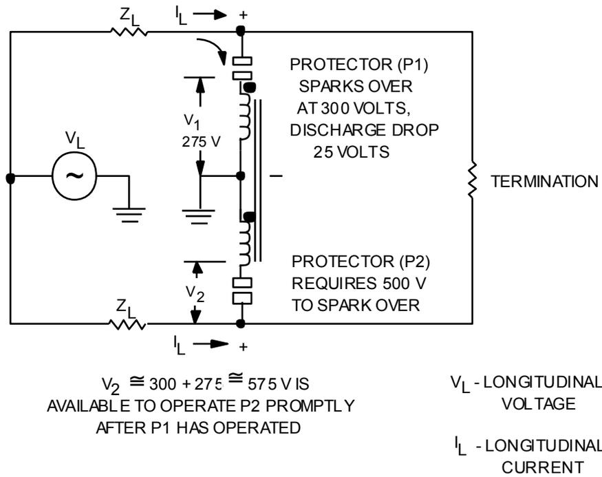
**Figure 8** - Mutual Drainage Reactor - Reduction of Unsymmetrical Protector Operation by Mutual Coupling
