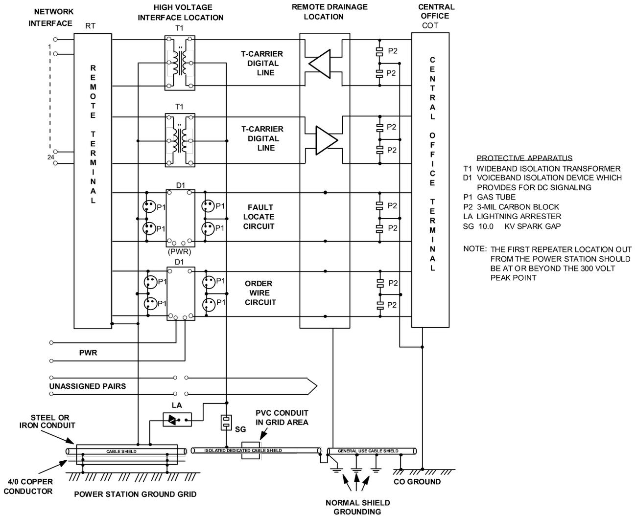
Figure 12 – Isolation System of protection Using Modular Components
