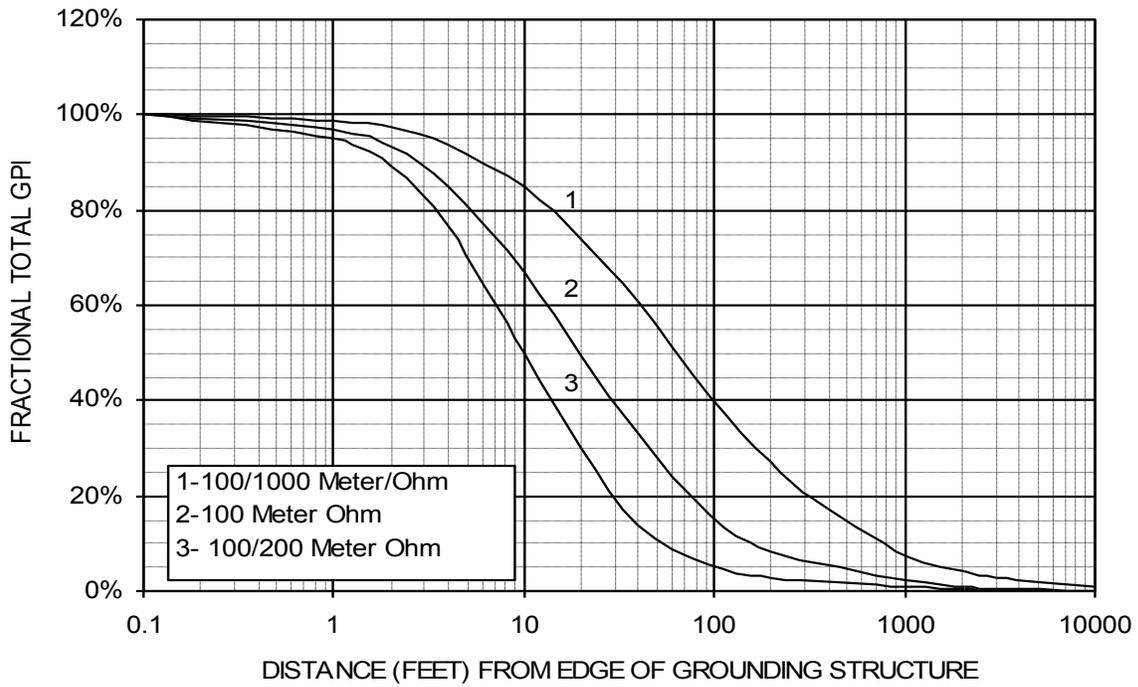
**Figure 5a** – 16,000 Square Feet: Ground Potential Distribution From Edge of Power Station Ground Grid With Respect to Remote Earth
