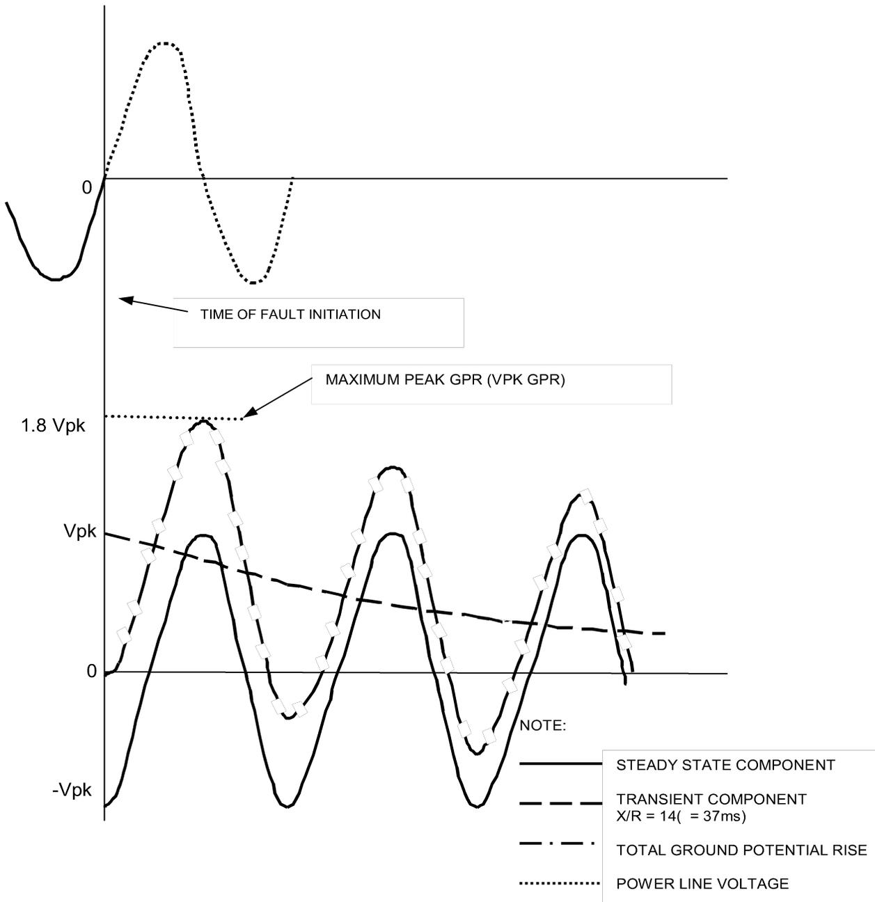
Figure 3 – Ground Potential Rise Composite Waveshape Due to Worst-Case Fault Initiation
