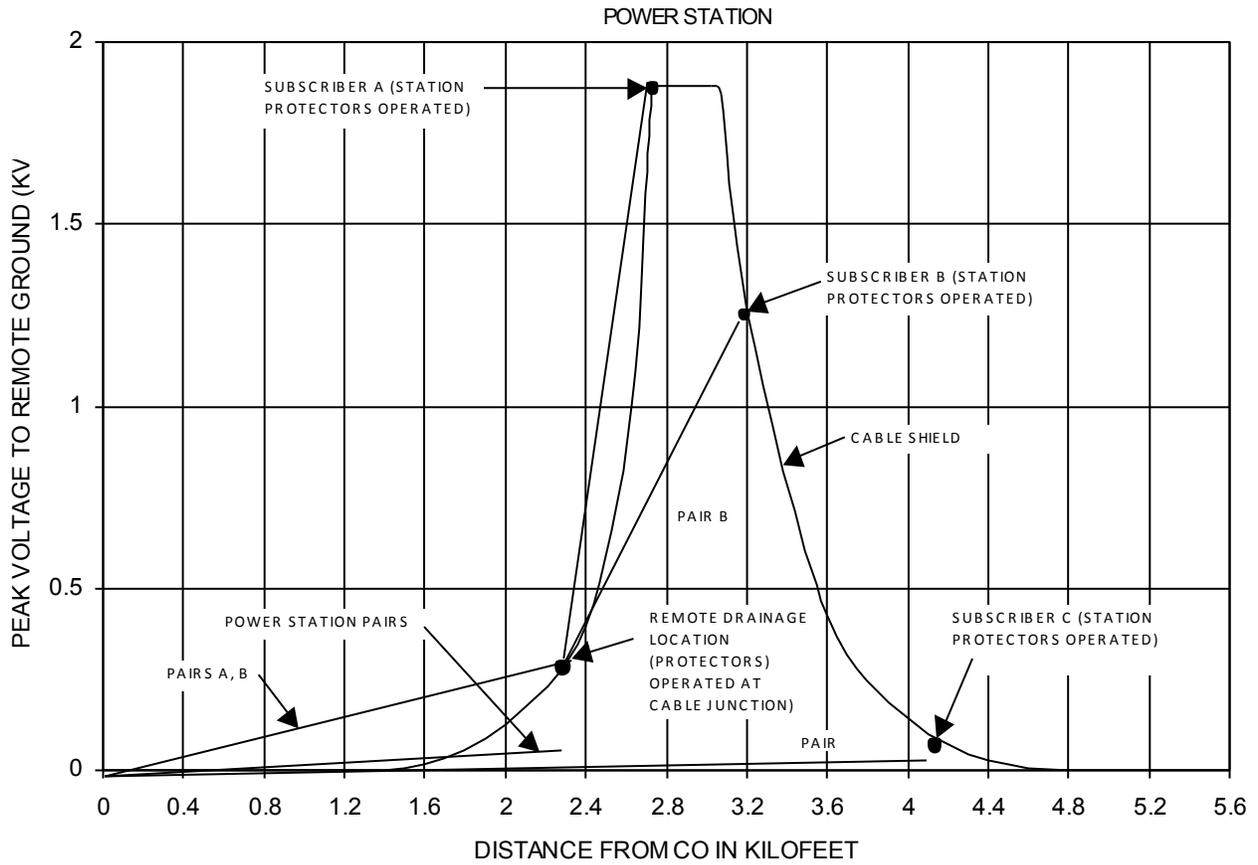
**Figure 16** – Voltage Gradient Along General Use Cable With Full Count Protection Applied At the Remote Drainage Location
