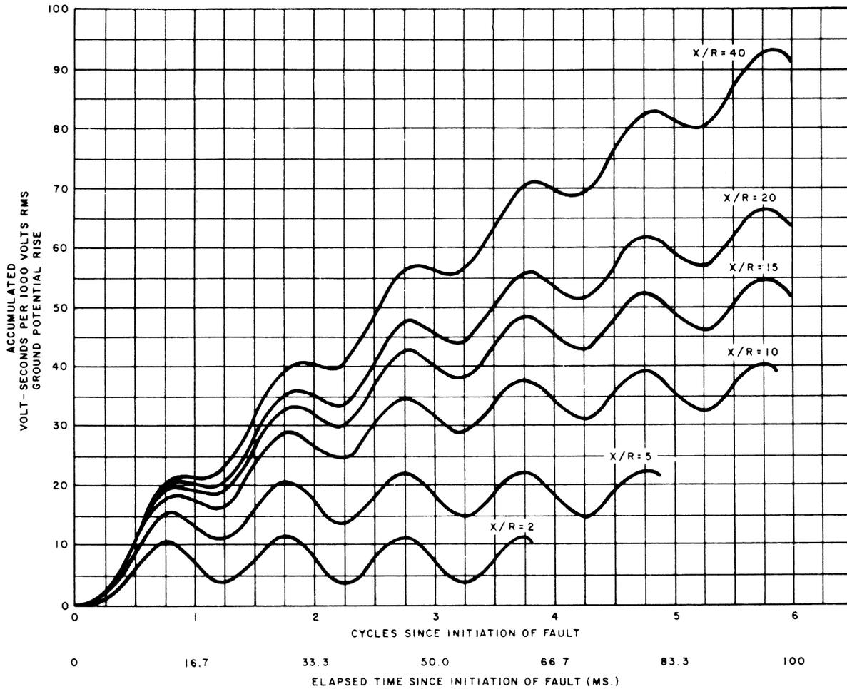
**Figure 5** – Accumulated Volt-Time Area Per 1000 Volts RMS Ground Potential Rise Versus Elapsed Time Since Initiation of Fault For Various X/R Ratios
