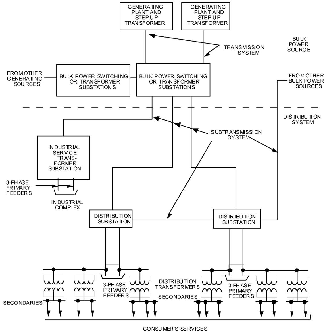
Figure 1 - Simplified Electric Power System Showing Component Pairs
