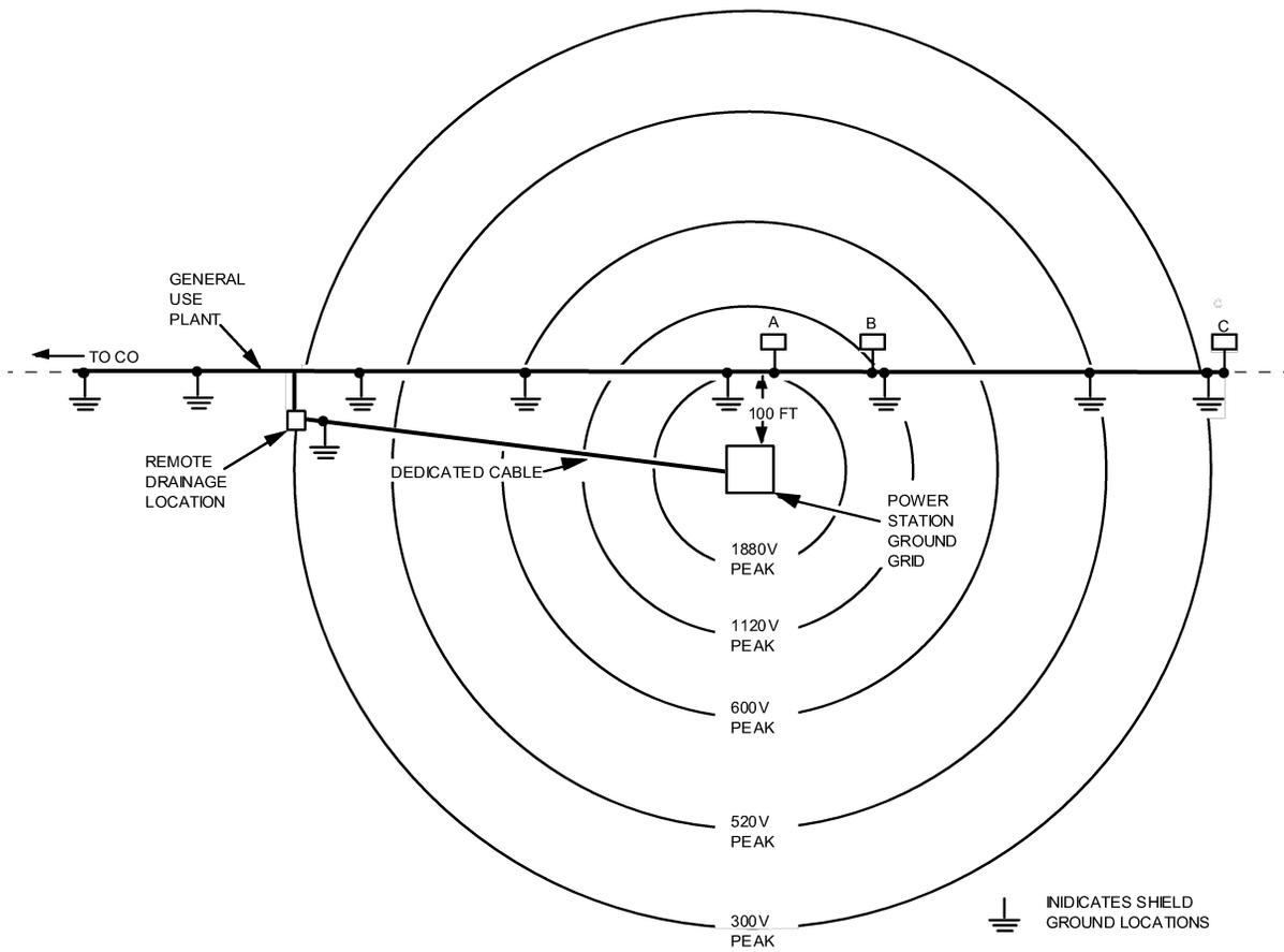
Figure 14 – GPR Voltage Gradient
