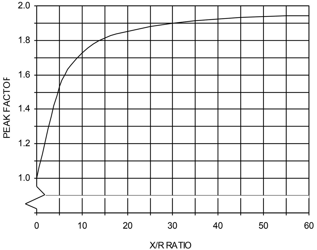
**Figure 4.** – Maximum Peak Factor vs. Power System X/R Ratio For Worst-Case Fault Initiation
