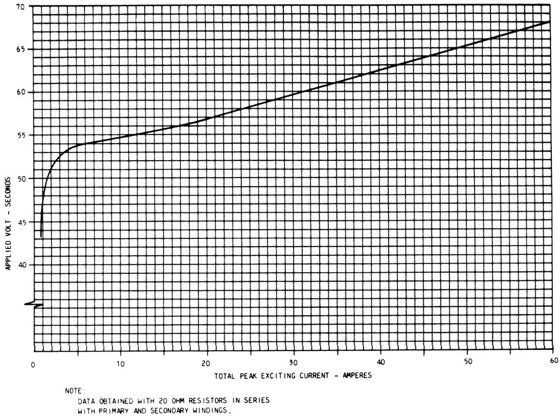
Figure 7 – 52-Volt-Second Rated Neutralizing Transformer Excitation Characteristic
