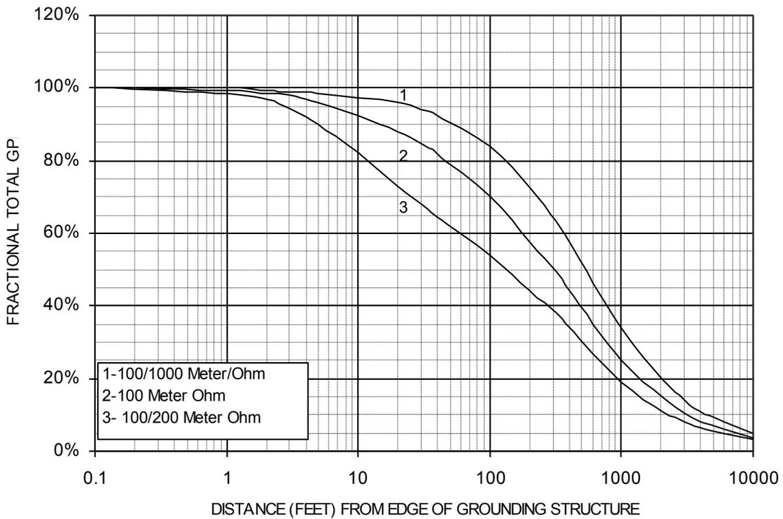
**Figure 5d** – 935,000 Square Feet: Ground Potential Distribution From Edge of Power Station Ground Grid With Respect to Remote Earth
