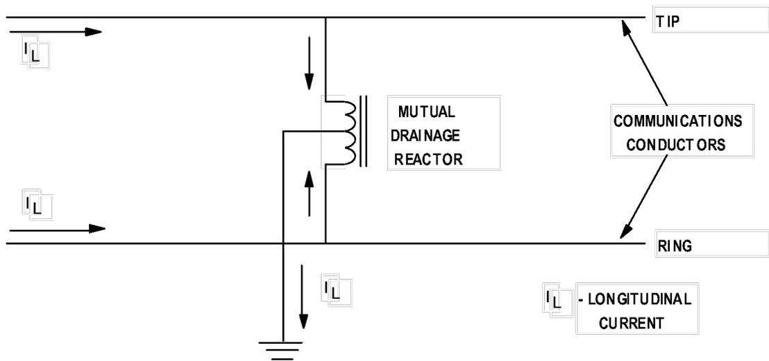
**Figure 7 – Direct Drainage Connection of Mutual Drainage Reacto**
