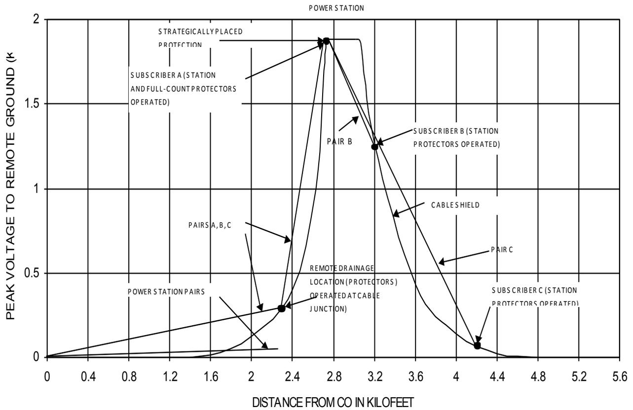
**Figure 17 – Voltage Gradient Along General Use Cable With Full Count Protection Applied At the Remote Drainage Location and Strategically Along Cable Route**
