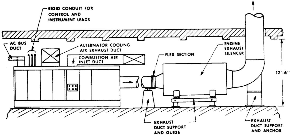
Fig. 7—Typical Megawatt Engine Plant Equipment Area
