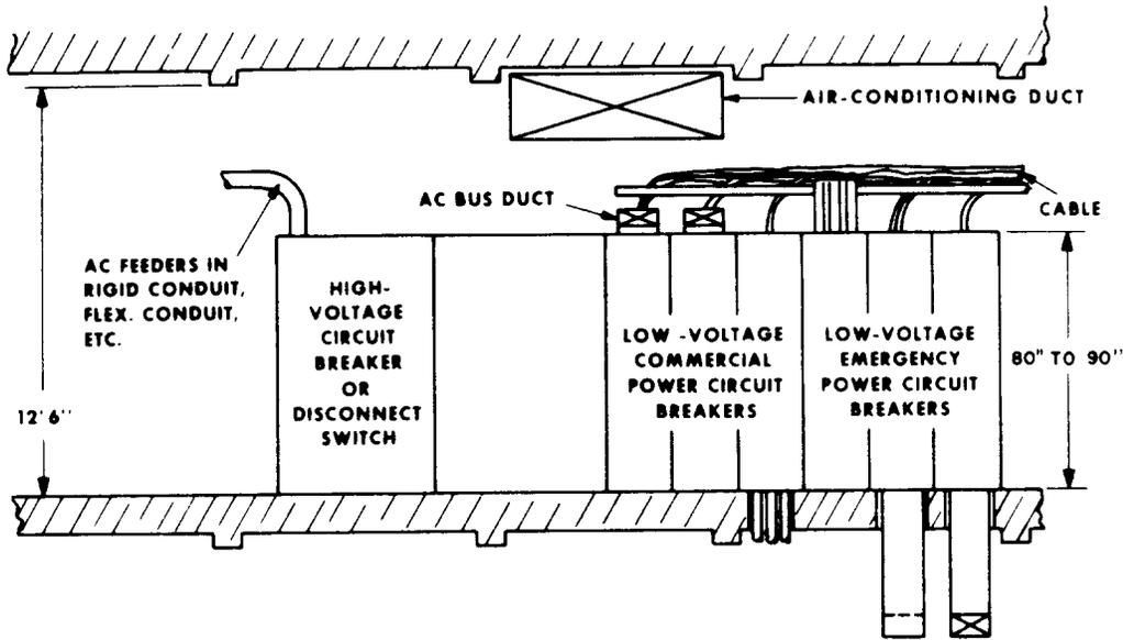
Fig. 6—Typical Building Power Equipment Area
