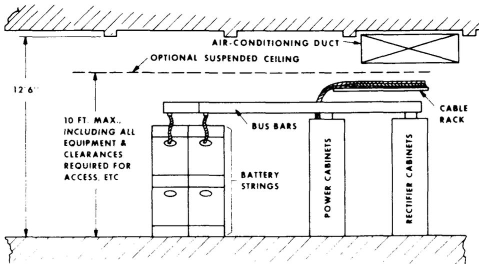
Fig. 5—Typical Telephone Power Equipment Area
