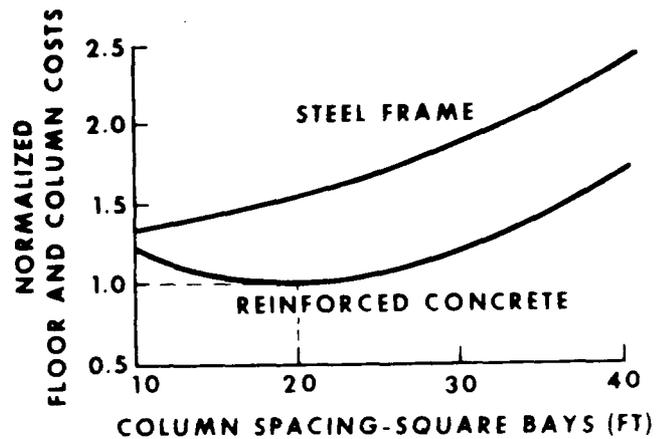
Fig. 1—Building Cost as a Function of Column Spacing
