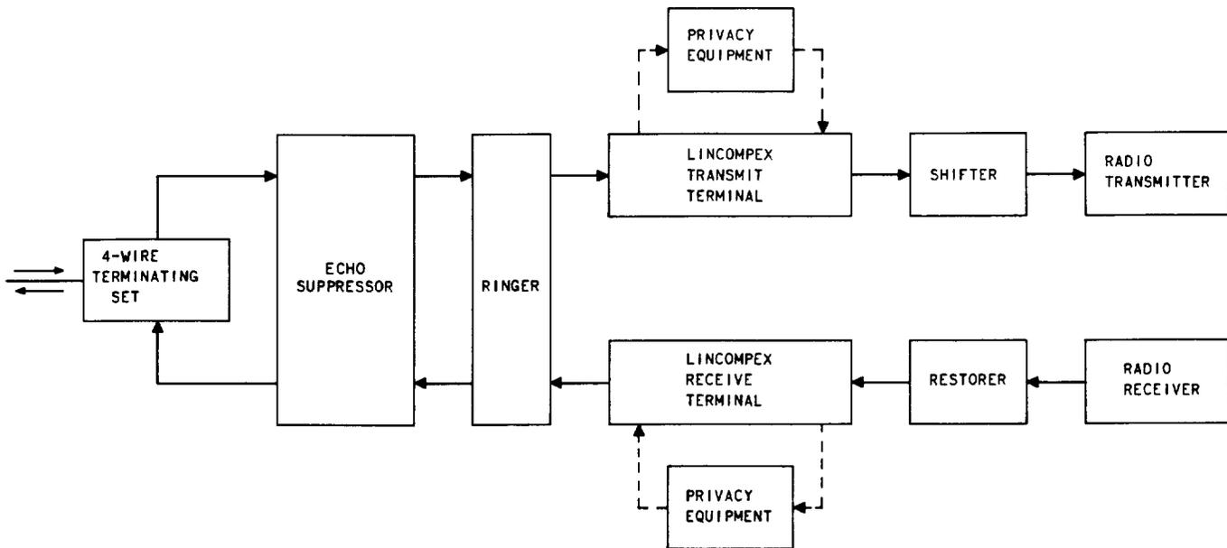
Fig. 3—Radiotelephone Terminal Arrangement
