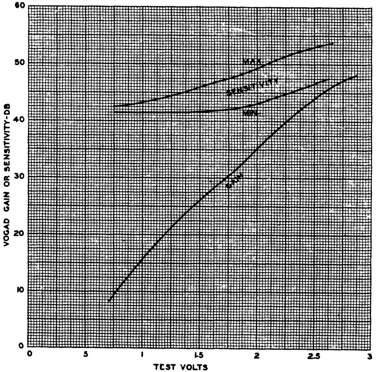
Fig. 2 - Gain and Sensitivity vs. Test Volts
