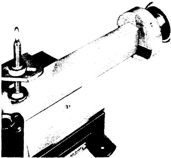
Fig. 5—Rotary File Assembly Inserted in Waveguide End
