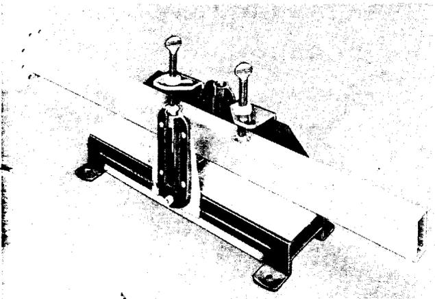
**Fig. 4—Waveguide Section Positioned for Filing**
