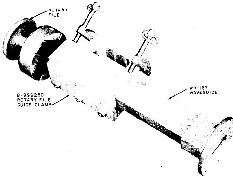
Fig. 7—WR-137 Waveguide Positioned for Filing
