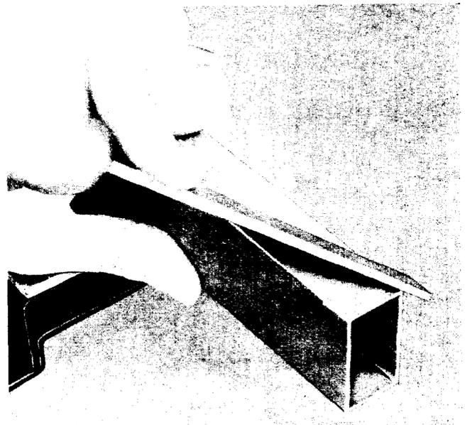
Fig. 9—Rounding Outside Corners of Waveguide
