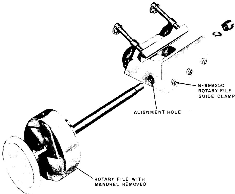
Fig. 6—Preparation for Filing WR-137 or WR-90 Waveguide
