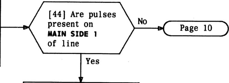
[45] See DANGER 1. At RT, perform Bridged Error Test [DLP-577] on MAIN SIDE 2. Connect patch cord as shown in FIG. 2
