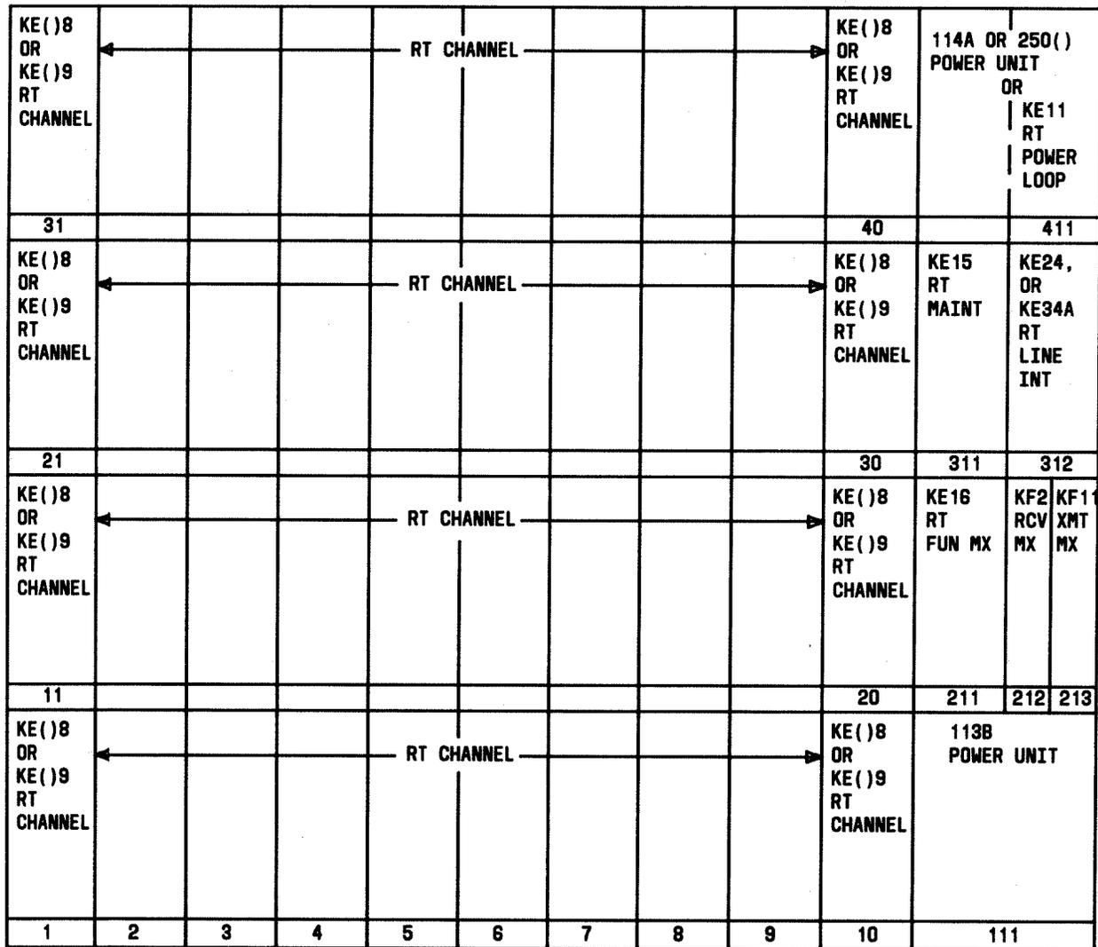
FIG. 1 - RT Frame (Lower System) - Circuit Pack Locations Shown
