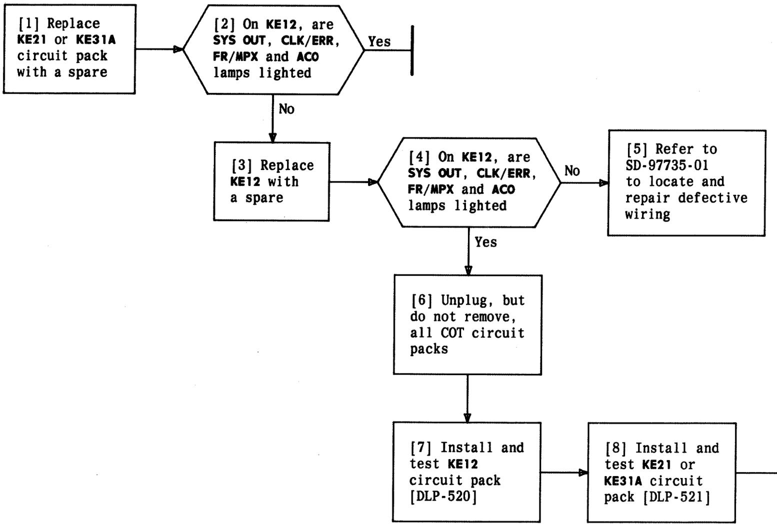
**CLEAR KE12 LAMP TROUBLE WHEN INSTALLING
