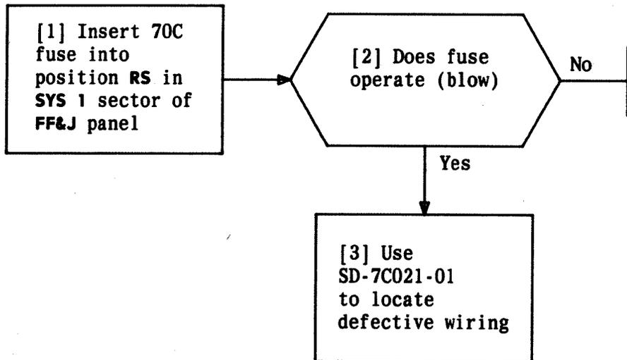
**INSERT 70C FUSE IN POSITION RS LOCATED IN SYS 1 SECTOR OF FF&J PANEL**
