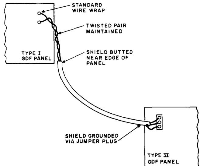
Fig. 3—Cross-Connection Between Type I and Type II Group Distribution Frames
