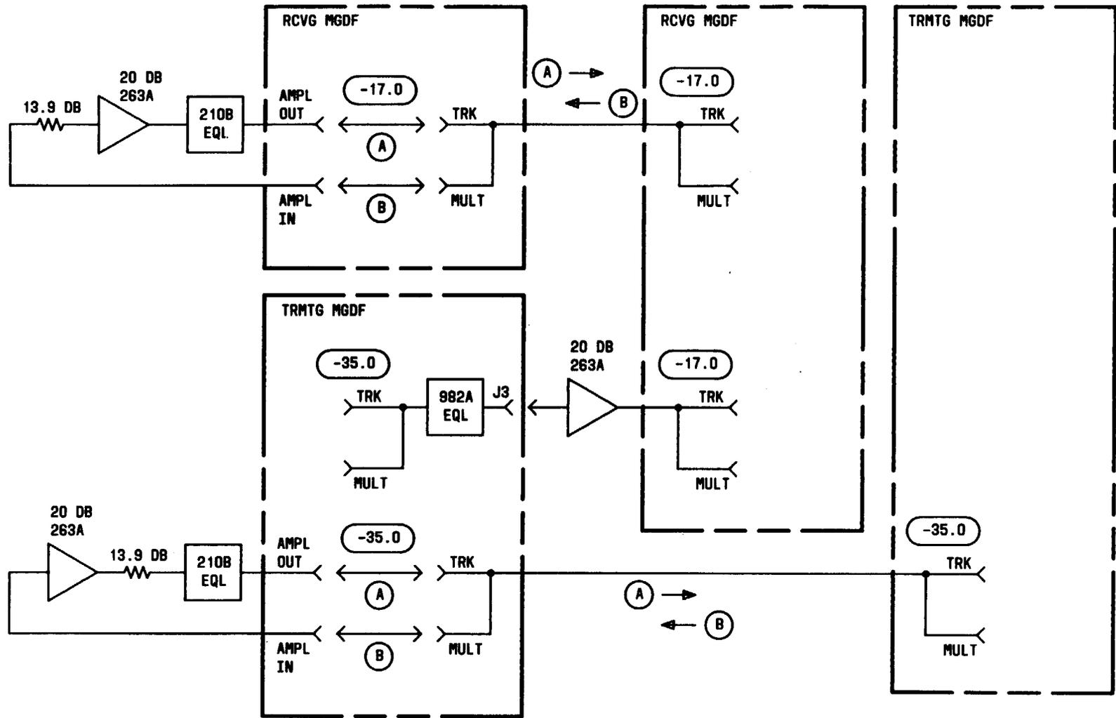
Fig. 12—Trunks Between Mastergroup Distribution Frames
