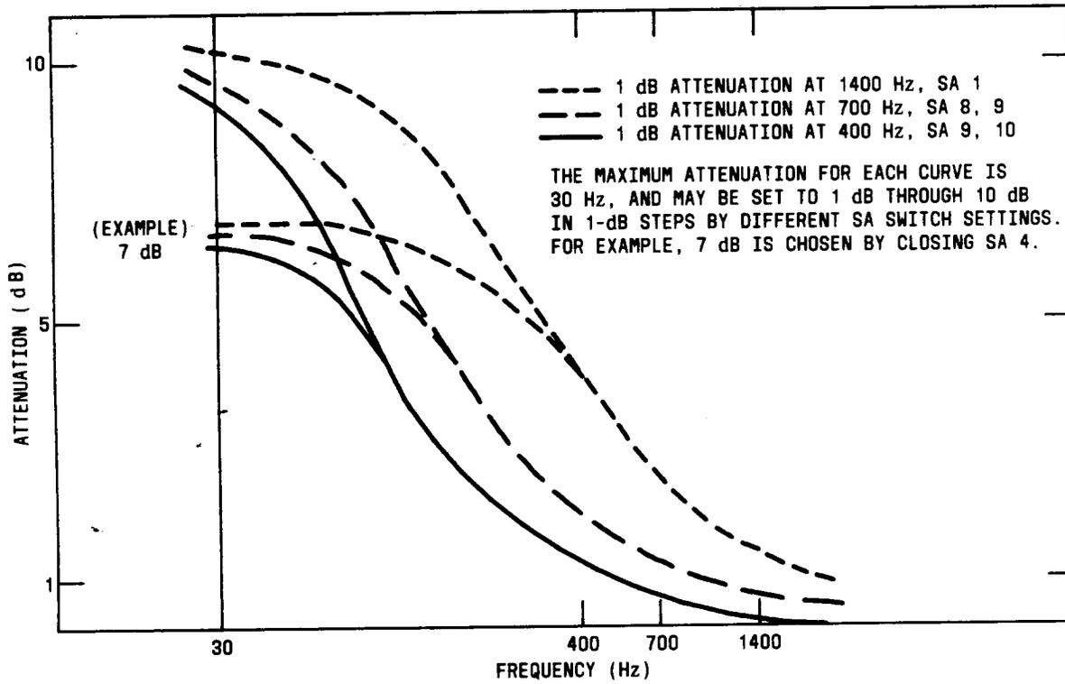
Fig. 7—QVF52B and E Low-Frequency Equalization
