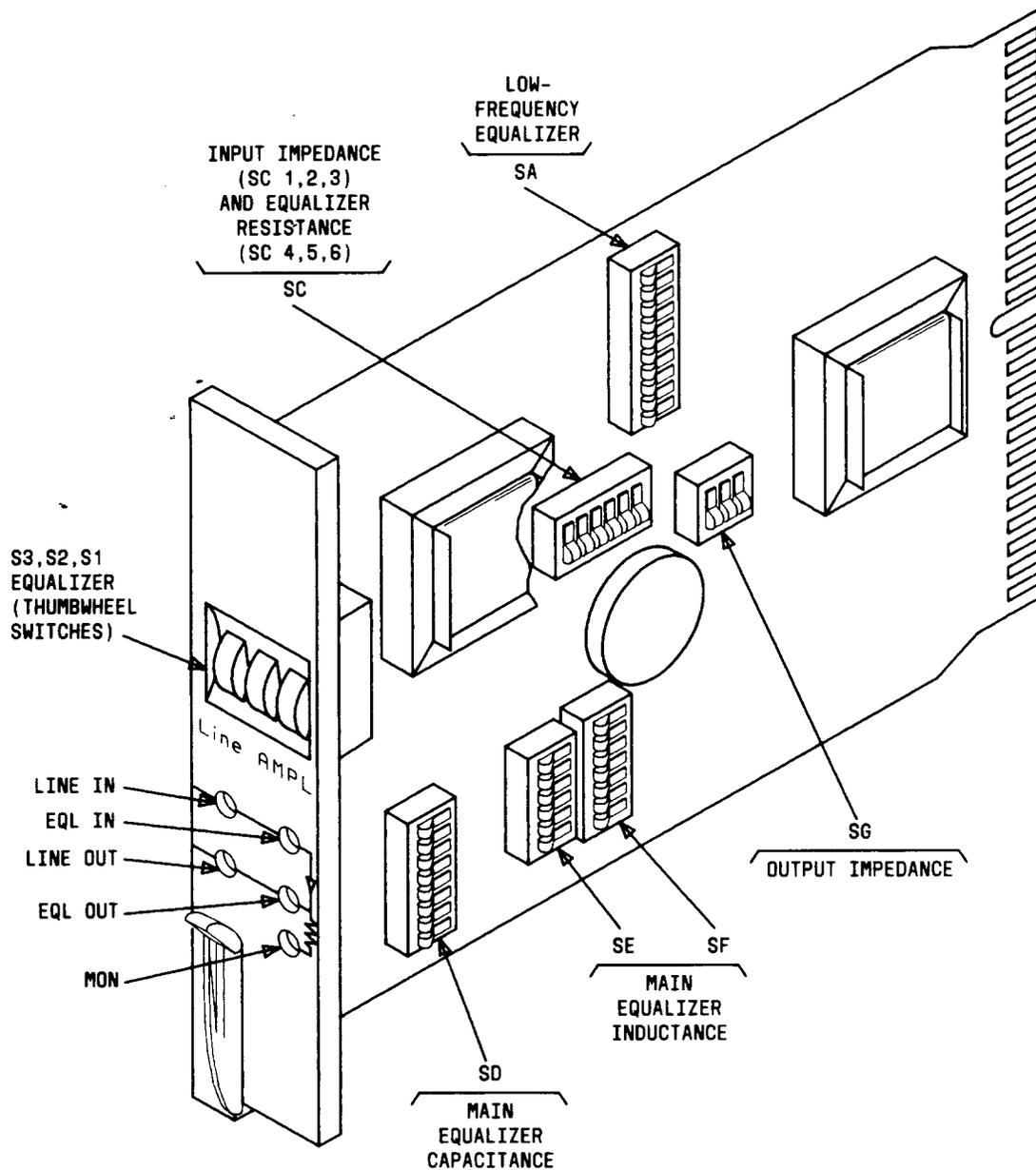
Fig. 3—QVF52D Physical Layout
