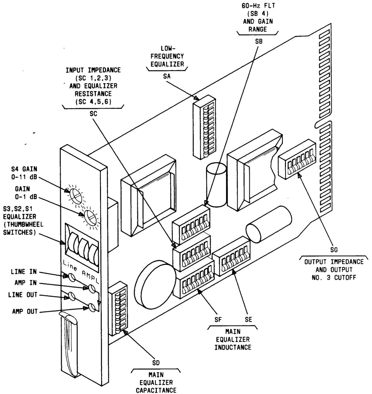
Fig. 2—QVF52E Physical Layout
