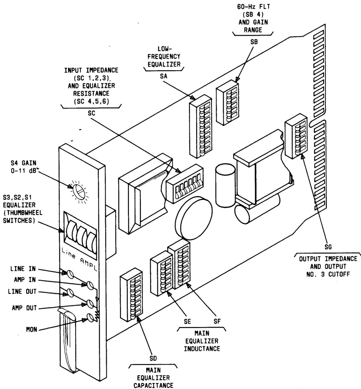
Fig. 1—QVF52B Physical Layout
