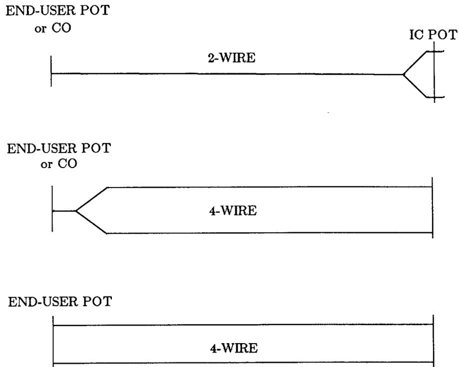
**Figure 9.** Typical VG7 Channel Configurations
