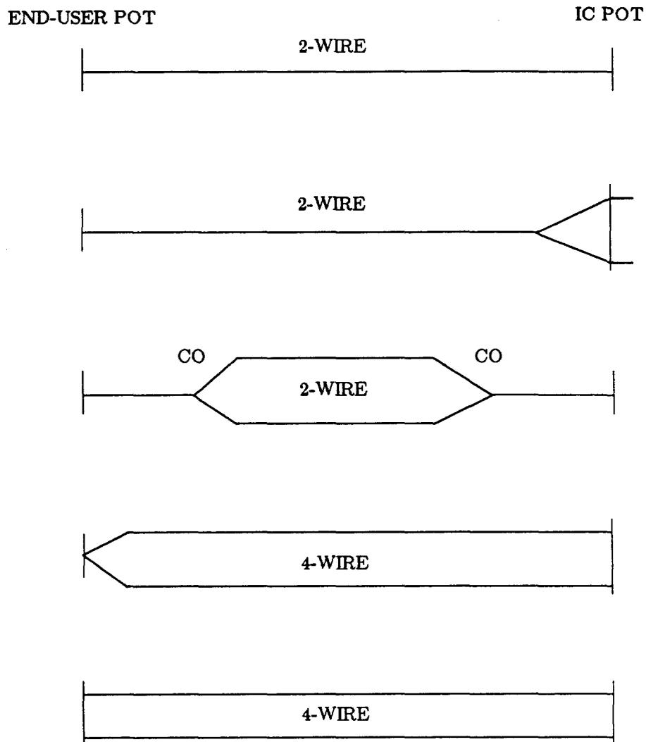
**Figure 7.** Typical VG5 Channel Configurations
