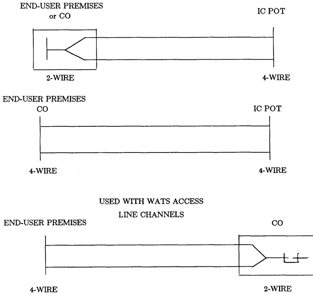
Figure 2. Typical Effective 4-Wire Channel Configurations
