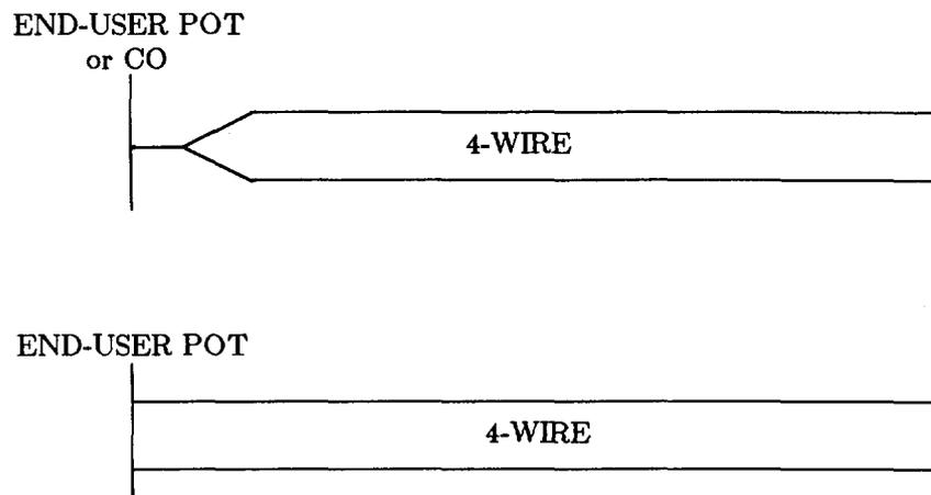
**Figure 10.** Typical VG8 Channel Configurations
