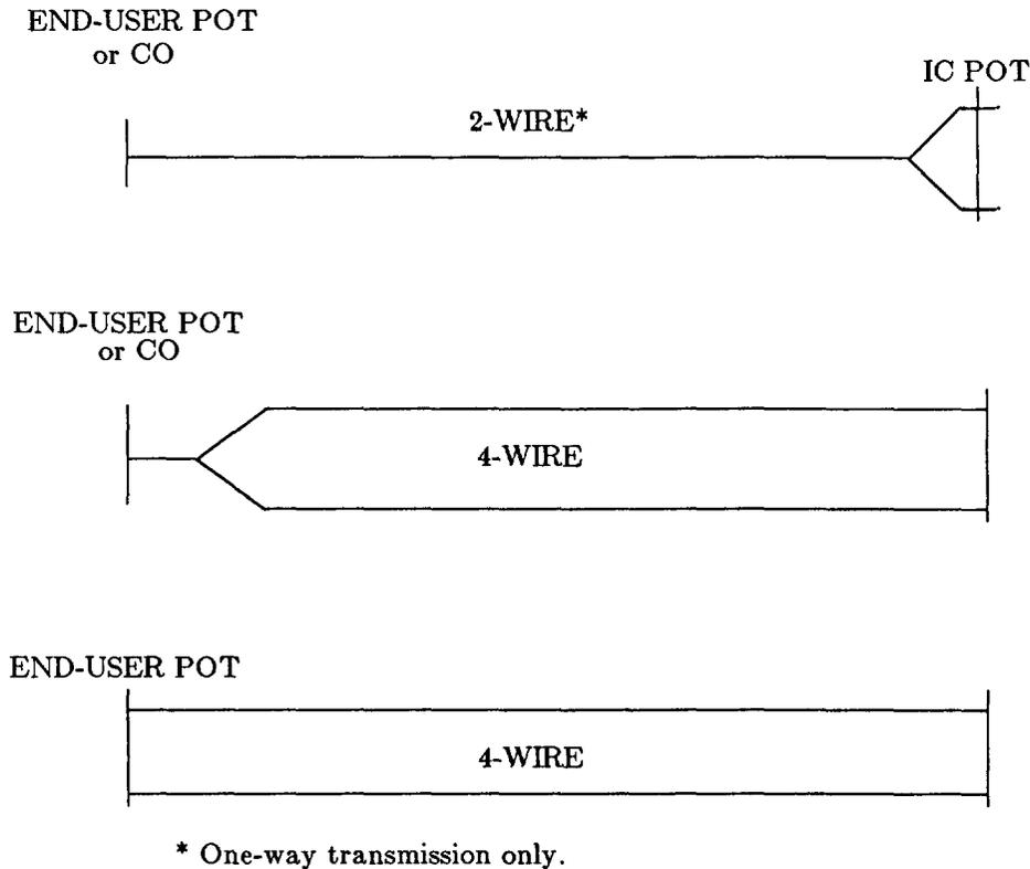
**Figure 14.** Typical VG12 Channel Configurations
