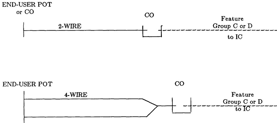
Figure 15. Typical WATS Access Line Configurations
