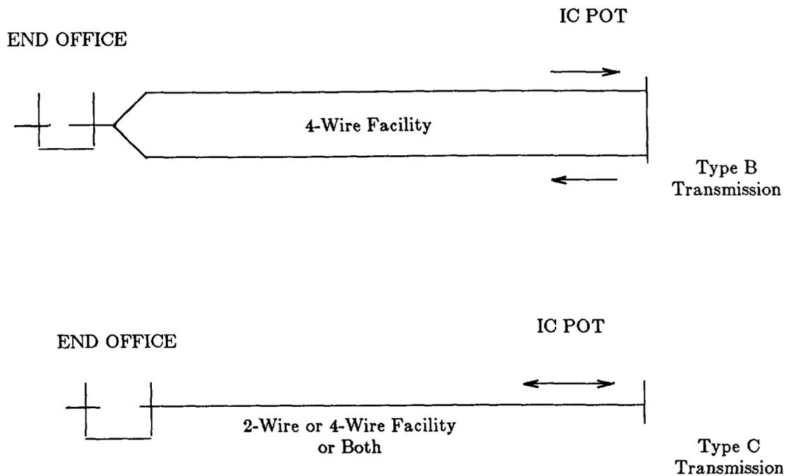
**Figure 16.** Typical Feature Group A Configurations
