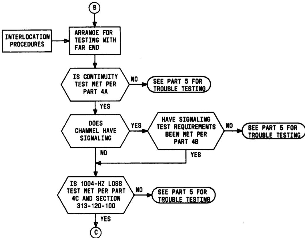
Flowchart 1—Required Preservice and Trouble Tests (Sheet 3 of 7)
