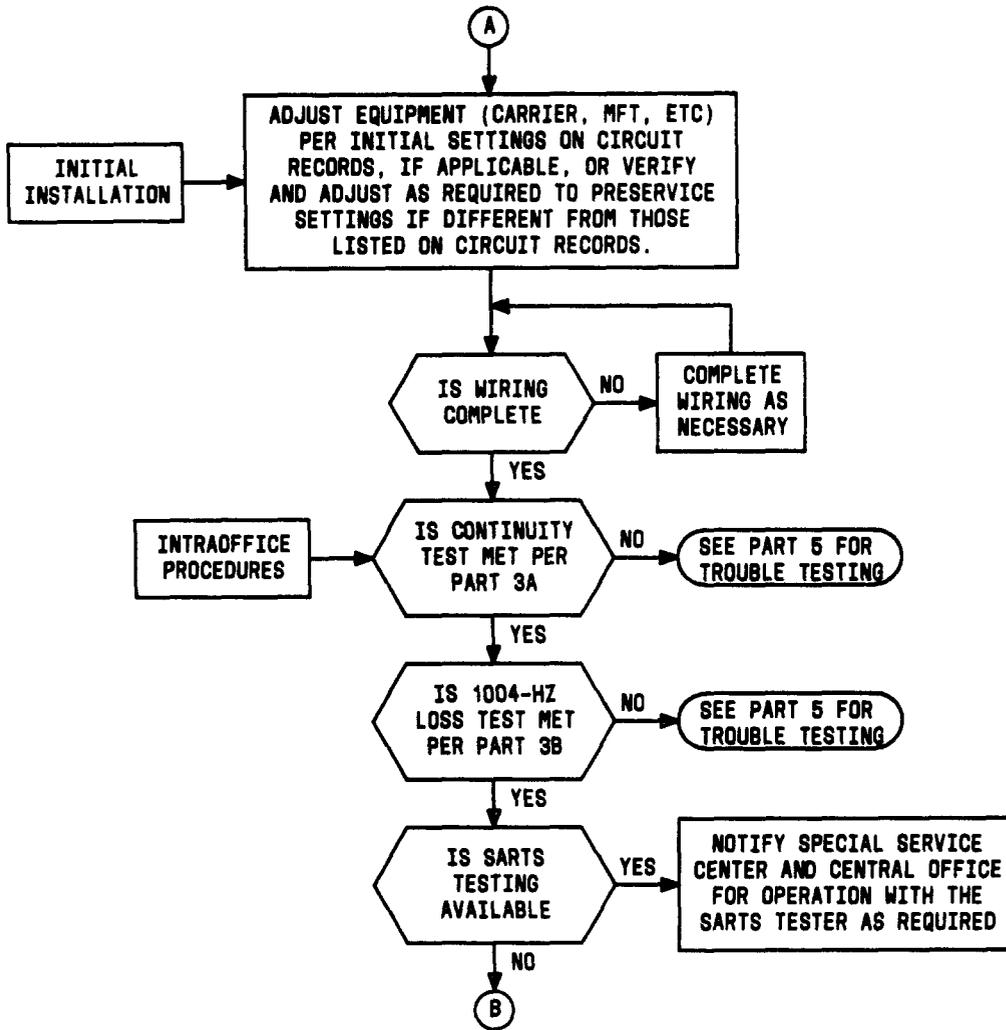
Flowchart 1—Required Preservice and Trouble Tests (Sheet 2 of 7)
