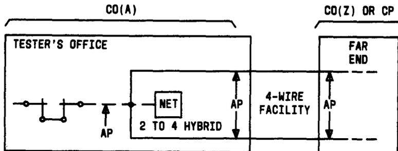
Fig. 1—2-Wire to 4-Wire Conversion at Tester's Office
