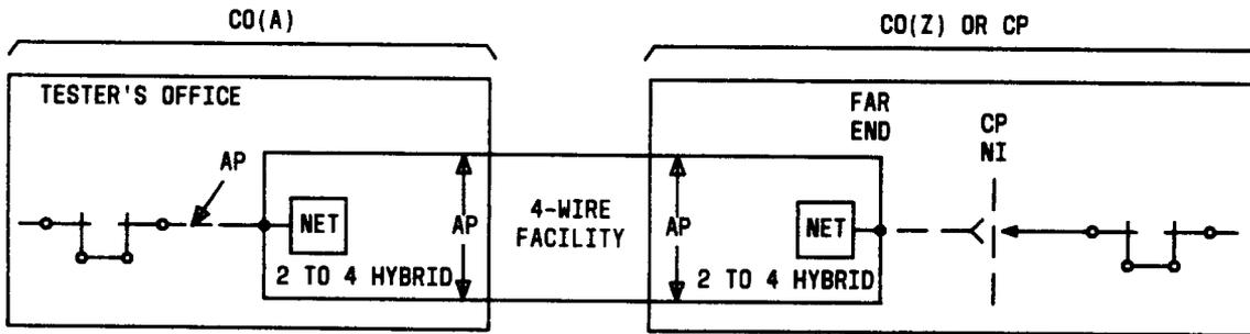
Fig. 3—2-Wire to 4-Wire Conversion at Both Ends
