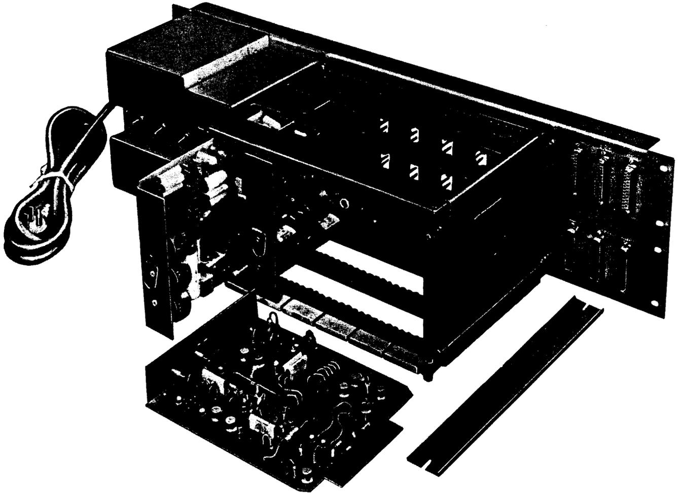
Fig. 7—820E Data Auxiliary Set—Front View 1—108 Data Set and Interface Card Installed in Set 1—109 Data Set Displayed in Front
