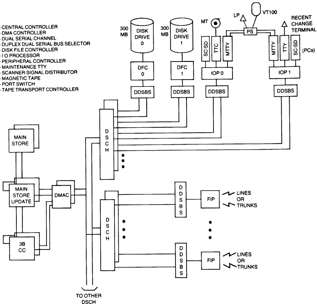
Fig. 1—Packet Switch Hardware Configuration (2.04)
