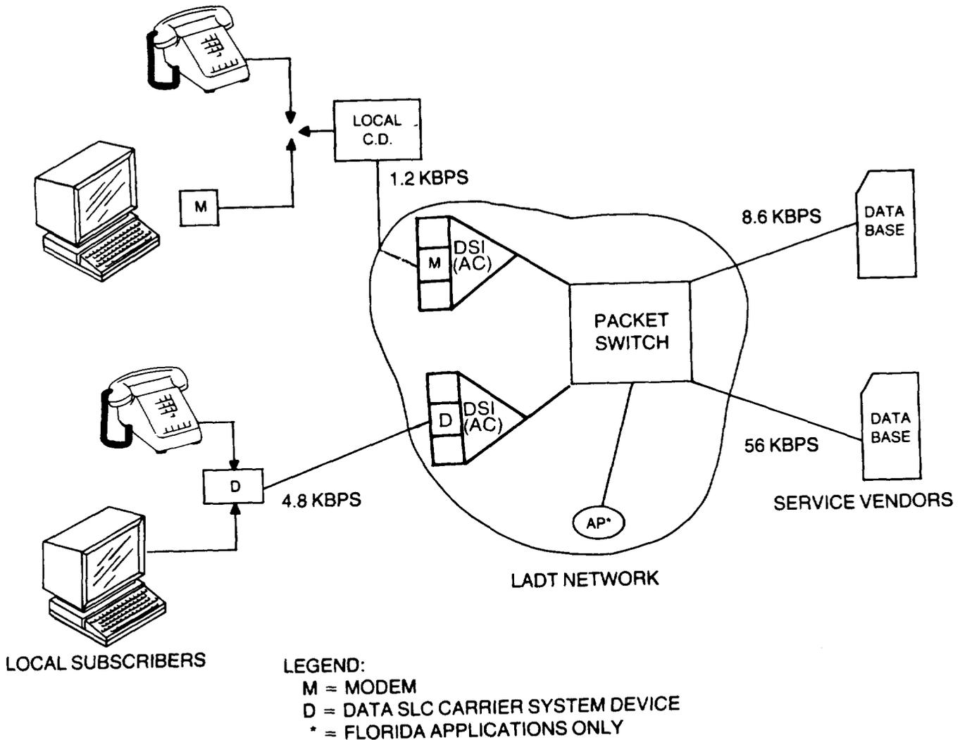
Fig. 1—LADT Basic Network Architecture (2.04)
