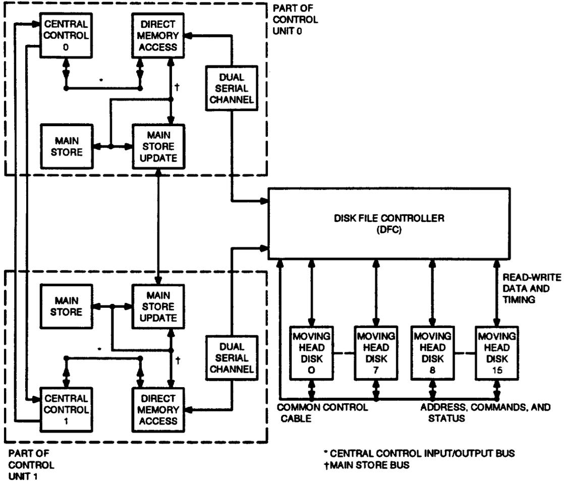
**Figure 3. Control Unit—Moving Head Disk Drive Interface**
