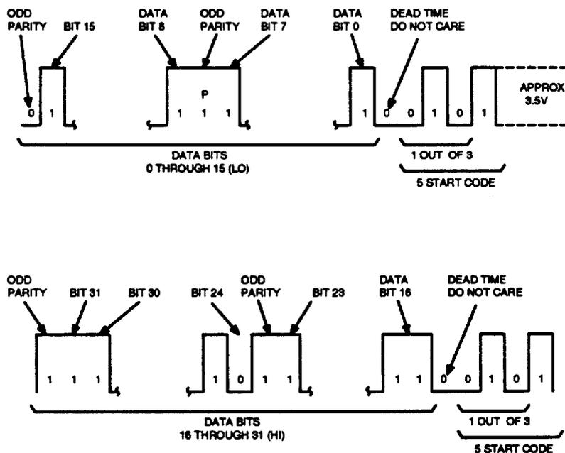
Figure 11. Disk File Controller—Direct Memory Access Message Format
