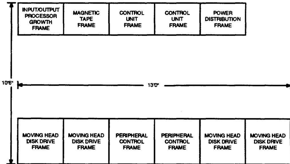
**Figure 1. Typical Computer Floor Plan**
