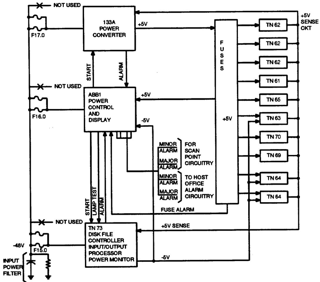
Figure 12. Disk File Controller Unit Power and Alarm Circuit (Generic 1)
