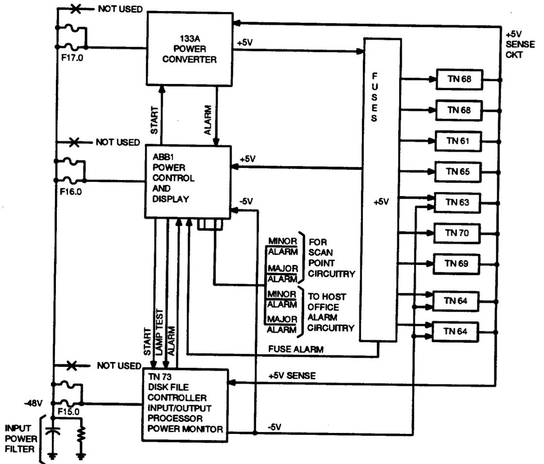
Figure 13. Disk File Controller Unit Power and Alarm Circuit (Generic 2)
