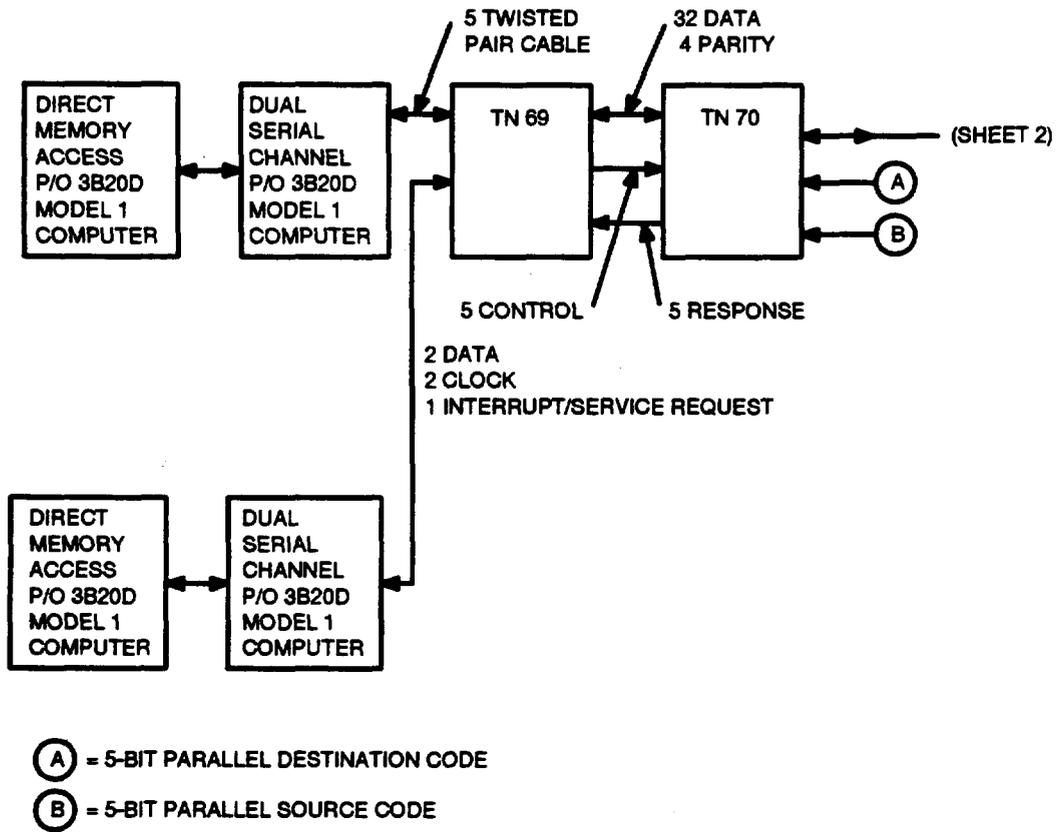
Figure 9. Disk File Controller Unit Block Diagram (Generic 2) (Sheet 1 of 2)
