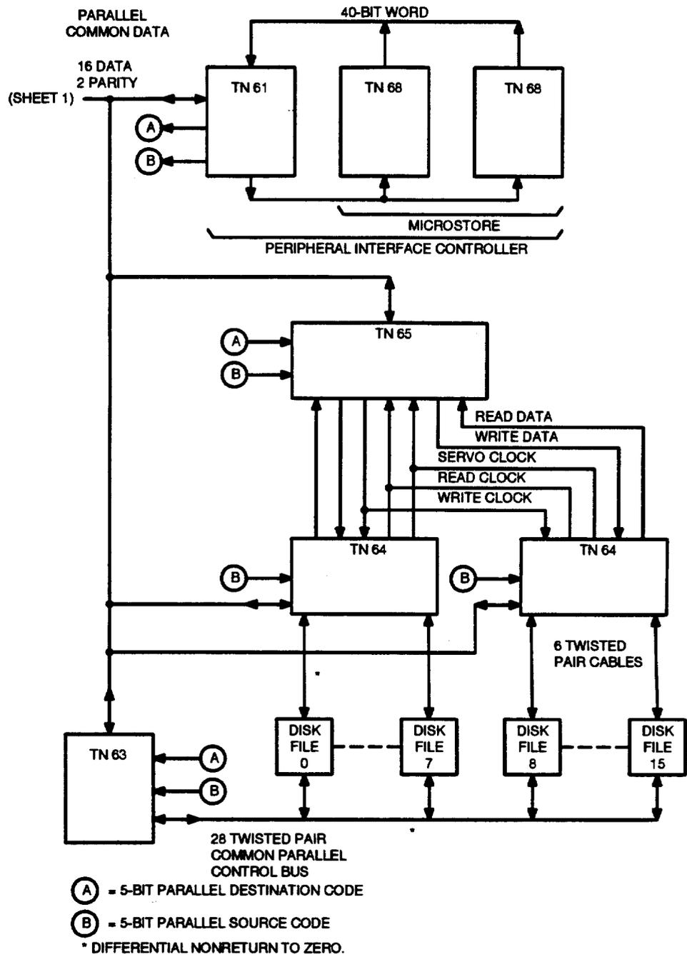
Figure 9. Disk File Controller Unit Block Diagram (Generic 2) (Sheet 2 of 2)
