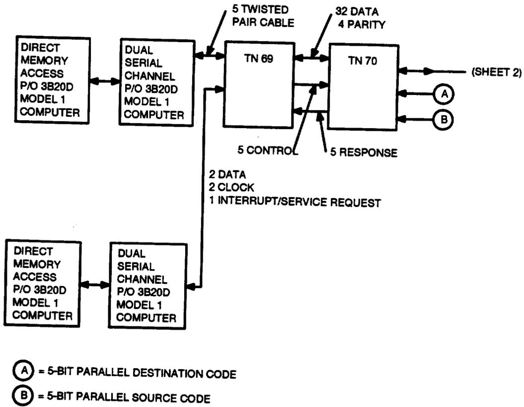
Figure 10. Disk File Controller Unit Block Diagram (Generic 3) (Sheet 1 of 2)
