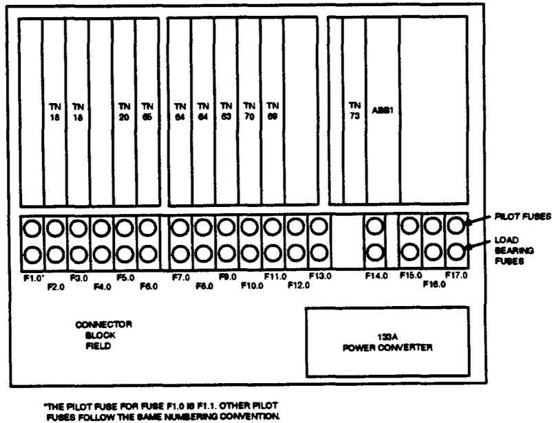
Figure 7. Typical Disk File Controller Layout (Generic 3)
