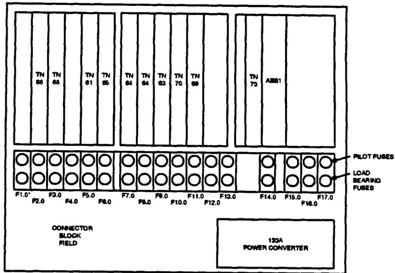
THE PILOT FUSE FOR FUSE F1. IS F1.1. OTHER PILOT FUSES FOLLOW THE SAME NUMBERING CONVENTION.
