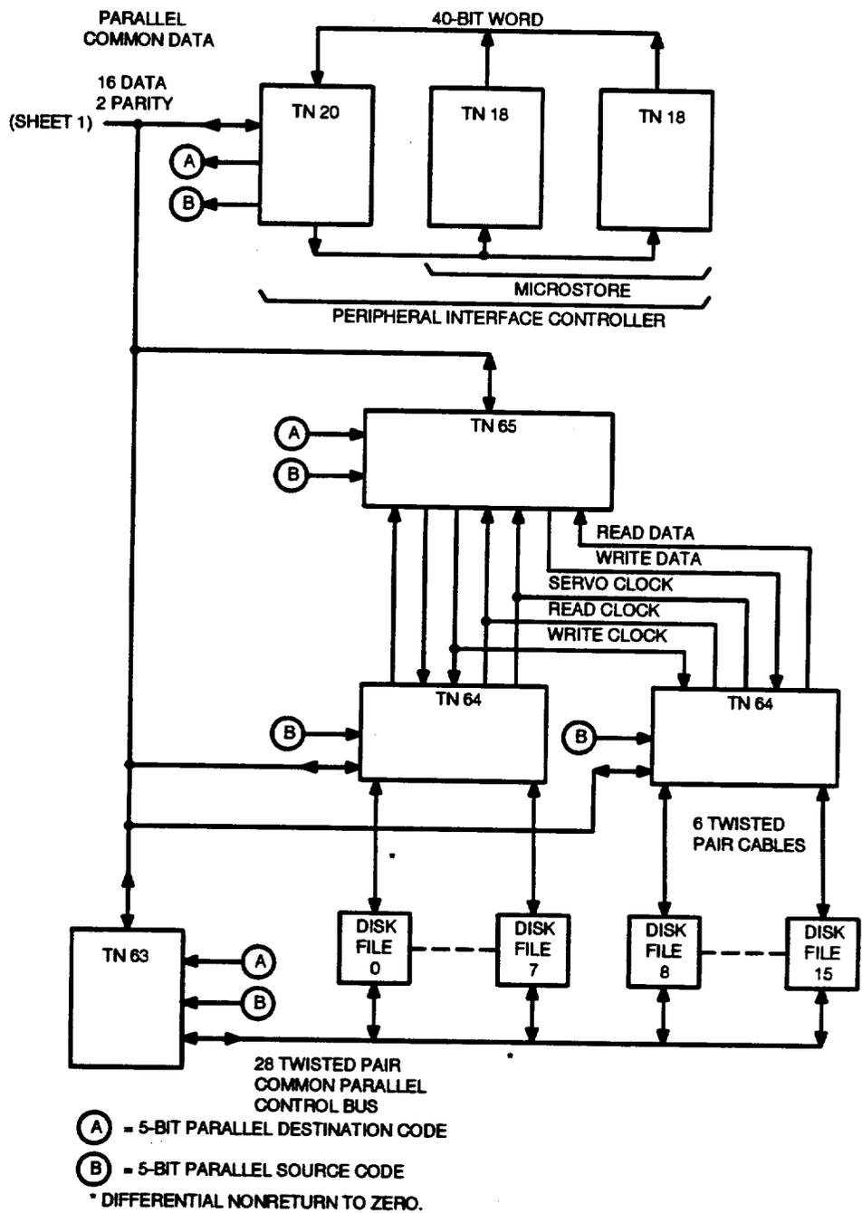
Figure 10. Disk File Controller Unit Block Diagram (Generic 3) (Sheet 2 of 2)
