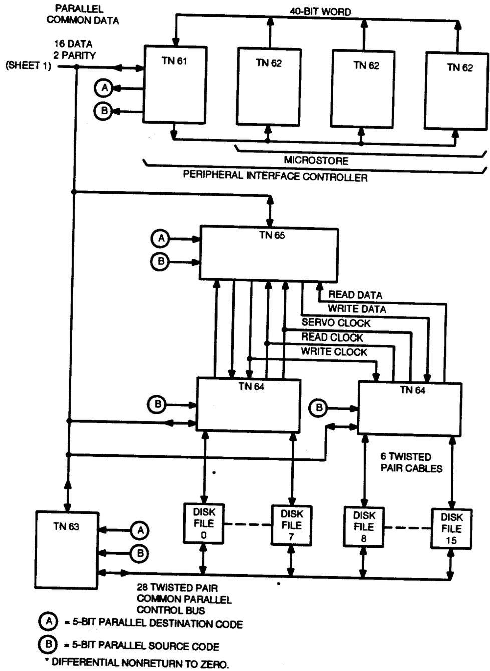
Figure 8. Disk File Controller Unit Block Diagram (Generic 1) (Sheet 2 of 2)
