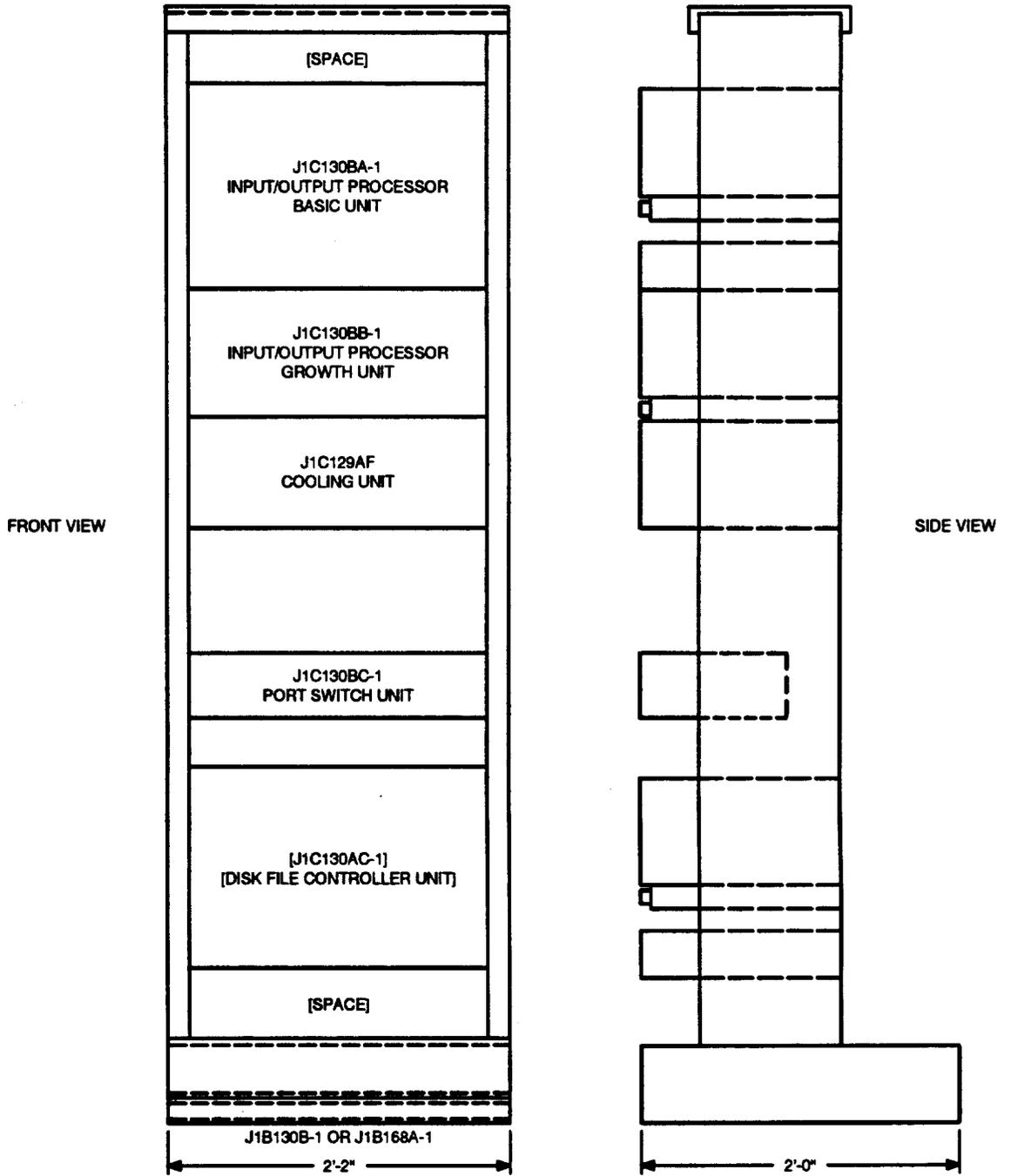
Figure 2. Typical Peripheral Control Frame With Disk File Controller
