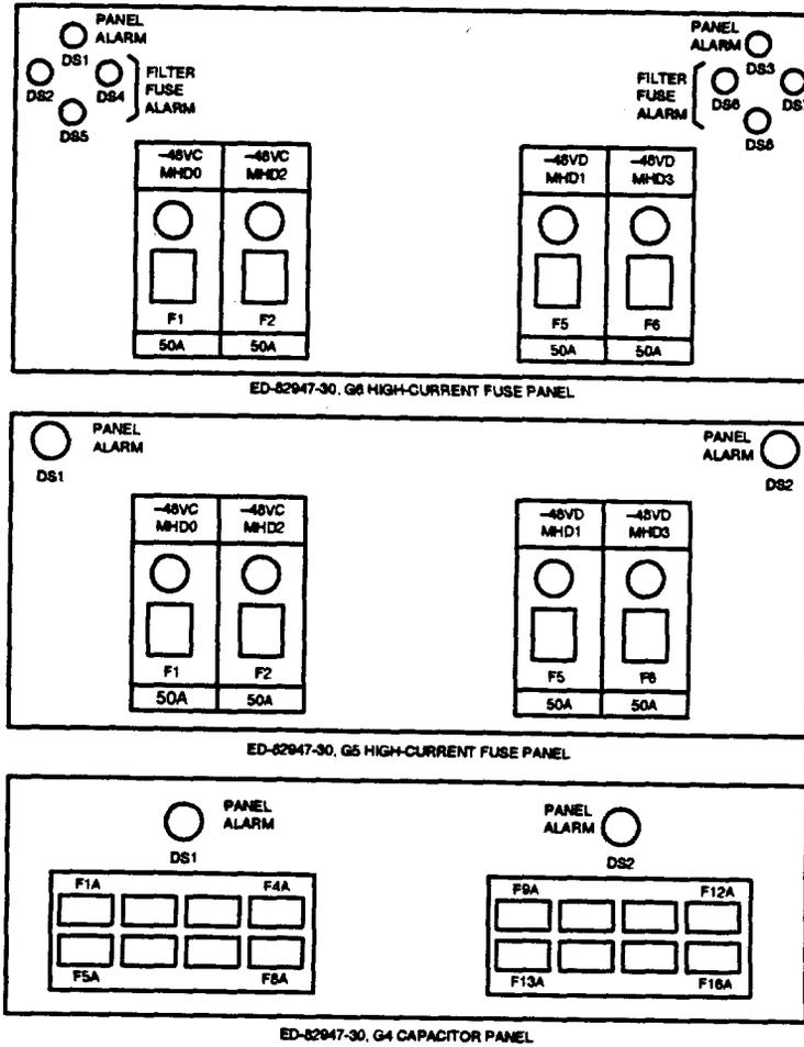
Figure 21. High-Current Fuse Panels
