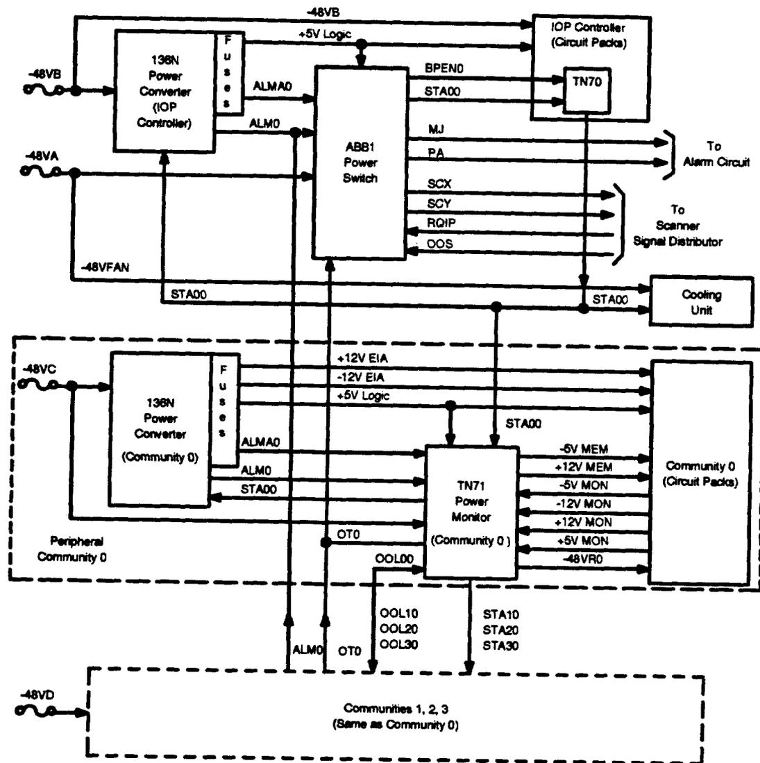
Figure 25. Input/Output Processor Power Block Diagram
