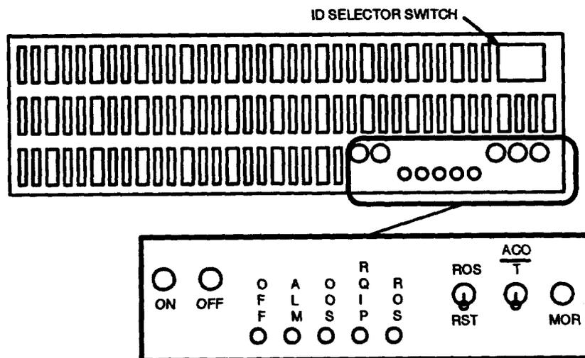
**Figure 19. SCSI Disk Unit Package**
