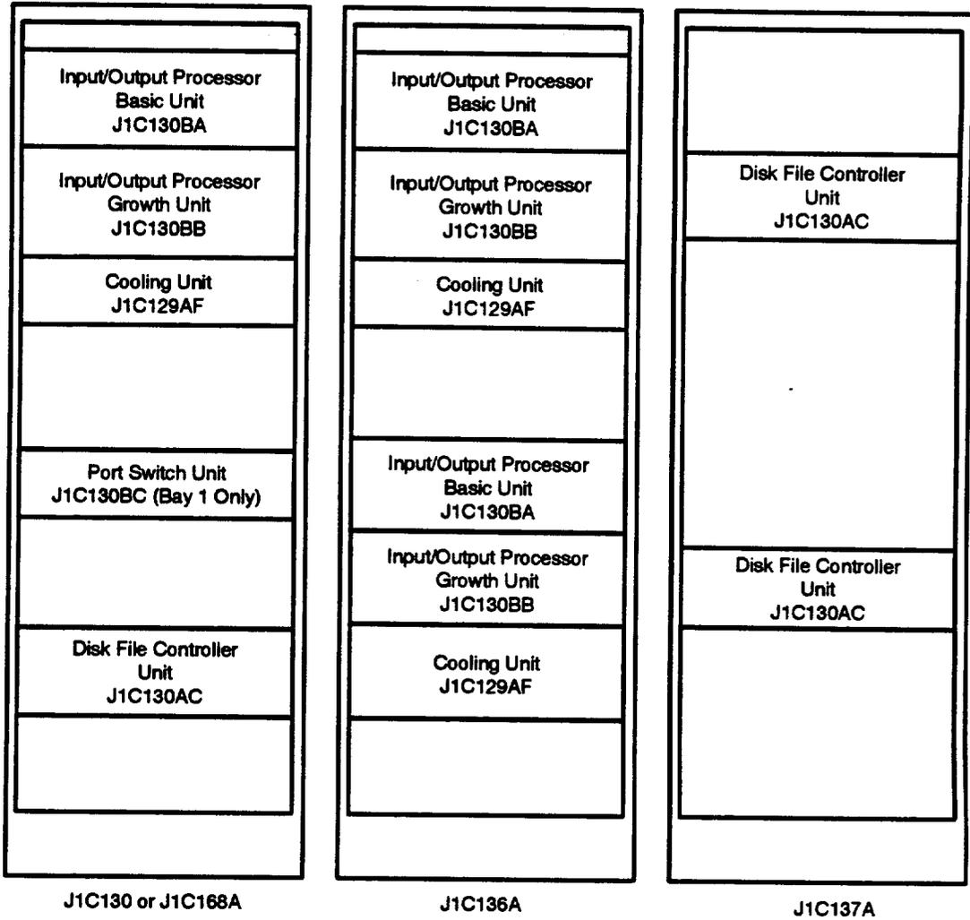
Figure 2. Peripheral Control Frames
