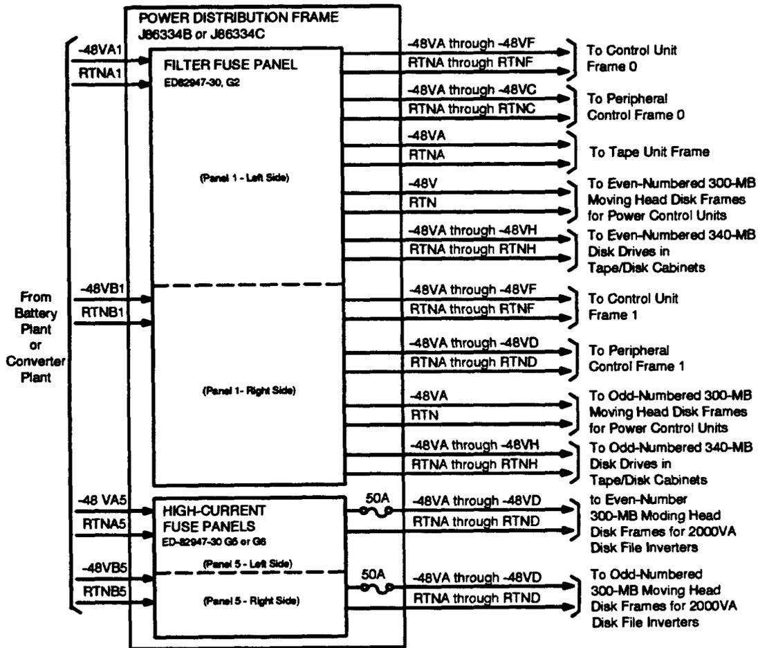
Figure 22. Power Distribution Frame Block Diagram
