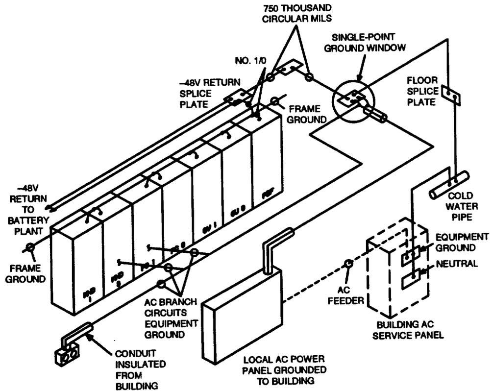
Figure 8. Typical Overhead Single-Point Ground System
