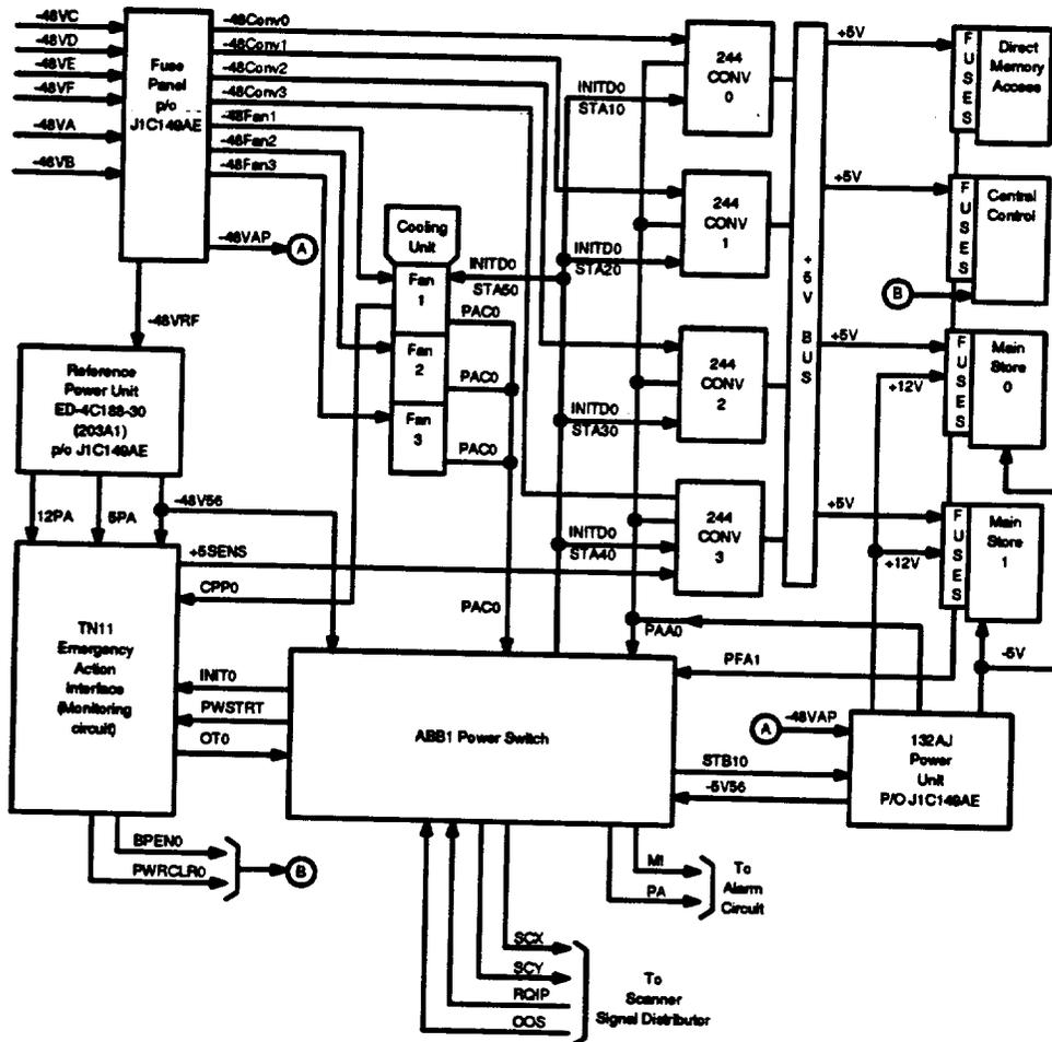
Figure 24. Control Unit Power Block Diagram
