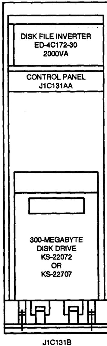
Figure 3. Moving Head Disk Frame
