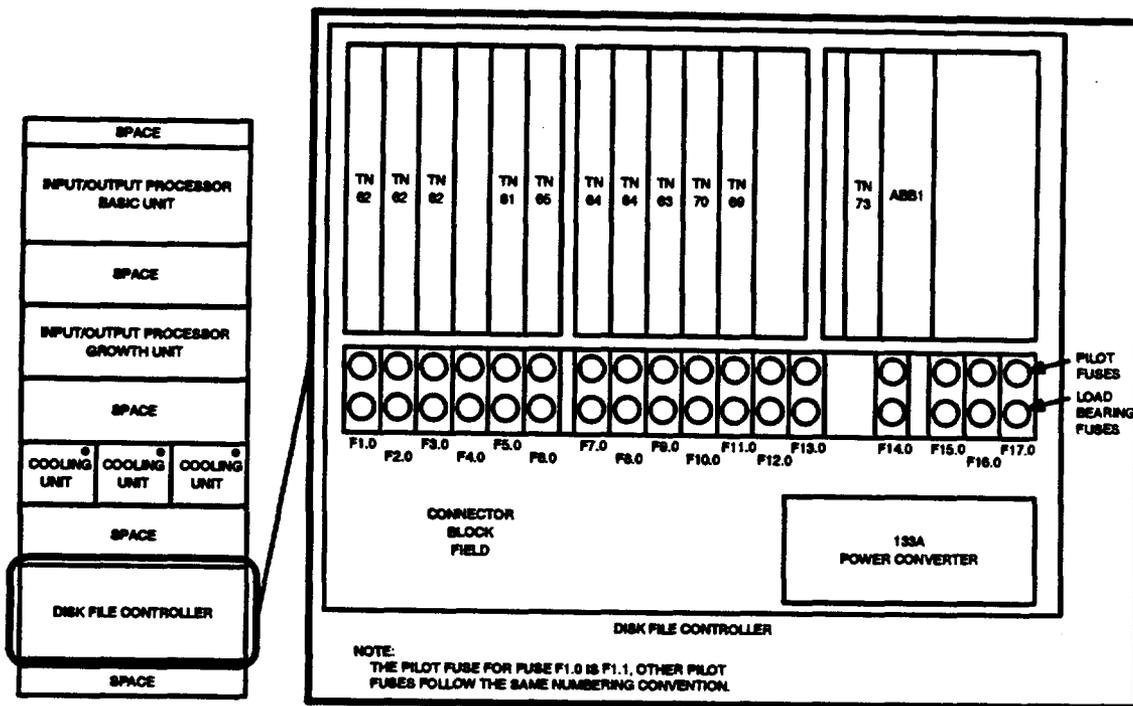
**Figure 2. Peripheral Control Frame—SMD—Disk File Controller**
