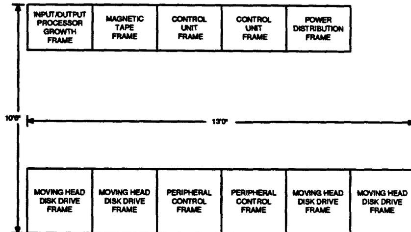
**Figure 7. Typical 3B20D Model 1 Computer Floor Plan**
