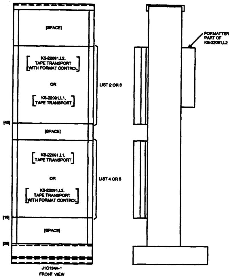
**Figure 5. Magnetic Tape Frame**
