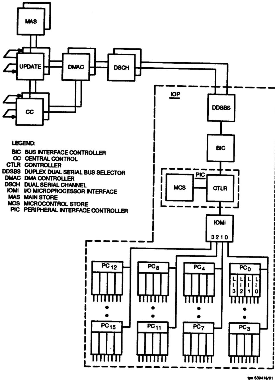
Figure 13. Input/Output Processor Block Diagram
