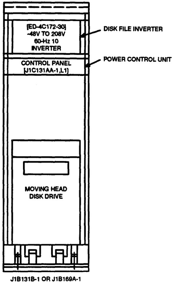
Figure 4. Moving Head Disk Frame (80/300 Mbyte)
