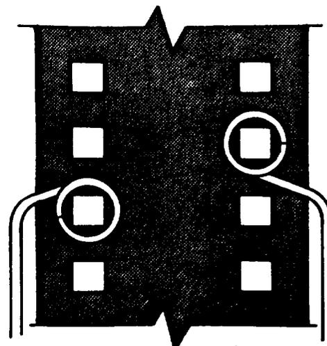
Figure II-7—Typical Terminal Wire Wrap
