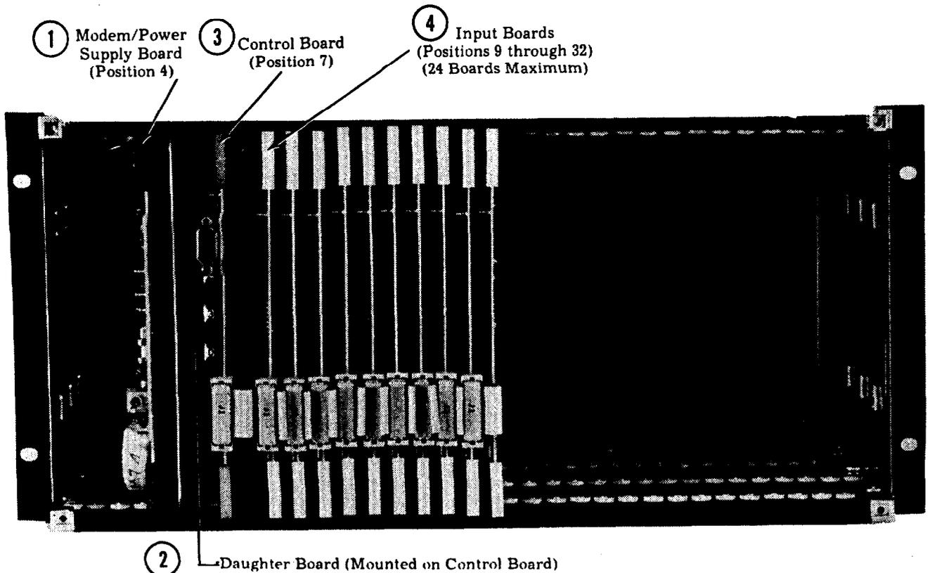
**Figure VI-1—Traffic Recorder Parts Location**
