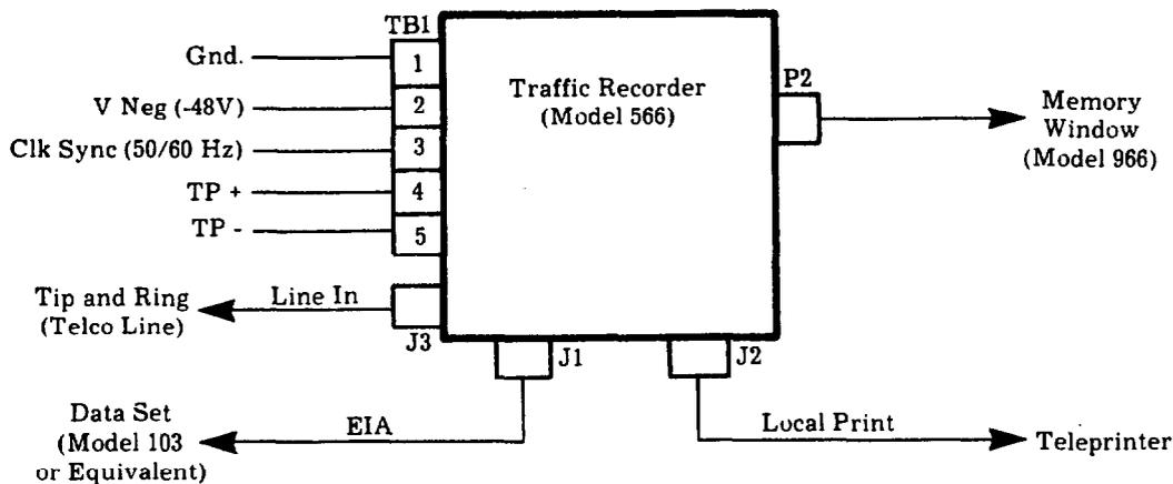
**Figure II-5—Equipment Interface Diagram**
