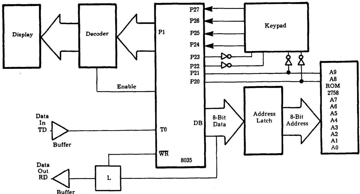
Figure IV-2—Model 966, Block Diagram
