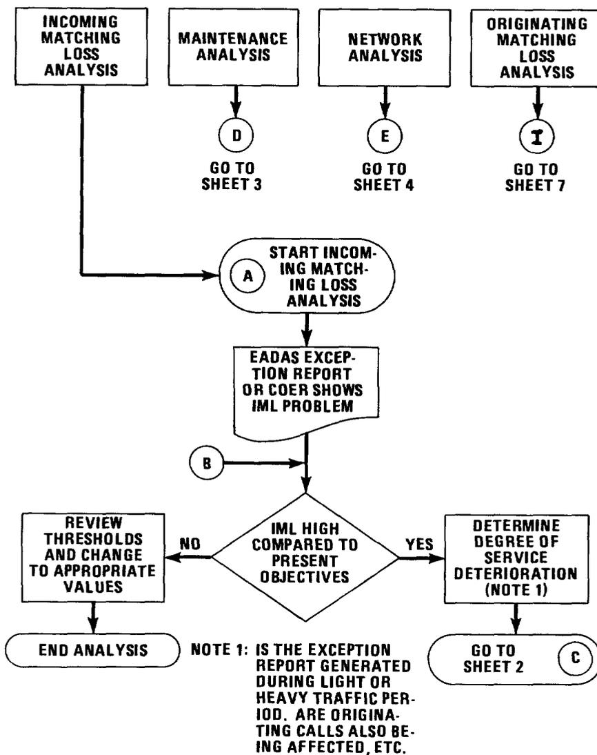
Figure 1 - Analysis Flowchart (Sheet 1 of 8) (10.01, 10.02)
