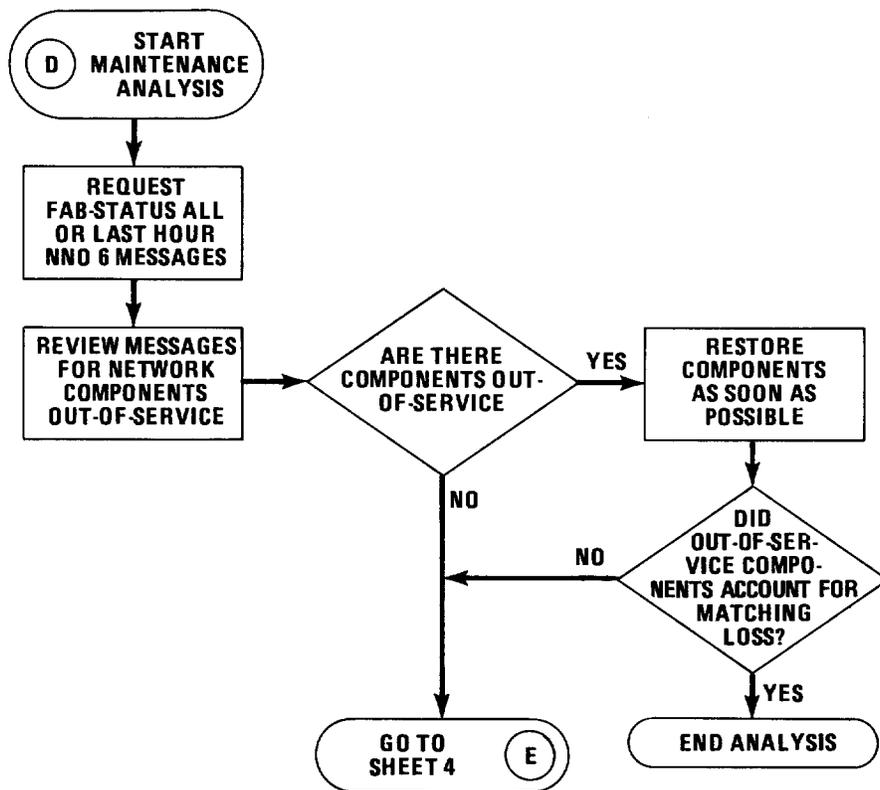
Figure 1 - Analysis Flowchart (Sheet 3 of 8) (10.01, 10.02, 10.06)
