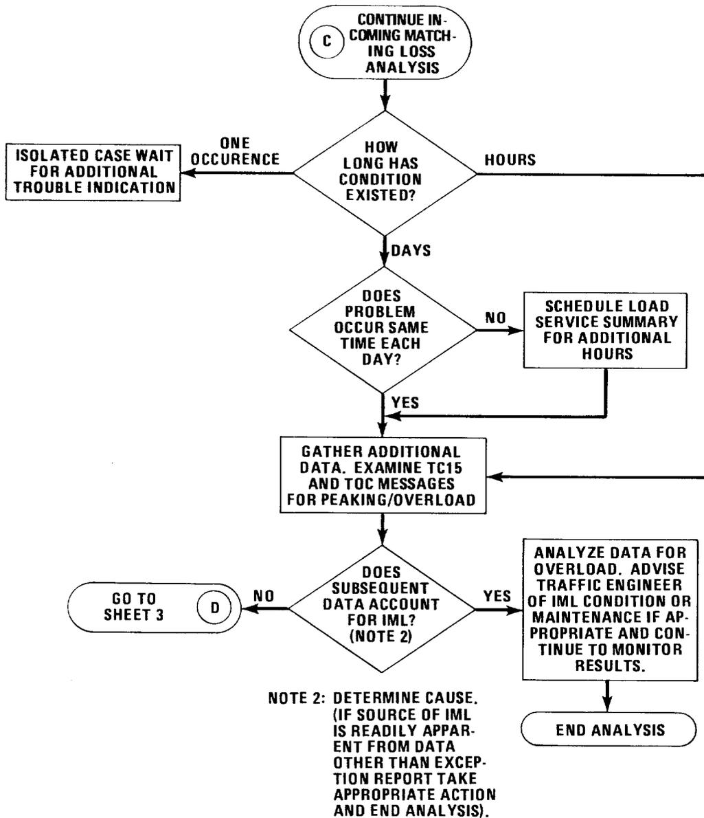
Figure 1 - Analysis Flowchart (Sheet 2 of 8) (10.01, 10.02)
