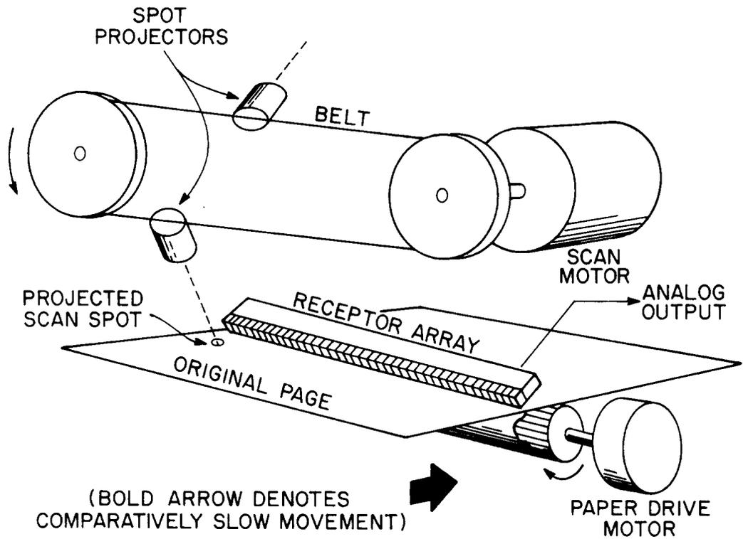
Fig 2—Through-Feed Method of Fax Scanning
