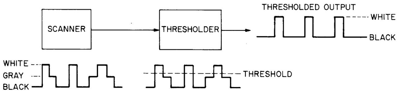
Fig 12—Effect of Thresholding on Scanner Output
