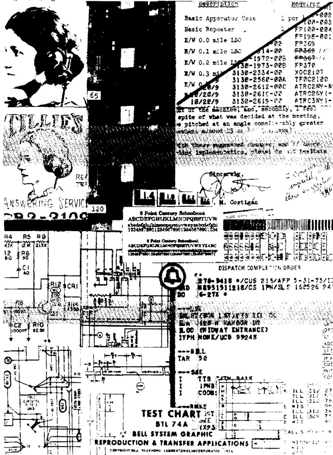
Fig 6—Visual Effect of High-Level Single-Frequency Interference (SFI) on a Group 2 Transmission
